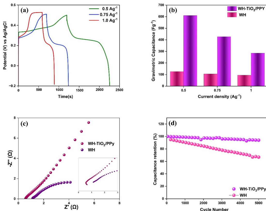
Fig. 7 (a) Galvanostatic charge–discharge curves of WH–TiO<sub>2</sub>/PPy at different current densities, (b) gravimetric capacitance of WH–TiO<sub>2</sub>/PPy and WH (c) Nyquist plots for WH–TiO<sub>2</sub>/PPy and WH, (d) cycling stability of WH–TiO<sub>2</sub>/PPy and WH.
