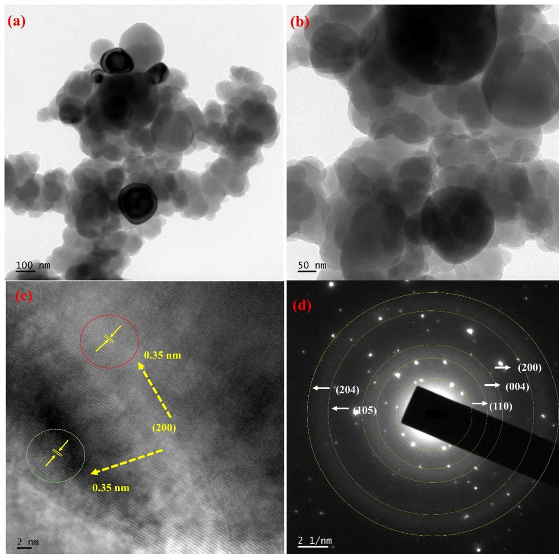
Fig. 4 TEM images showing the morphology of WH-TiO<sub>2</sub>/PPy at (a) 50, (b) 100 nm, (c) HRTEM, (d) SAED pattern.
