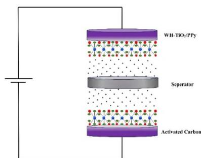
Fig. 8 The schematic assembly process for the asymmetric supercapacitor of WH-TiO<sub>2</sub>/PPy//AC.
