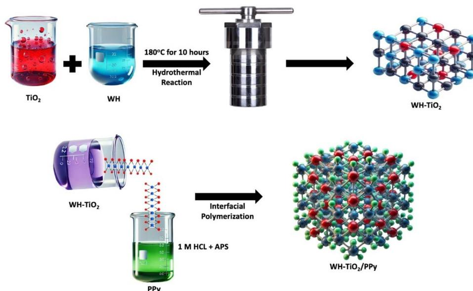
Fig. 1 Schematic illustration of the preparation process of WH–TiO<sub>2</sub>/PPy.
