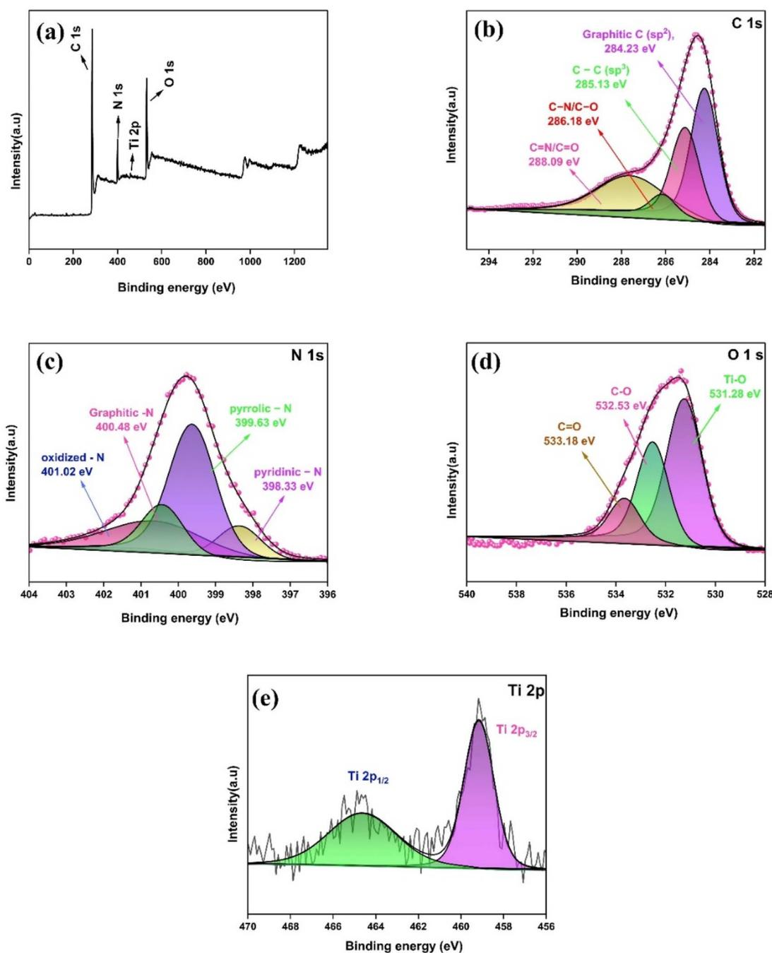
Fig. 5 XPS analysis of WH-TiO<sub>2</sub>/PPy composite: (a) survey spectrum, (b) C 1s, (c) N 1s, (d) O 1s, (e) Ti 2p.
