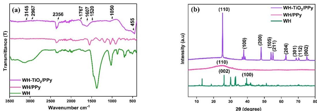
Fig. 2 (a) FTIR spectra of WH-TiO<sub>2</sub>/PPy, WH/PPy, and WH, and (b) XRD patterns of WH-TiO<sub>2</sub>/PPy, WH/PPy, and WH.
