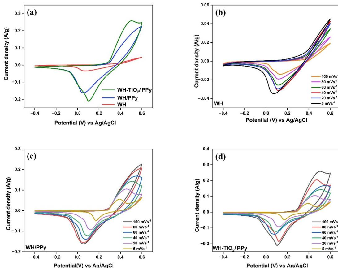
Fig. 6 (a) Cyclic voltammograms of WH, WH/PPy, and WH-TiO<sub>2</sub>/PPy electrodes in 3 M KOH electrolyte at a constant sweep rate of 100 mV s<sup>-1</sup>. Comparison of CV profiles for (b) WH, (c) WH/PPy, and (d) WH-TiO<sub>2</sub>/PPy at a scan rate (5–100 mV s<sup>-1</sup>).
