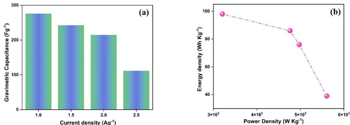
Fig. 10 (a) Gravimetric capacitance at different current densities calculated for the cell, (b) Ragone plot for WH-TiO<sub>2</sub>/PPy.
