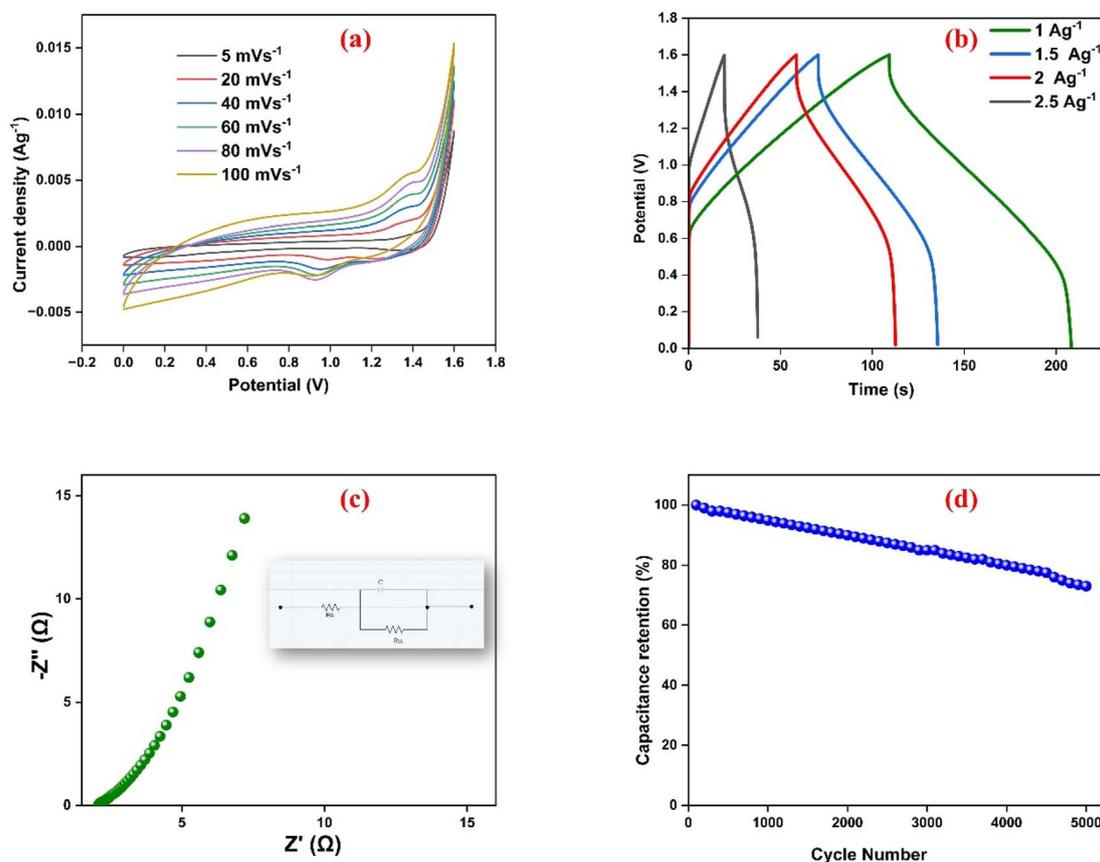
Fig. 9 Electrochemical performance of the WH-TiO<sub>2</sub>/PPy//AC asymmetric supercapacitor in 3 M KOH electrolyte. (a) Cyclic voltammograms at various scan rates, (b) galvanostatic charge-discharge curves recorded at different current densities, (c) Nyquist plot showcasing the impedance characteristics of the fabricated cell, and (d) cycling stability illustrating the capacitance retention over repeated charge-discharge cycles.
