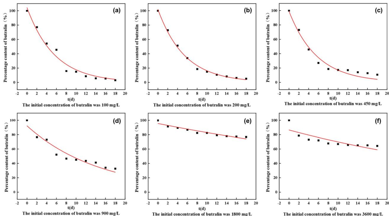
Fig. 4 First-order kinetic model for six different concentrations of butralin. The initial butralin concentrations of were  $100 \text{ mg L}^{-1}$  (a),  $200 \text{ mg L}^{-1}$  (b),  $450 \text{ mg L}^{-1}$  (c),  $900 \text{ mg L}^{-1}$  (d),  $1800 \text{ mg L}^{-1}$  (e),  $3600 \text{ mg L}^{-1}$  (f).
