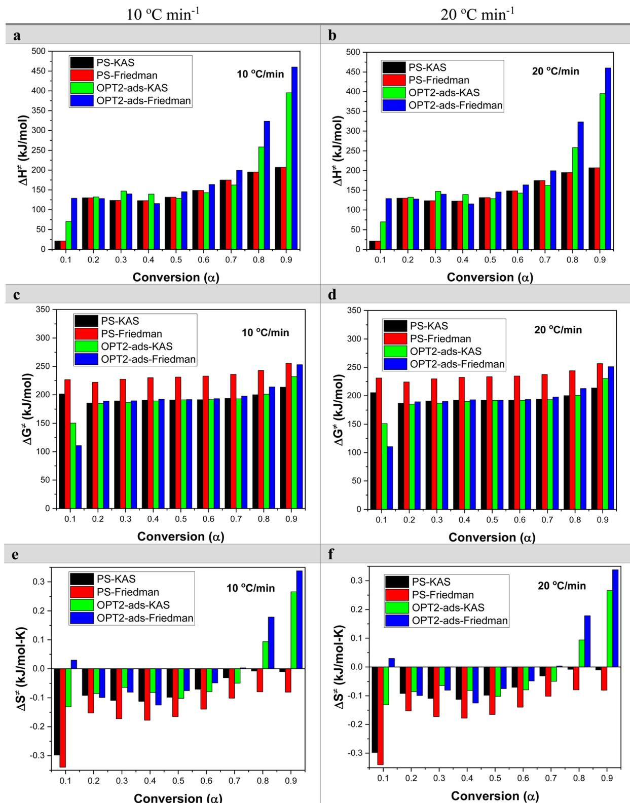
Fig. 8  $\Delta H^{\ddagger}$  vs. conversion for OPT2-ads and the parent sample (a) 10 °C min<sup>-1</sup> (b) 20 °C min<sup>-1</sup>;  $\Delta G^{\ddagger}$  vs. conversion for OPT2-ads and the parent sample (c) 10 °C min<sup>-1</sup> (d) 20 °C min<sup>-1</sup>;  $\Delta S^{\ddagger}$  vs. conversion for OPT2-ads and the parent sample (e) 10 °C min<sup>-1</sup> (f) 20 °C min<sup>-1</sup>
