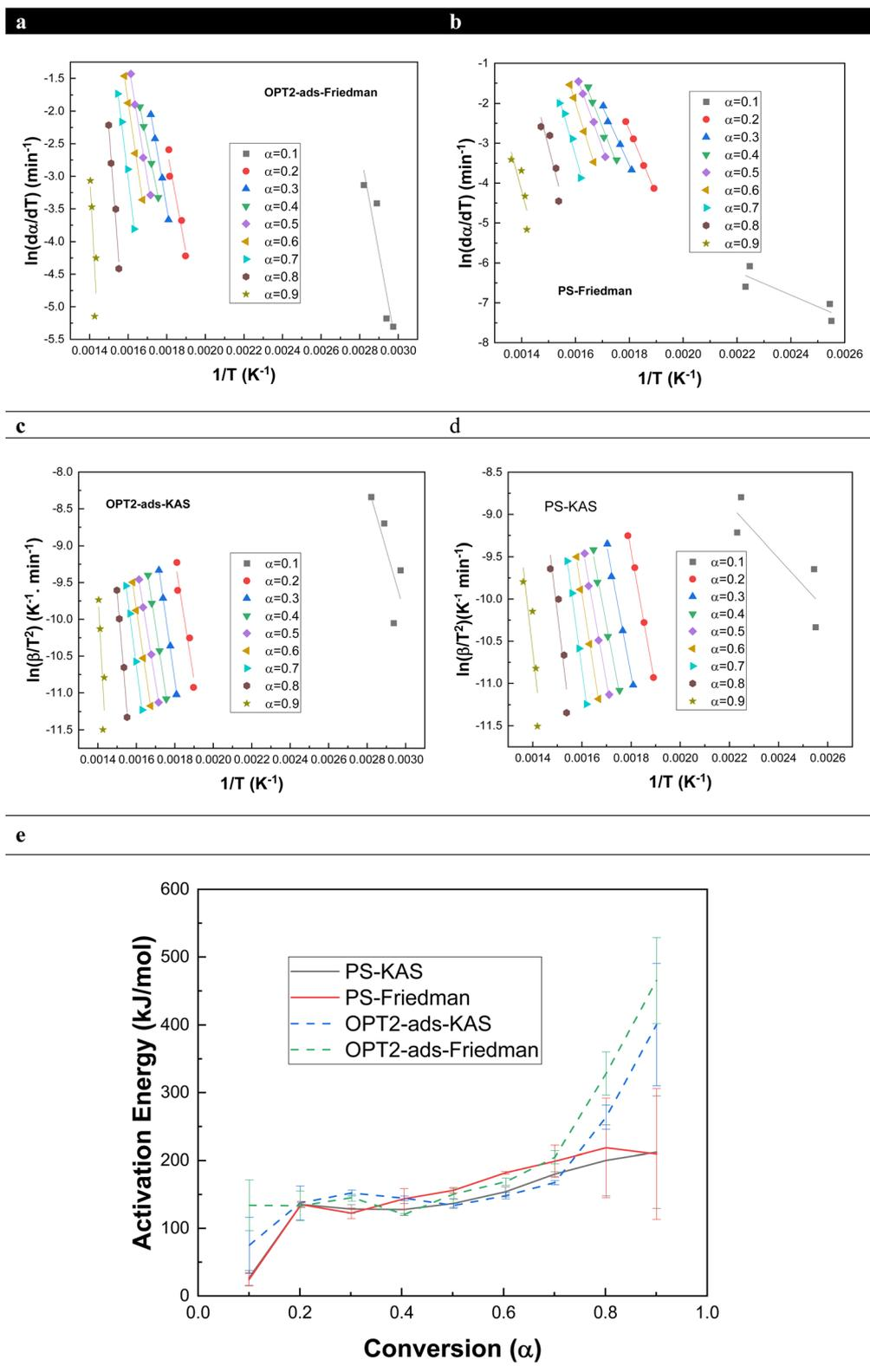
Fig. 7 Activation plots (a) Friedman plot for OPT2-ads (b) Friedman plot for the parent PF (c) KAS plot for OPT2-ads (d) KAS plot for the parent PF (e) variations in  $E$  vs. conversion for OPT2-ads and the parent PF samples.
