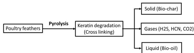
Scheme 1 Thermochemical (pyrolysis) reaction pathway of poultry feathers.
