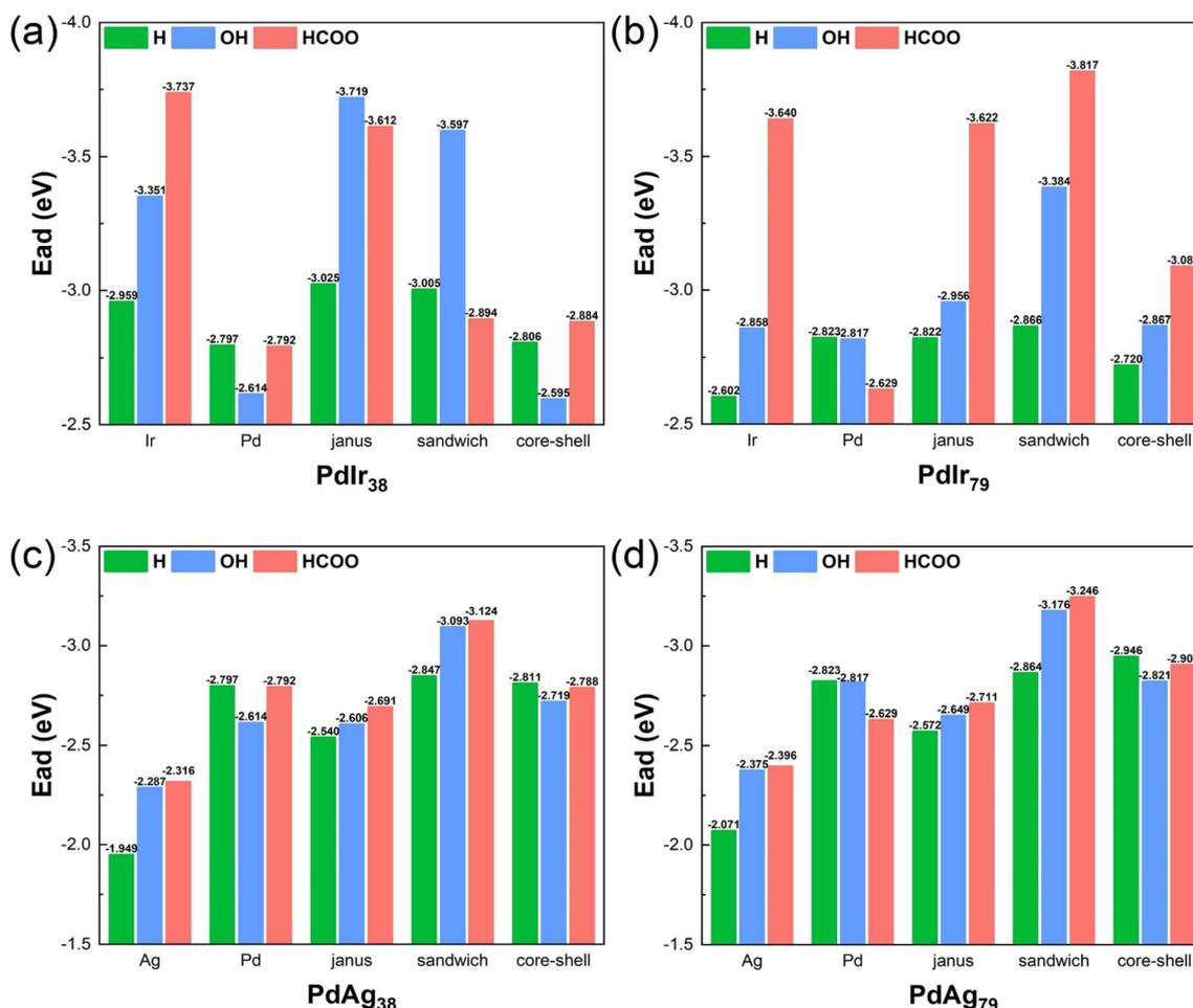
Fig. 1 The adsorption energy of H, OH, and HCOO on (a) PdIr<sub>38</sub>, (b) PdIr<sub>79</sub>, (c) PdAg<sub>38</sub> and (d) PdAg<sub>79</sub> nanoalloys.
