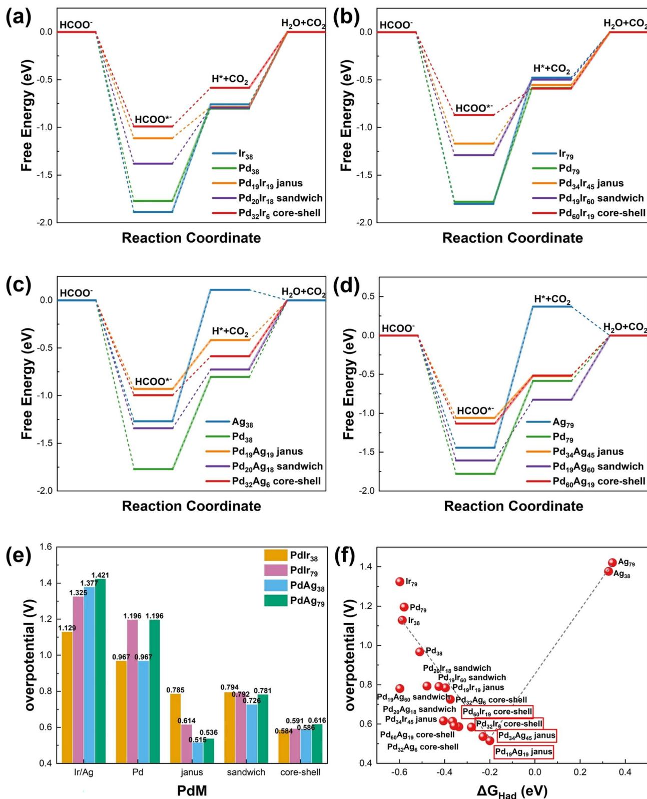
Fig. 3 Catalytic activity of the formate oxidation reaction (FOR) on PdM<sub>38</sub> and PdM<sub>79</sub> (M = Ir, Ag) nanoalloys. The free energy diagram of FOR on (a) PdIr<sub>38</sub>, (b) PdIr<sub>79</sub>, (c) PdAg<sub>38</sub> and (d) PdAg<sub>79</sub> nanoalloys. (e) The overpotential of FOR of the PdM<sub>38</sub> and PdM<sub>79</sub> (M = Ir, Ag) nanoalloys. (f) A plot of the overpotential of FOR versus the hydrogen adsorption free energy.
