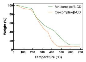
Fig. 4 TGA curves of Mn-complex/β-CD and Cu-complex/β-CD
