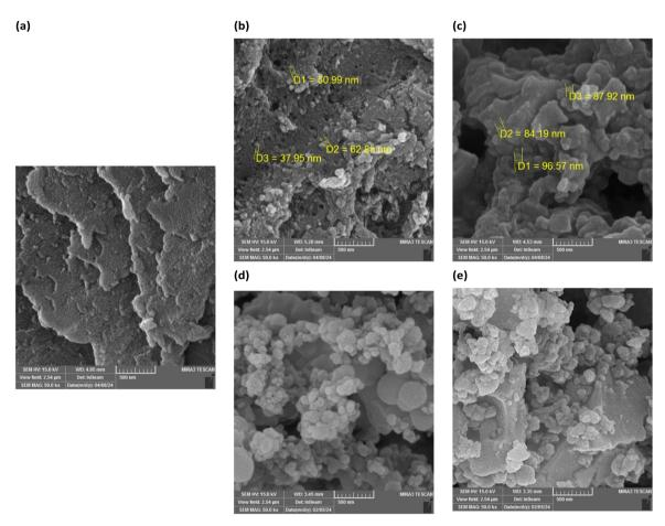
Fig. 3 SEM image of (a) ligand; (b) Mn-complex; (c) Mn-complex/β-CD; (d) Cu-complex and (e) Cu-complex/β-CD.
