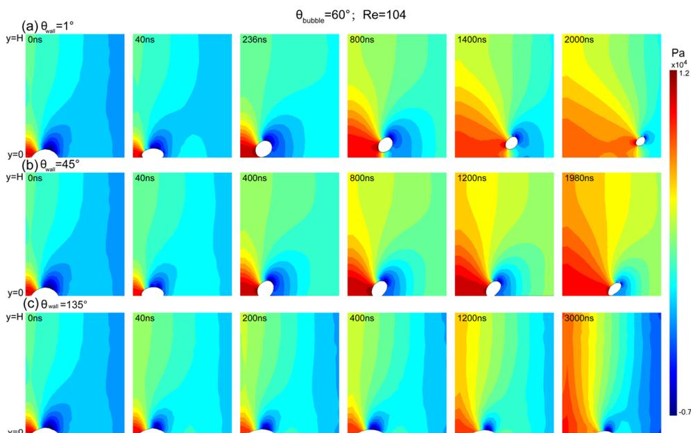
Fig. 9 Pressure contour plots showing the effects of microchannel wall wettability on bubble morphology. The value of  $\theta_{wall}$  was (a)  $1^\circ$ , (b)  $45^\circ$  and (c)  $135^\circ$ . The color bar indicates flow field pressure (Pa).
