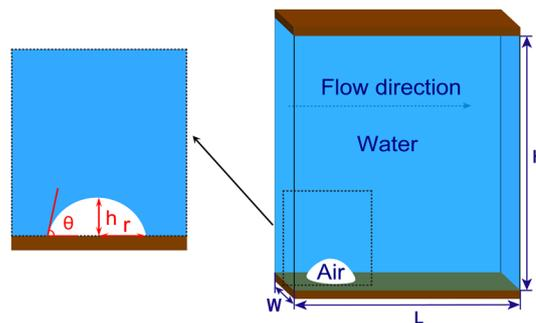
Fig. 1 Schematic diagram of microchannel model. A zoomed-in view showing the morphological parameters of a surface gas bubble. The bubble radius is  $2.4 \mu\text{m}$ , and the initial contact angle  $\theta$  is varied within the range of  $30^\circ$  to  $90^\circ$  in the simulation study.
