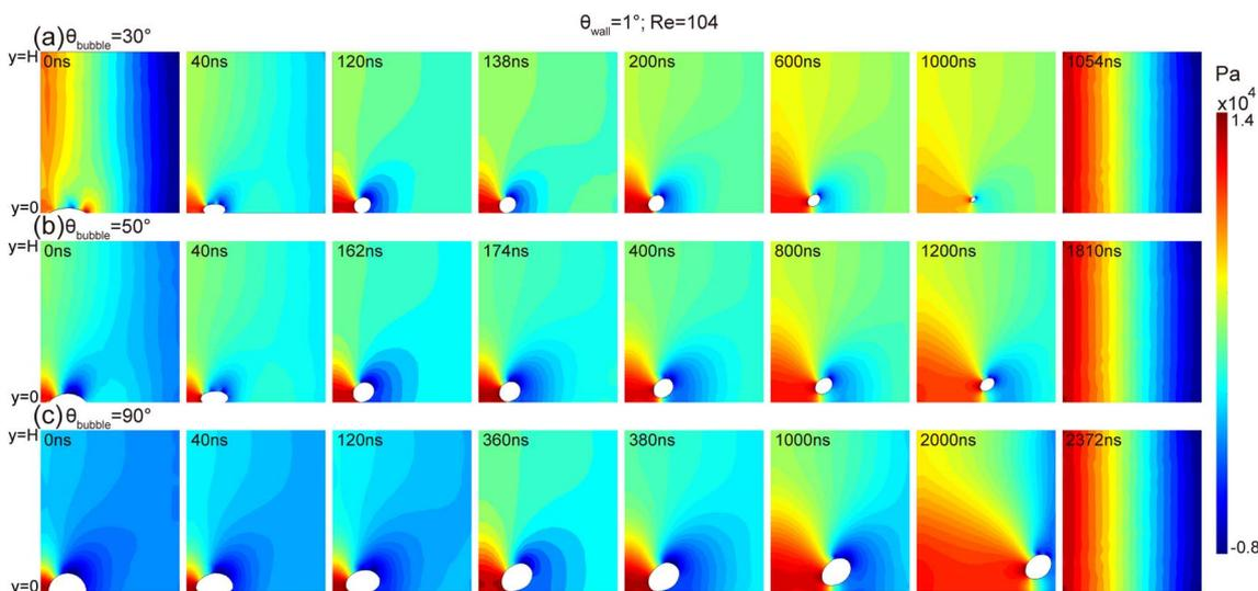
**Fig. 5** Pressure contour plots showing the effects of bubble initial contact angle on the bubble morphology in the course of surface-to-bulk conversion. The initial contact angle of surface gas bubble is (a) 30°, (b) 50° and (c) 90°. The color bar reflects the pressure change of the flow field (Pa).
