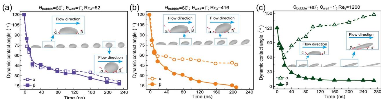
Fig. 11 Dynamic evolution of contact angles for surface bubbles at different Reynolds numbers (Re): (a) 52, (b) 416 and (c) 1200. The advancing angle and receding angles are denoted as  $\alpha$  and  $\beta$  respectively.
