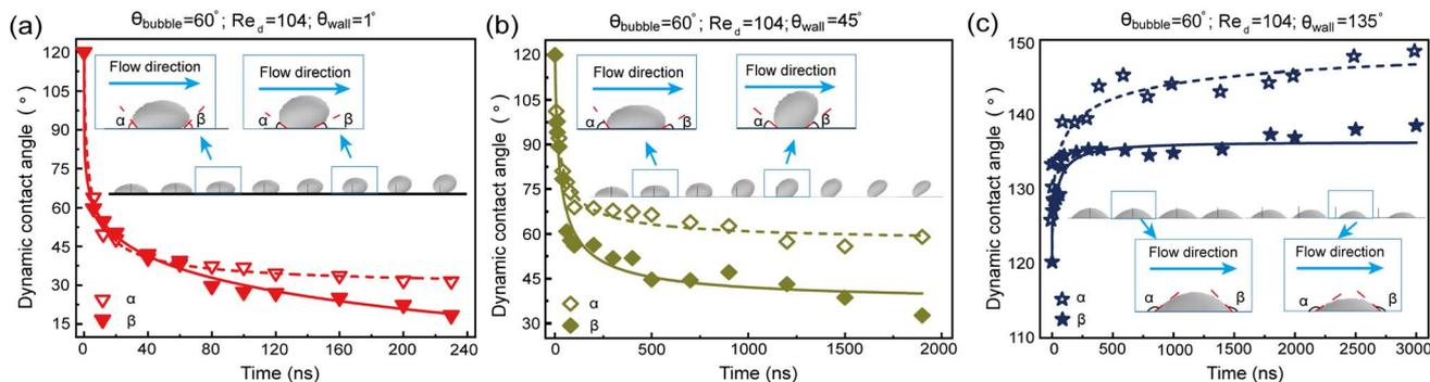
Fig. 12 Dynamic evolution of contact angles for surface bubbles at different wall wettabilities. The wetting angles  $\theta_{\text{wall}}$  are (a)  $1^\circ$ , (b)  $45^\circ$  and (c)  $135^\circ$ . The advancing and receding angle are labeled as  $\alpha$  and  $\beta$ , respectively.
