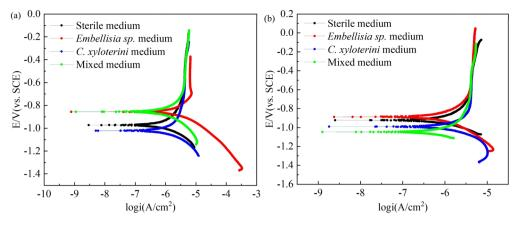
Fig. 7 Potentiodynamic polarization curves of 7B04 aluminum alloy after 12 d (a) and 28 d (b) of immersion in different systems.
