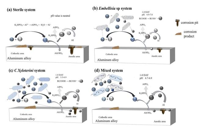
Fig. 12 Aluminium corrosion mechanism diagrams in sterile (a), Embellisia sp. (b), C. xyloterini (c), and mixed (d) systems
