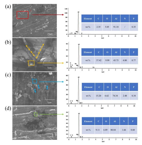
Fig. 9 Surface morphology and the corresponding EDS spectra of 7B04 aluminum alloy specimens after 28 d of immersion in sterile (a). Embellisia sp. (b), Candida xyloterini (c) and mixed (d) systems. Note: The double-headed arrow in the figure represents the length of the bacteria.
