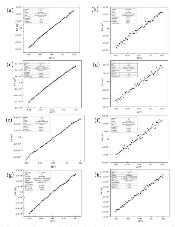
Fig. 8 Linear fitting results for the low overpotential interval of aluminum alloy polarization curves for different systems (a) Candida xyloterini-12d, (b) Candida xyloterini-28d, (c) Embellisia sp.-12d, (d) Embellisia sp.-24, (e) mixed-12d, (f) mixed-12d, (g) sterile-12d, (h) sterile-24d.
