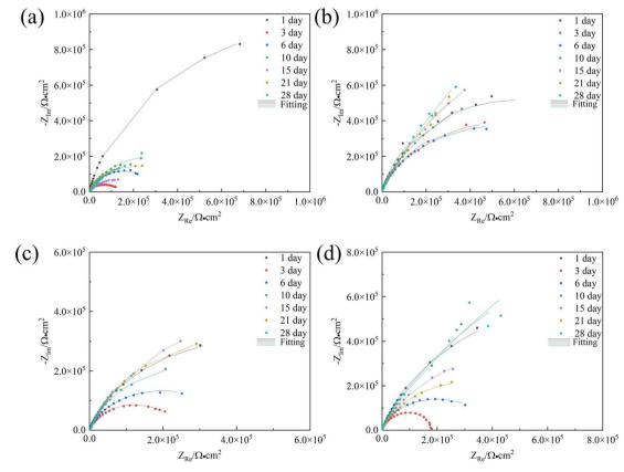
Fig. 3 Nyquist plots of 7B04 aluminum alloy after different immersion time in sterile (a), Embellisia sp. (b), C. xyloterini (c) and mixed (d) systems.
