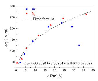
Fig. 10 Relationship between the  $\Delta$ THK and  $\Delta\sigma_{\rm f}$  of films treated with N<sub>2</sub> and Ar plasma.
