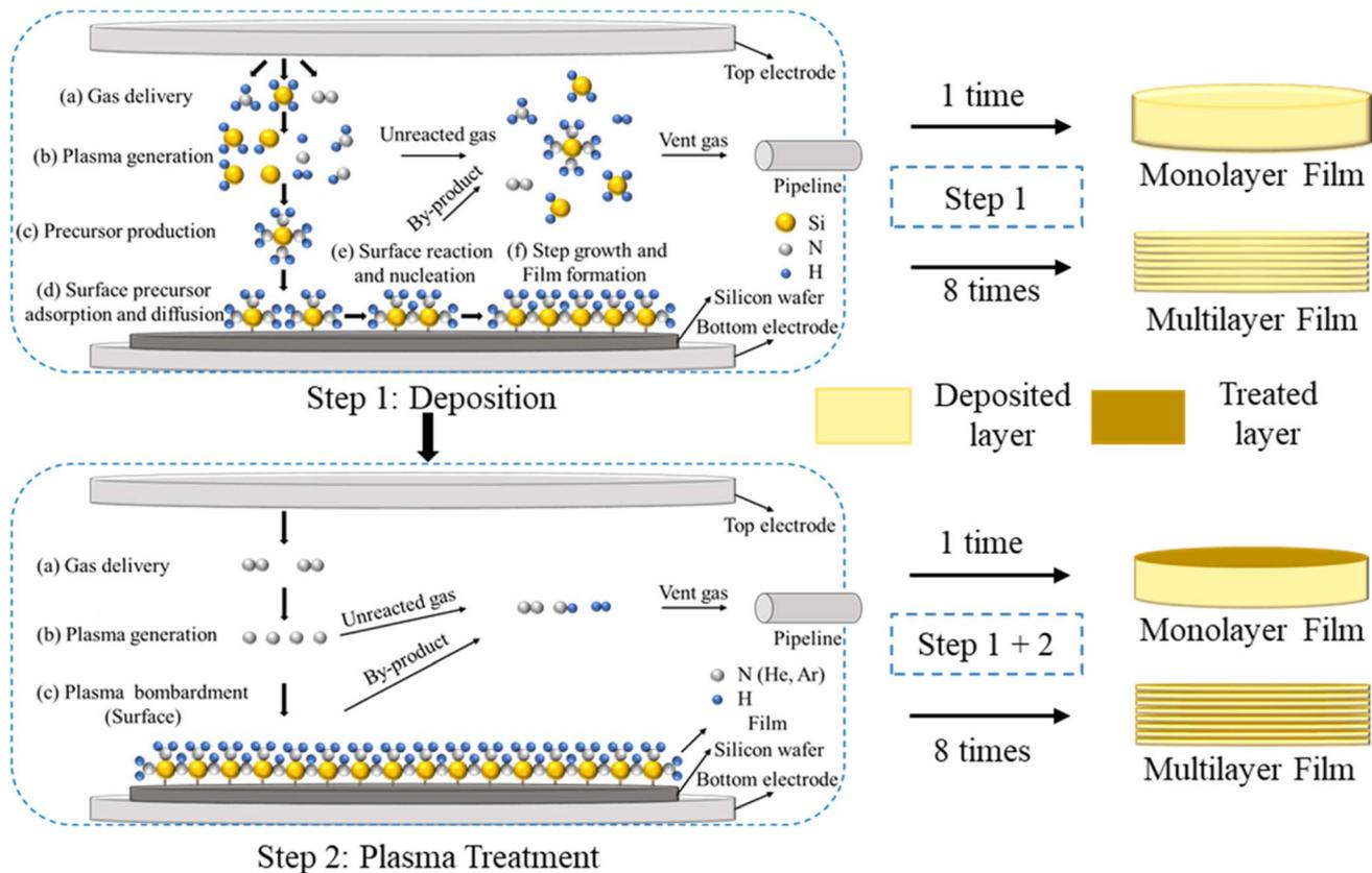
Fig. 1 Schematic of the deposition and treatment process of the Si<sub>x</sub>N<sub>y</sub>:H film.<sup>32</sup>
