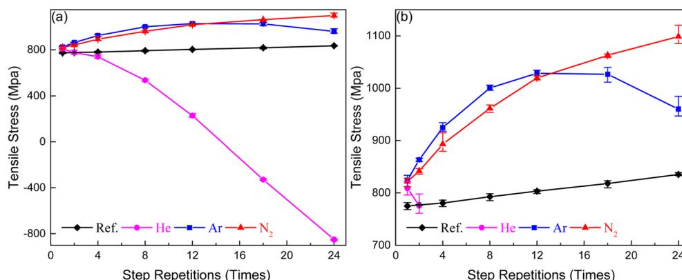
Fig. 2 The effect of He, Ar, and N<sub>2</sub> plasma bombardment on the stress of films (a) and an enlarged version of (a) and (b).
