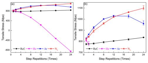
Fig. 2 The effect of He, Ar, and N<sub>2</sub> plasma bombardment on the stress of films (a) and an enlarged version of (a) and (b).
