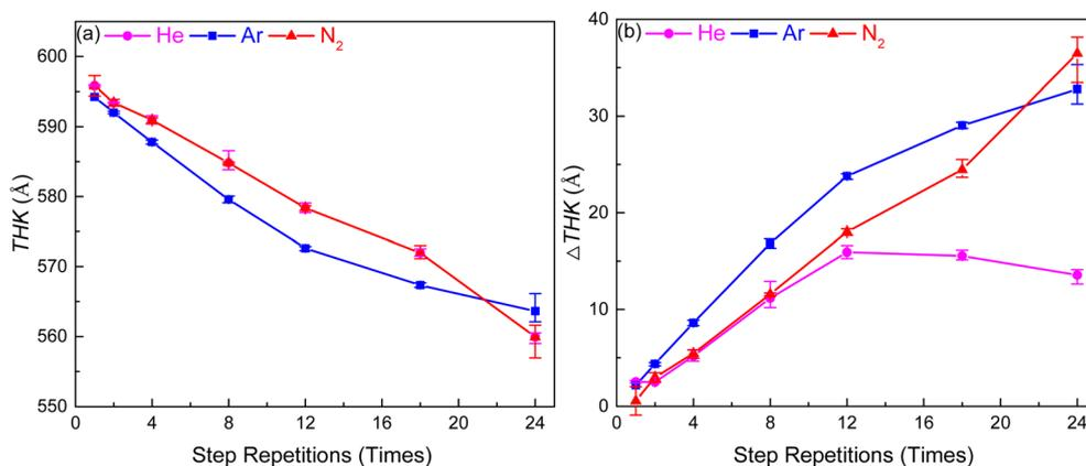
Fig. 6 The effect of He, Ar, and N<sub>2</sub> plasma bombardment on the (a) THK and (b)  $\Delta$ THK of films.
