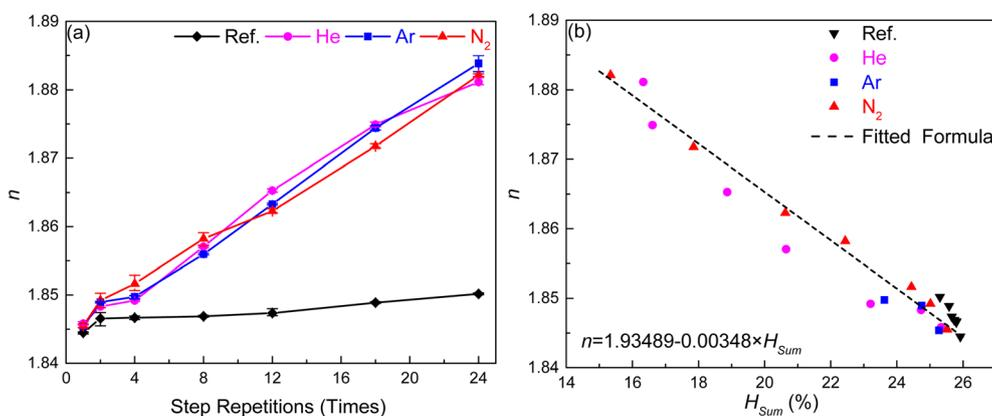
Fig. 7 (a) The effect of He, Ar, and N<sub>2</sub> plasma bombardment on the refractive index of films, and (b) the relationship between H<sub>sum</sub> and the refractive index.
