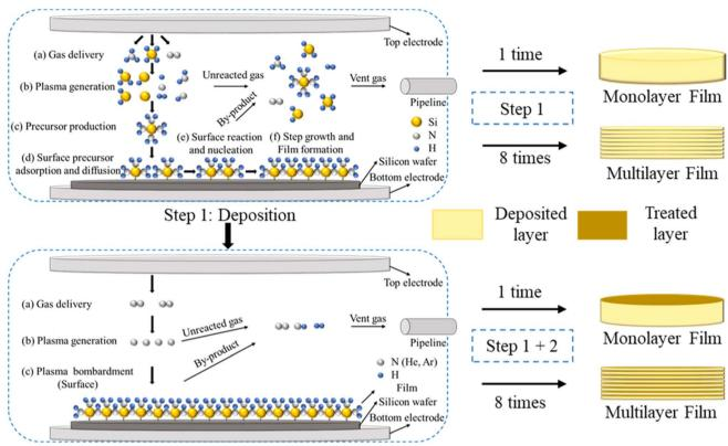
Fig. 1 Schematic of the deposition and treatment process of the  $SiN_x$ :H film.<sup>32</sup>
