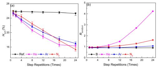
Fig. 3 The effect of He, Ar, and  $N_2$  plasma bombardment on the (a)  $H_{sum}$  and (b)  $R_{N-H/Si-H}$  of films.
