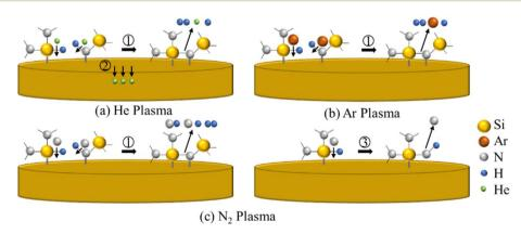
Fig. 4 Schematic of the plasma bombardment process on the film surface: (a) He plasma; (b) Ar plasma; (c) N<sub>2</sub> plasma.
