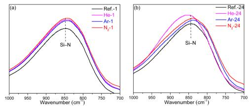
Fig. 11 FT-IR spectrum of (a) monolayer silicon nitride films and (b) multilayer silicon nitride films.
