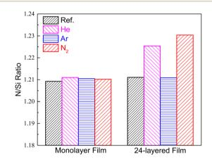
Fig. 5 The effect of He, Ar, and N<sub>2</sub> plasma bombardment on the N/Si atomic ratio of films.
