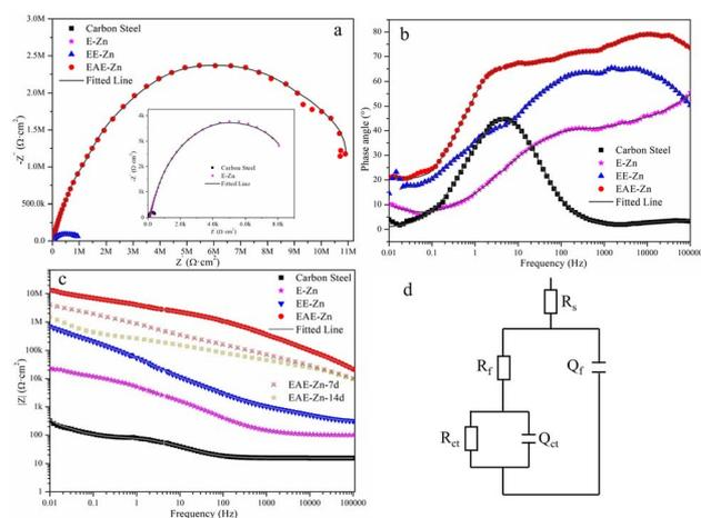
Fig. 8 Nyquist plots (a) Bode plots of negative phase angle vs. frequency (b), Bode plots of  $|Z|$  value vs. frequency (c) and the equivalent circuit model (d) of E-Zn, EE-Zn and EAE-Zn coatings in 3.5 wt% NaCl solution.
