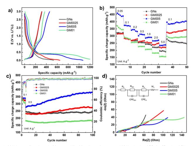
Fig. 6 (a) Voltage profile at 1st cycle, (b) rate capability, (c) cycling performance, and (d) Nyquist plot of EIS after 25 cycles of GNs and all GNs@MnO<sub>2</sub> samples.
