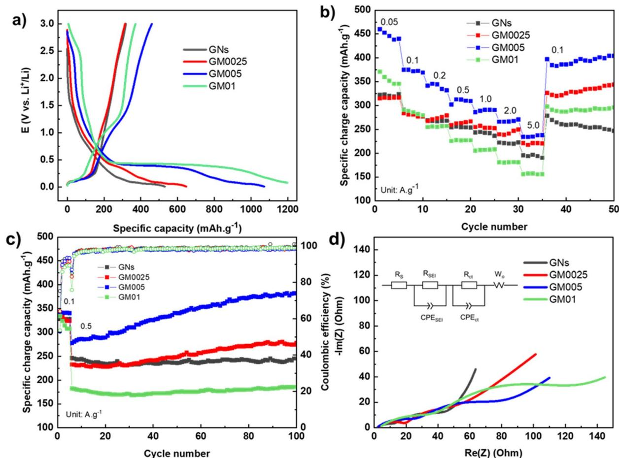
Fig. 6 (a) Voltage profile at 1st cycle, (b) rate capability, (c) cycling performance, and (d) Nyquist plot of EIS after 25 cycles of GNs and all GNs@MnO<sub>2</sub> samples.
