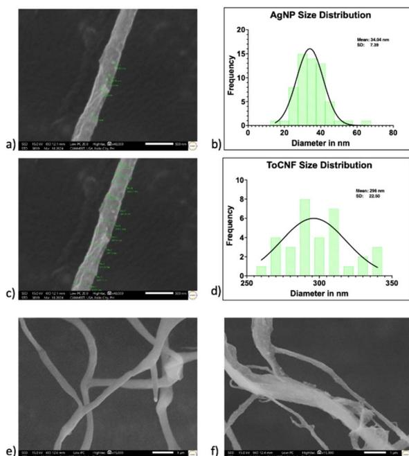
Fig. 10 SEM micrographs of (a) AgNPs at 40 000 $\times$  magnification (scale bar = 500 nm) and their corresponding size distribution (b); (c) ToCNFs at 40 000 $\times$  magnification (scale bar = 500 nm) with size distribution (d); and surface morphology comparison of (e) neat ToCNFs and (f) AgNP-loaded ToCNFs at 15 000 $\times$  magnification (scale bar = 1  $\mu\text{m}$ ). Particle size distributions are based on  $n = 60$  measurements.
