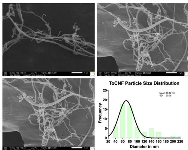
Fig. 6 SEM micrographs of ToCNFs taken at 15 000 $\times$  magnification with a scale bar of 1  $\mu$ m and the corresponding particle size distribution histogram illustrating the diameter range of the nanofibers,  $n = 60$ .
