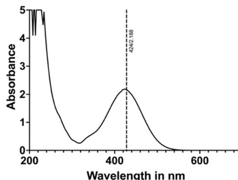
Fig. 9 UV-vis absorption spectrum of synthesized AgNP/ToCNF nanocomposite.
