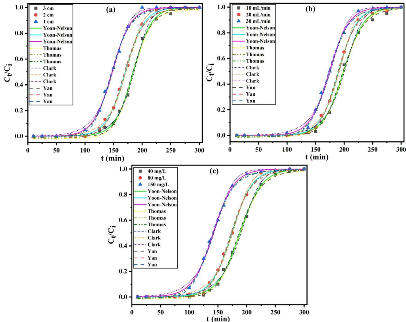
Fig. 7 Effect of bed height (a) at  $\mu = 30 \text{ mL min}^{-1}$  and  $C_i = 80 \text{ mg L}^{-1}$ , flow rate (b) at BH = 2 cm and  $C_i = 80 \text{ mg L}^{-1}$ , and initial  $Hg^{2+}$  concentration (c) at BH = 2 cm and  $\mu = 30 \text{ mL min}^{-1}$ , represented in the dots, for  $Hg^{2+}$  adsorption onto MFAC with the nonlinear fitting of Yoon-Nelson, Thomas, Clark, and Yan column models at 20 °C and pH 6.
