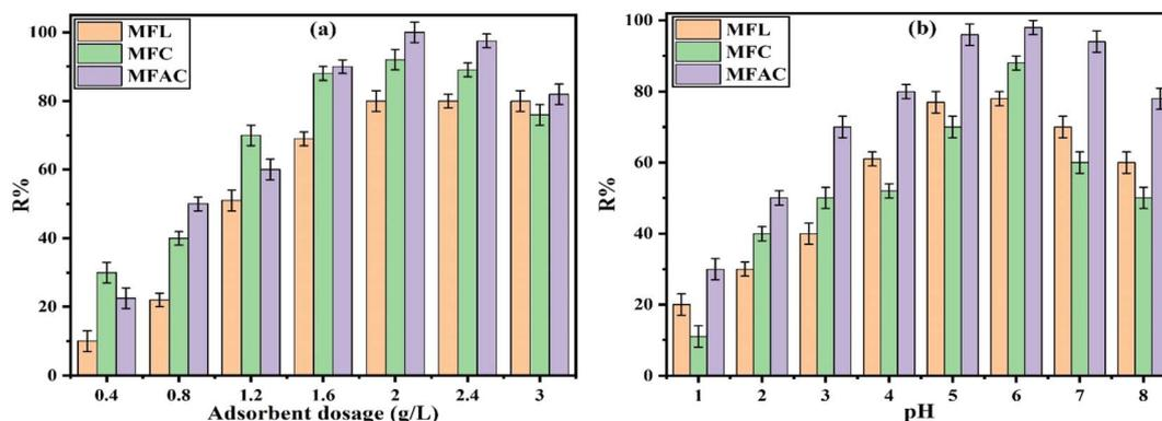
Fig. 3 Effect of adsorbent dose (a) and pH (b) for  $\text{Hg}^{2+}$  adsorption onto MFL, MFC, and MFAC at 20 °C,  $\text{Hg}^{2+}$  concentration of 900  $\text{mg L}^{-1}$ , and 60 min of shaking duration.
