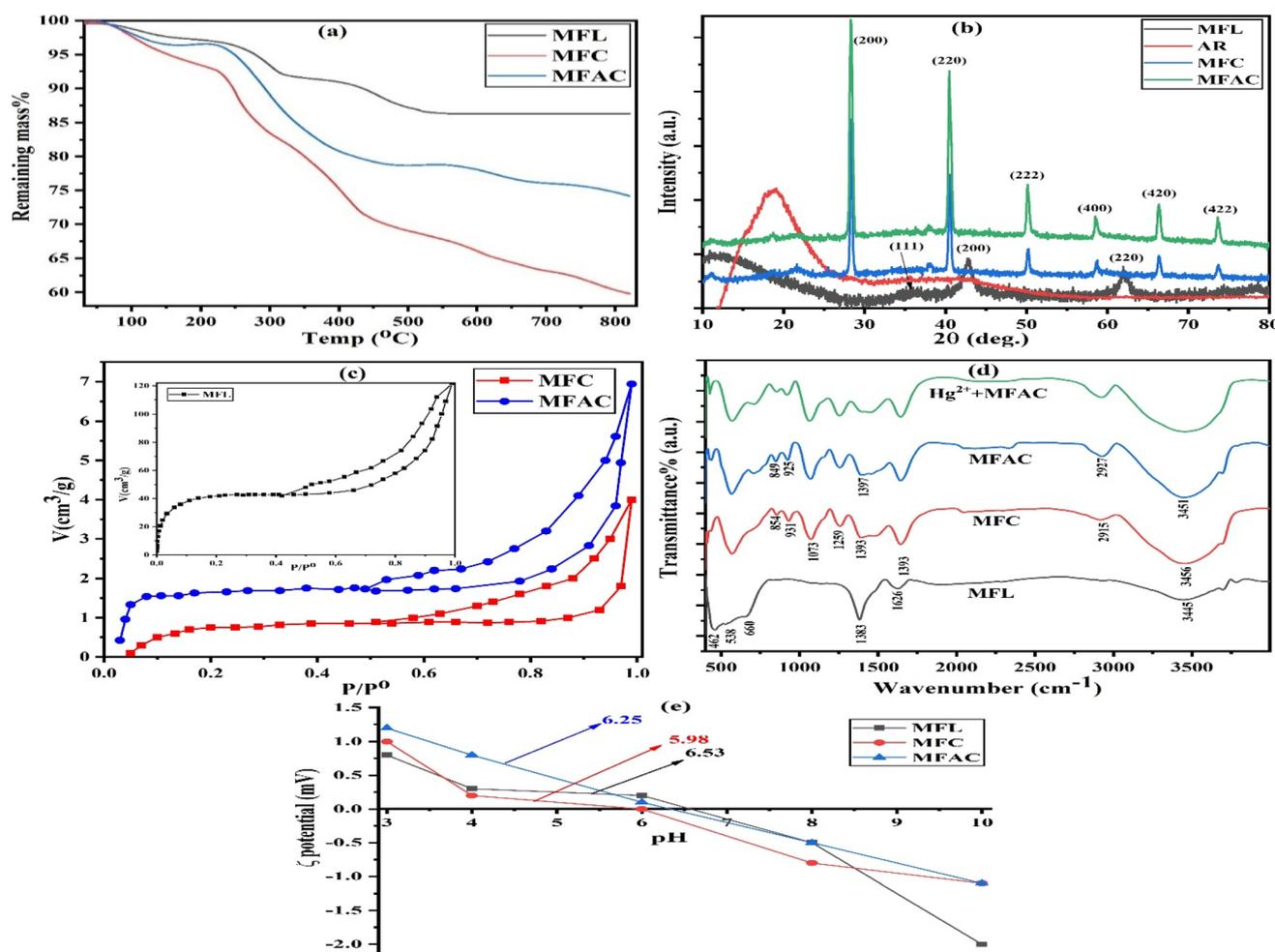
Fig. 1 TGA (a), XRD (b), N<sub>2</sub> adsorption (c), ATR-FTIR (d), zeta potential (e) curves for MFL, MFC, and MFAC, additionally, XRD for AR gum and ATR-FTIR curve of MFAC after Hg<sup>2+</sup> adsorption.
