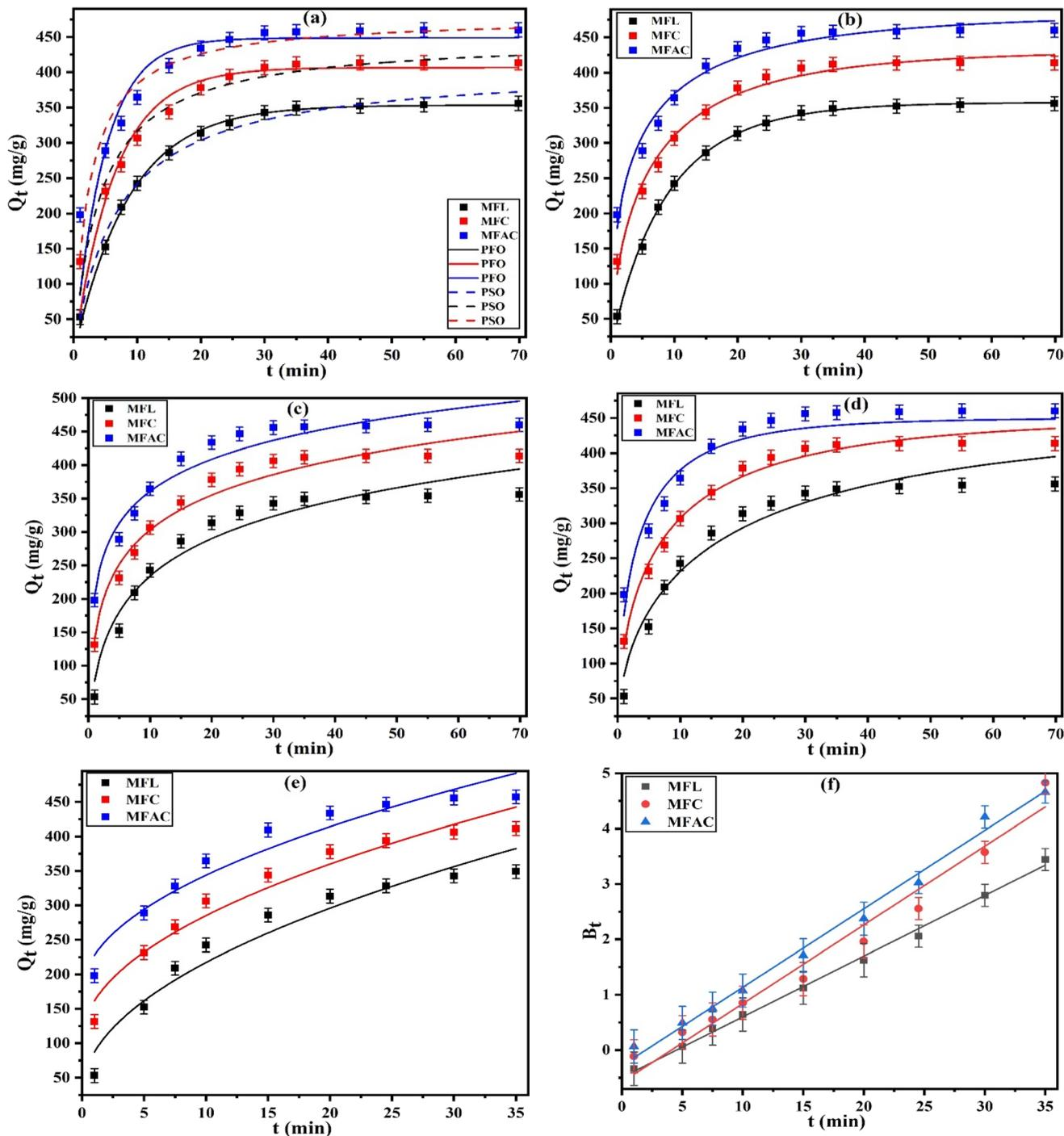
Fig. 4 The nonlinear plots of PFO and PSO (a), Avrami (b), Elovich (c), Bangham's pore diffusion (d), intra-particle diffusion (e), and linear Boyd (f) for the adsorption of  $\text{Hg}^{2+}$  onto MFL, MFC, and MFAC (at 20 °C, pH 6, initial  $\text{Hg}^{2+}$  concentration of 900  $\text{mg L}^{-1}$ , and adsorbent dosage of 2  $\text{g L}^{-1}$ ).
