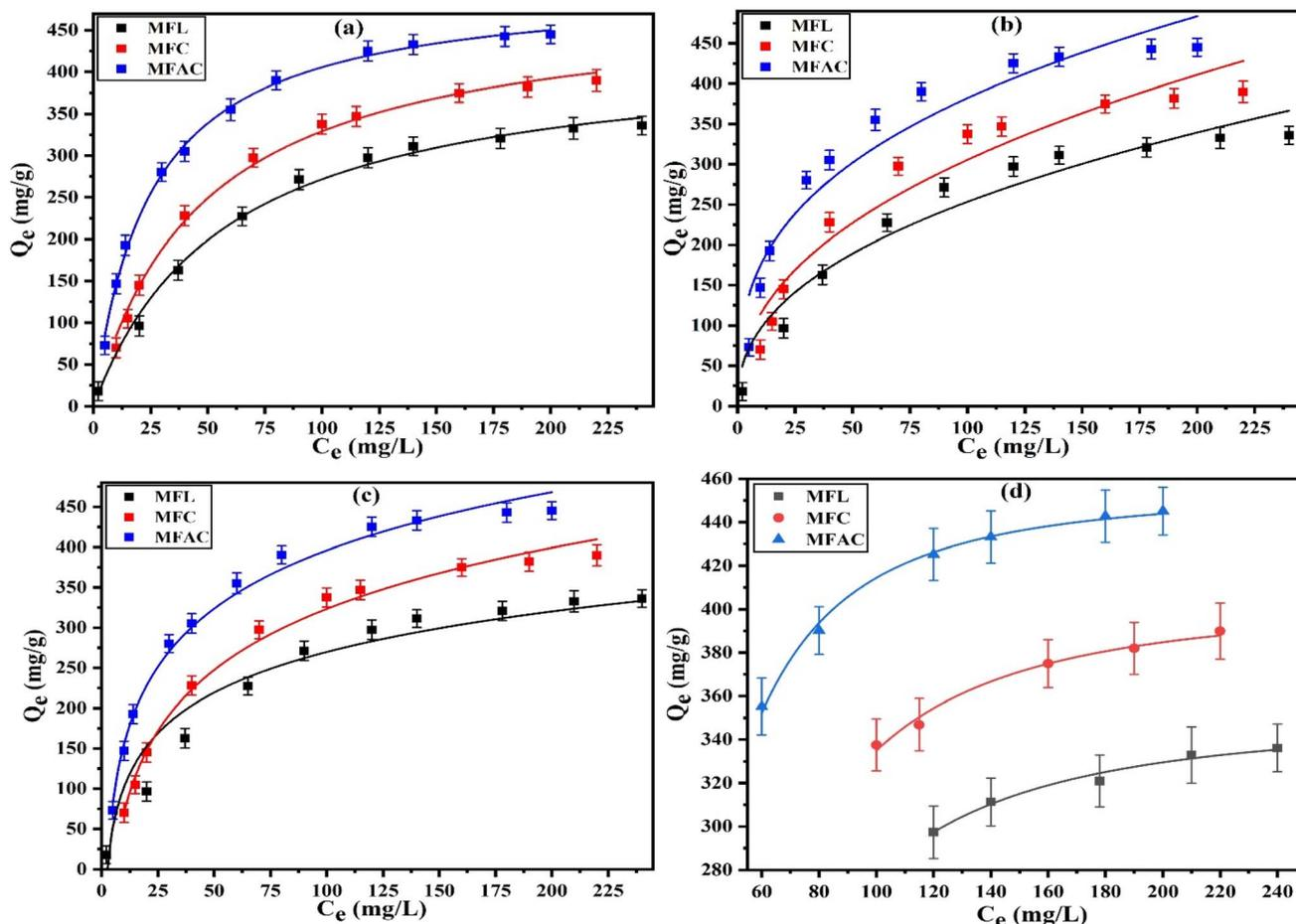
Fig. 5 The nonlinear plots of Langmuir (a), Freundlich (b), Temkin (c), and DR (d) for the adsorption of  $\text{Hg}^{2+}$  onto MFL, MFC, and MFAC at 20 °C, an adsorbent dosage of  $2 \text{ g L}^{-1}$ , and pH 6 for 30 min of shaking duration.
