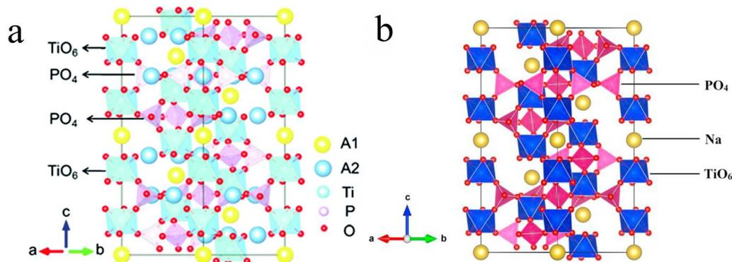
Fig. 2 Schematic illustration of the crystal structure. (a) Schematic illustration of the NASICON-type structure.<sup>39</sup> (b) Schematic illustration of the NTP structure.<sup>47</sup>
