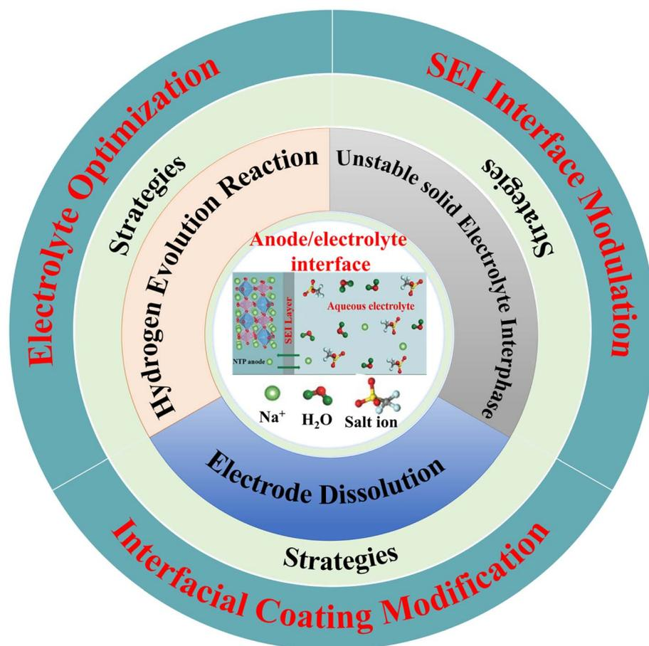
Fig. 3 Schematic illustration of the challenges and design strategy of NaTi<sub>2</sub>(PO<sub>4</sub>)<sub>3</sub> anode/electrolyte interface in ASIBs.
