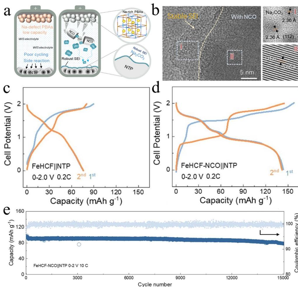
Fig. 9 Mechanism and performance evaluation of *in situ* SEI protection in ASIBs. (a) Schematic illustration of NCO additives for sodium supplementation with simultaneous construction of SEI interface in PBA-based full ASIBs.<sup>33</sup> (b) The cryo-TEM images of and elemental EDS mapping.<sup>33</sup> (c and d) The initial three charge–discharge profiles of FeHCF||NTP and FeHCF–NCO||NTP ASIBs at 0.2C. (e) The long-term cycling performance of FeHCF–NCO||NTP ANIBs at 10C.<sup>33</sup>
