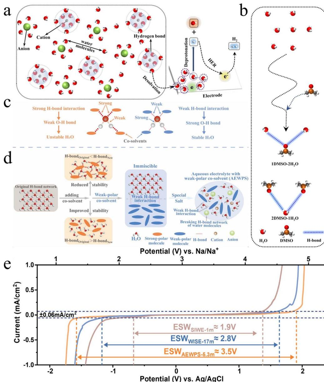
Fig. 5 Schematic illustration showing the design strategy and battery performance after optimizing the electrolyte. (a) Schematic diagram of the HER process.<sup>58</sup> (b) H-bond patterns between DMSO and water molecules.<sup>58</sup> (c and d) Schematic showing design strategies for aqueous electrolytes with a wide ESPW.<sup>60</sup> (e) Linear sweep voltammetry curves of different electrolytes at a scanning rate of 10 mV s<sup>-1</sup>.<sup>60</sup>
