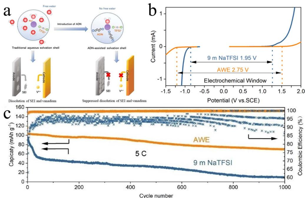
Fig. 8 Mechanism and performance of realizing *in situ* SEI protection in ASIBs. (a) Unique solvated structure lacking free water molecules.<sup>72</sup> (b) ESPW of AWE and 9 m NaTFSI obtained by linear sweep voltammetry on Pt foil electrodes.<sup>72</sup> (c) Long term cycling performance of Na<sub>3</sub>V<sub>2</sub>(PO<sub>4</sub>)<sub>3</sub>/NaTi<sub>2</sub>(PO<sub>4</sub>)<sub>3</sub> full cell at 5C.<sup>72</sup>
