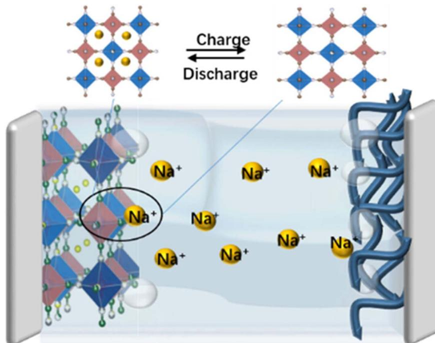
Fig. 1 Schematic diagram illustrating the working principle of an ASIB during charge/discharge cycles.<sup>28</sup>
