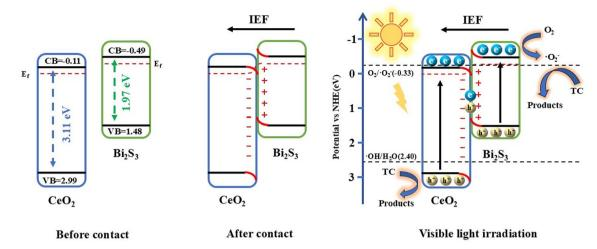
Fig. 10 Schematic energy band structure and photocatalytic mechanism of CeO<sub>2</sub>/Bi<sub>2</sub>S<sub>3</sub>-2 photocatalysts.
