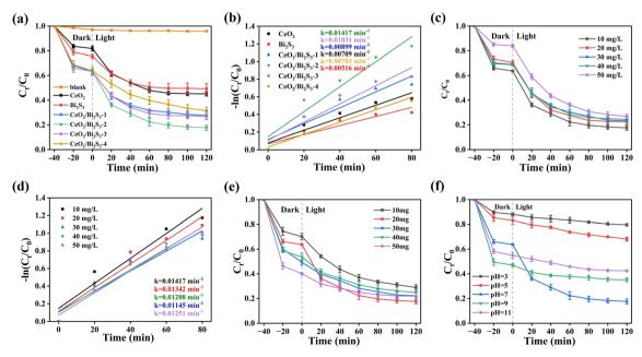
Fig. 4 (a) Photocatalytic degradation of TC by as-prepared photocatalysts under simulated solar illumination and (b) its kinetic fitting curves; 20 mg CeO<sub>2</sub>/Bi<sub>2</sub>S<sub>3</sub>-2 degradation of (c) different initial concentrations of TC solution and (d) its kinetic fitting curves; photocatalytic degradation of tetracycline solution by CeO<sub>2</sub>/Bi<sub>2</sub>S<sub>3</sub>-2 at (e) different catalyst dosage (f) different initial pHs.
