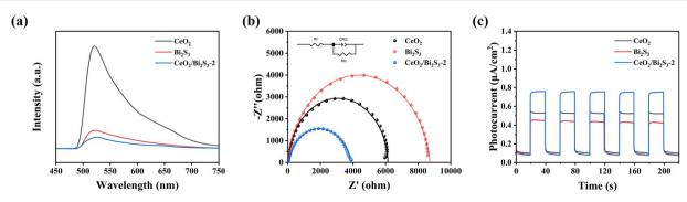
Fig. 5 (a) PL, (b) EIS Nyquist plot, and (c) transient photocurrent response of CeO<sub>2</sub>, Bi<sub>2</sub>S<sub>3</sub> and CeO<sub>2</sub>/Bi<sub>2</sub>S<sub>3</sub>-2.
