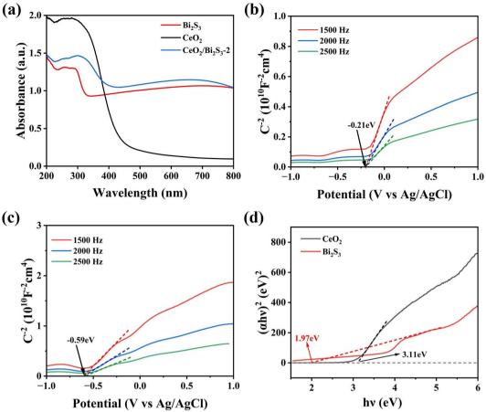
$\mbox{Fig. 8} \mbox{ (a) DRS spectra. Mott-Schottky spectra of (b) $CeO_2$ and (c) $Bi_2S_3$. (d) Tauc plot of $CeO_2$ and $Bi_2S_3$.}$
