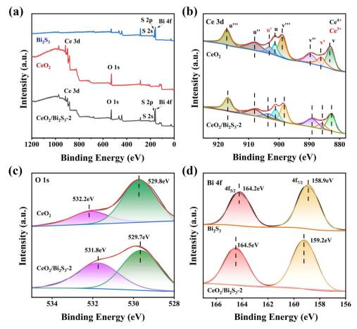
Fig. 3 XPS spectra of CeO<sub>2</sub>, Bi<sub>2</sub>S<sub>3</sub>, and CeO<sub>2</sub>/Bi<sub>2</sub>S<sub>3</sub>-2: (a) survey scan spectra; (b) Ce 3d; (c) O 1s; (d) Bi 4f.
