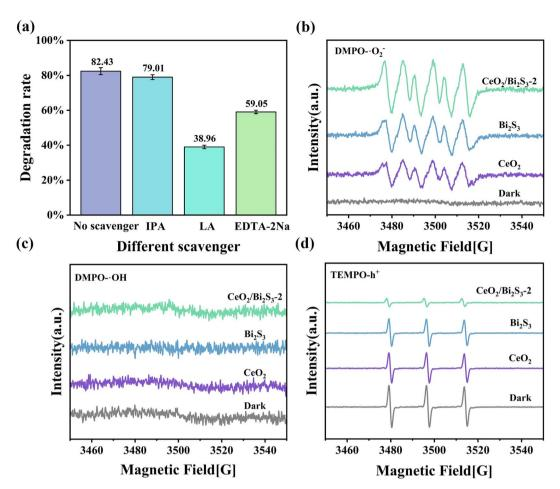
Fig. 7 (a) Effect of different scavengers on the photocatalytic degradation of TC by  $CeO_2/Bi_2S_3-2$ ; EPR signals of (b) DMPO $-\cdot O_2^-$ ; (c) TEMPO $-\cdot O_1^+$ ; (d) DMPO $-\cdot O_2^-$ .
