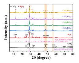
Fig. 1 Powder XRD diffraction patterns of CeO<sub>2</sub>, Bi<sub>2</sub>S<sub>3</sub>, and CeO<sub>2</sub>/Bi<sub>2</sub>S<sub>3</sub> samples.
