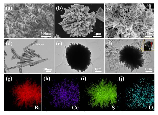
Fig. 2 SEM images of (a) CeO<sub>2</sub>; (b) Bi<sub>2</sub>S<sub>3</sub>; (c) CeO<sub>2</sub>/Bi<sub>2</sub>S<sub>3</sub>-2, TEM images of (d) CeO<sub>2</sub>; (e) Bi<sub>2</sub>S<sub>3</sub>; (f) CeO<sub>2</sub>/Bi<sub>2</sub>S<sub>3</sub>-2; EDS elemental distribution mapping of (g) Bi; (h) Ce; (i) S; (j) O in  $CeO_2/Bi_2S_3-2$ .
