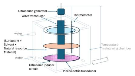
Fig. 6 Representation of ultrasonic extraction equipment.
