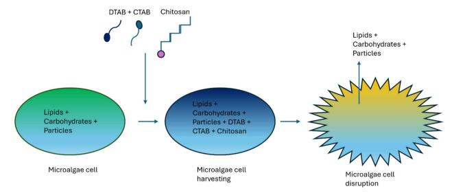
Fig. 3 Representation of the dual flocculation technique.
