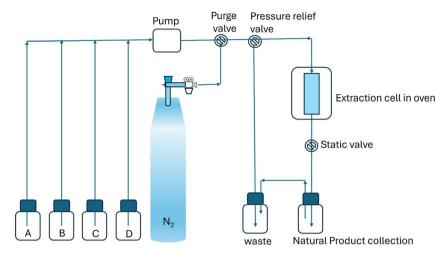
Fig. 4 Representation of pressurized liquid extraction (PLE) technique.
