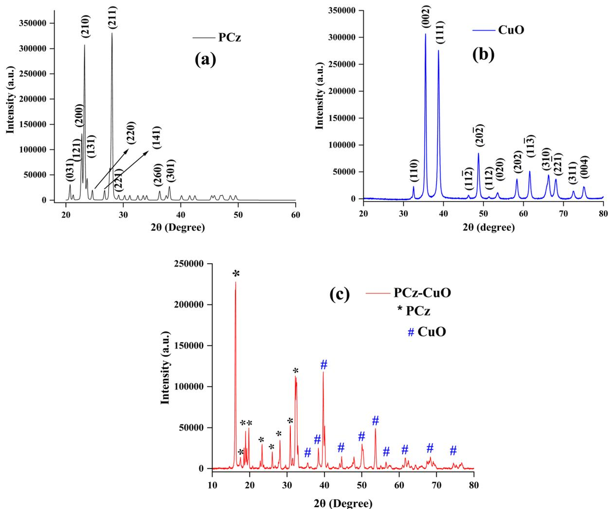
Fig. 2 P-XRD profile of (a) PCz, (b) CuO, and (c) PCz–CuO nanocomposite.
