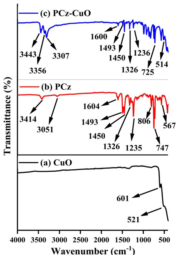
Fig. 1 FT-IR spectra of (a) CuO, (b) PCz, and (c) PCz-CuO nanocomposite.
