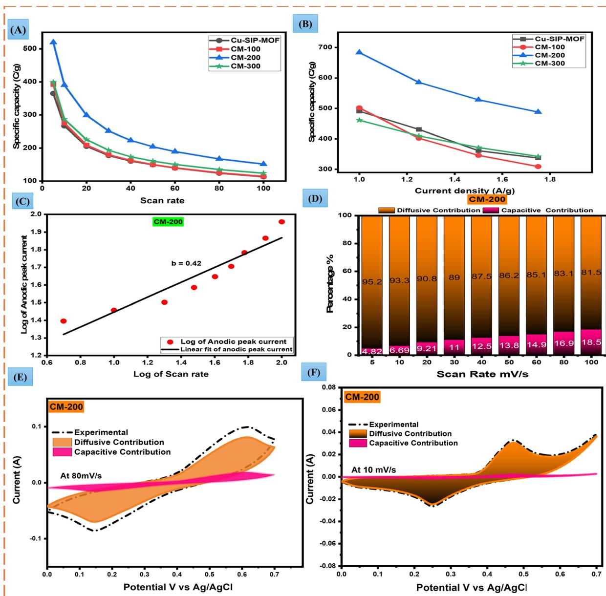
Fig. 5 (A) Specific capacities through CV at different scan rates. (B) Specific capacities calculated *via* GCD at various current densities. (C) Graph for  $b$ -value of CM-200. (D) Bar chart for capacitive and diffusive contributions. (E) Diffusive and capacitive contribution of CM-200 at 80 mV s<sup>-1</sup>. (F) Diffusive and capacitive contribution of CM-200 at 10 mV s<sup>-1</sup>.
