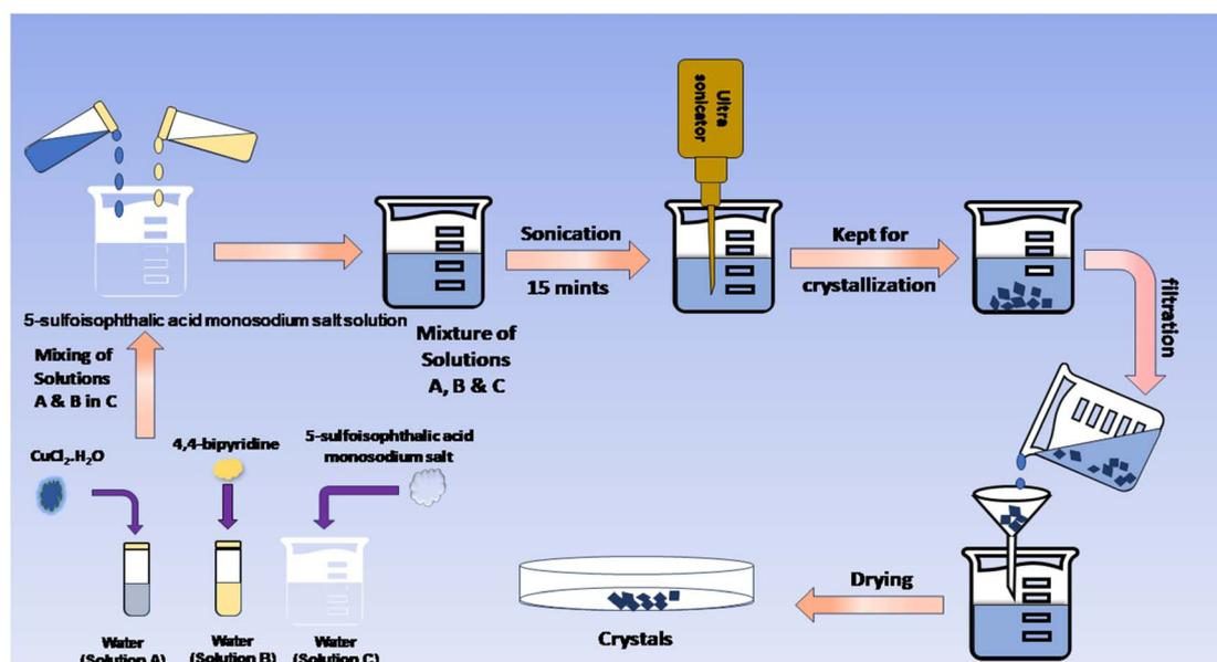
Fig. 1 Scheme for the synthesis of Cu-SIP-MOF.
