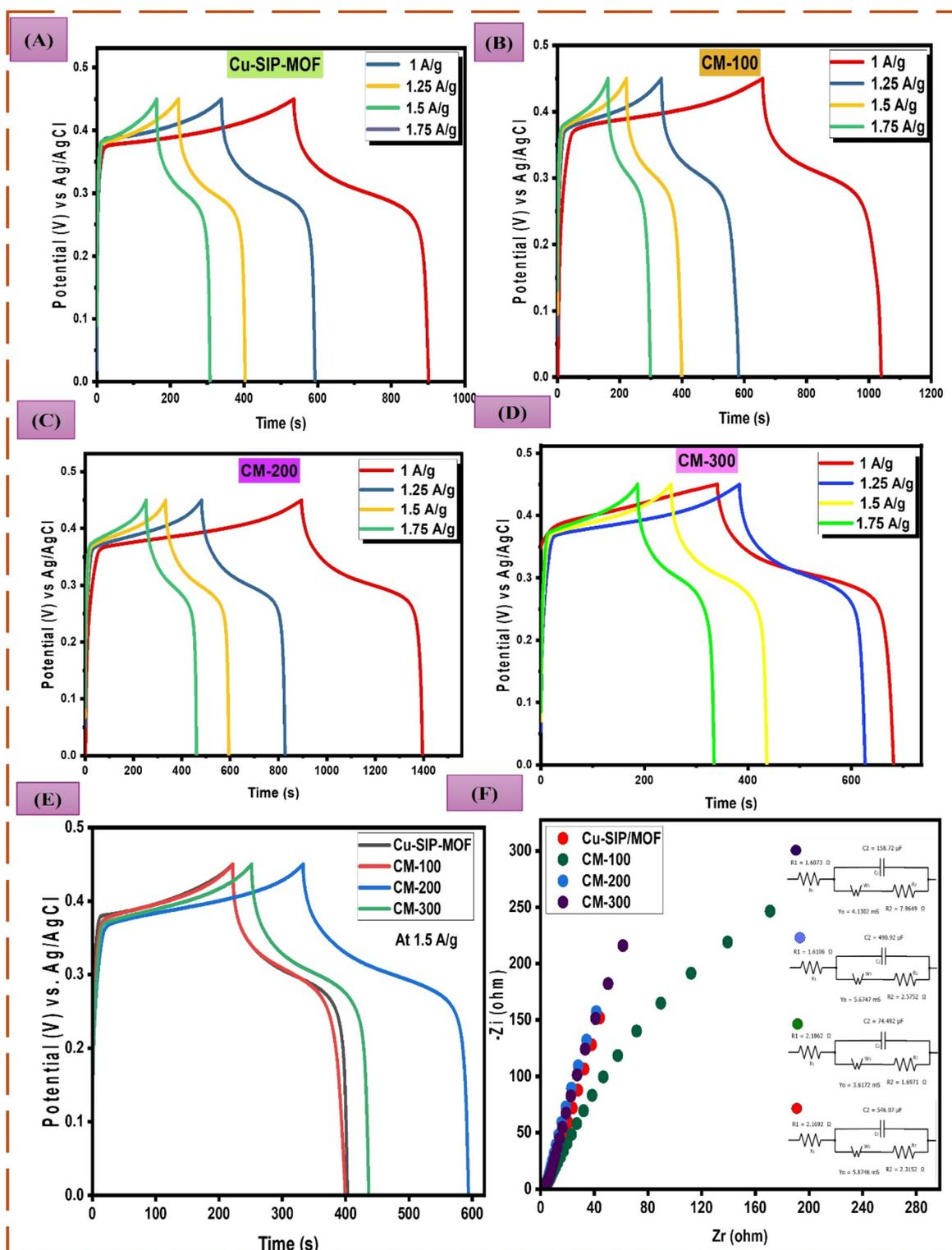
Fig. 6 (A) Galvanostatic charging–discharging at different scan rates for Cu-SIP-MOF, (B) CM-100, (C) CM-200 and (D) CM-300. (E) Comparison of GCD profiles of 1.5 A g<sup>-1</sup>. (F), EIS spectra of Cu-SIP-MOF, CM-100, CM-200 and CM-300 electrodes in three-electrode systems.
