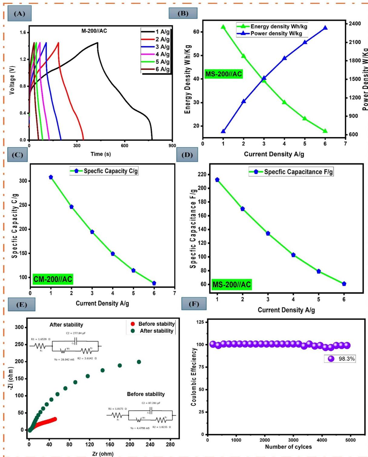
Fig. 8 (A) GCD profile at various current densities for the hybrid device. (B) Graph of energy and power density at various current densities. (C) Specific capacity for the CM-200//AC hybrid system at different current densities. (D) Specific capacitance for the CM-200//AC hybrid system at different current densities. (E) EIS spectra of CM-200//AC. (F) Plot representing coulombic efficiency after 5000 GCD cycles for the hybrid device.
