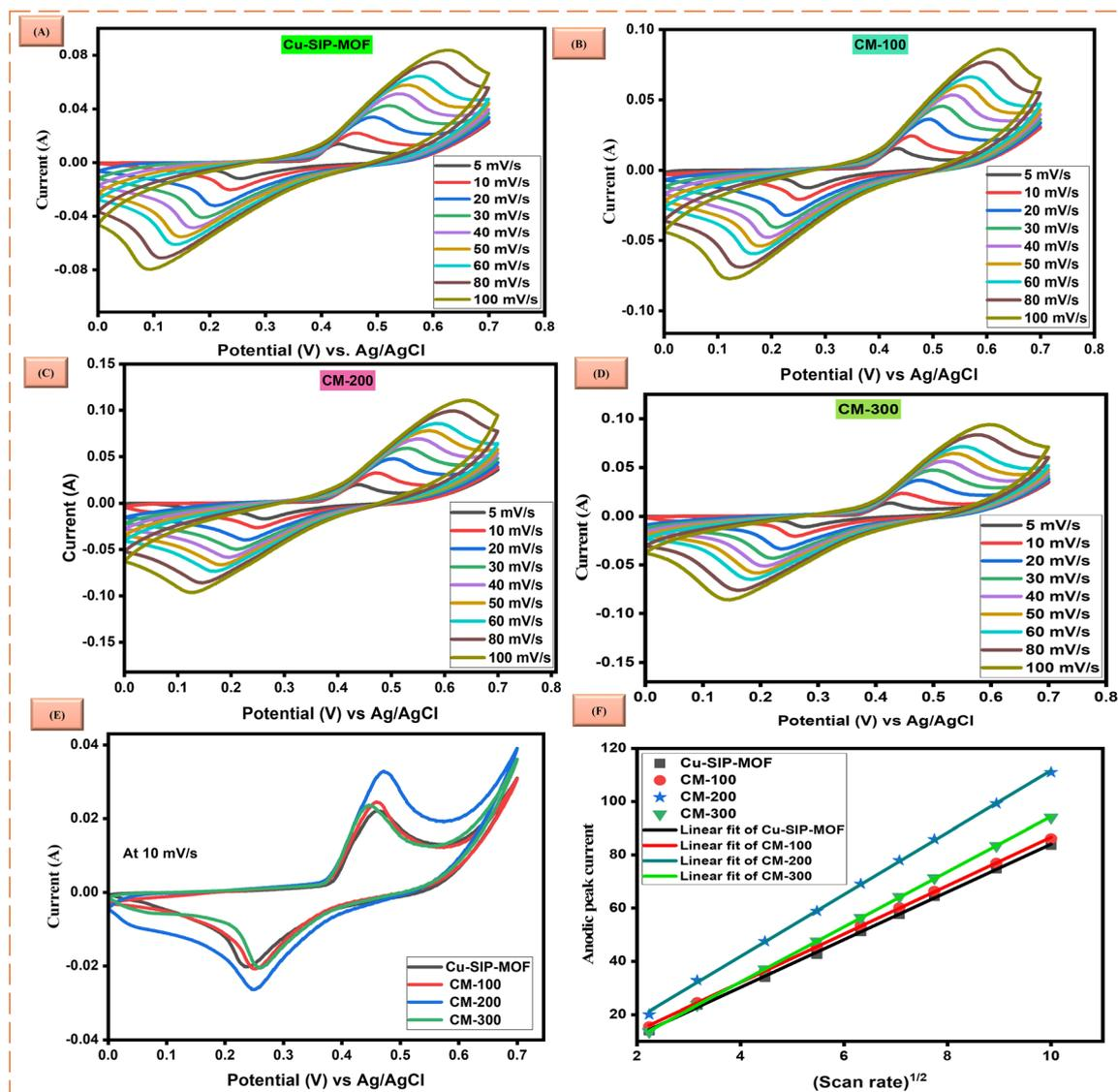
Fig. 4 (A) CV profiles of Cu-SIP-MOF, (B) CM-100, (C) CM-200 and (D) CM-300. (E) Graph of CV comparison for Cu-SIP-MOF, CM-100, CM-200 and CM-300 at 10  $\text{mV s}^{-1}$ . (F) Plot between the square root of the scan rate and the peak current for Cu-SIP-MOF, CM-100, CM-200 and CM-300.
