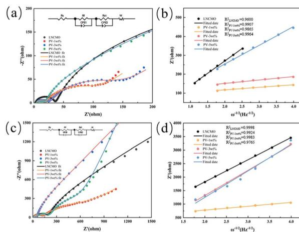
Fig. 10 EIS plots (a) before and (c) after 100 cycles. The profiles of  $Z'$  vs.  $\omega^{-1/2}$  (b) before cycling and (d) after 100 cycles.
