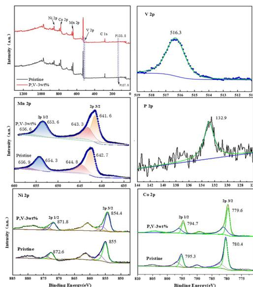
Fig. 7 XPS images of LNCMO and PV-3wt%.
