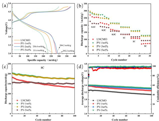
Fig. 8 (a) The initial charge–discharge profiles and (b) rate performance of LNCMO, PV-1wt%, PV-3wt%, and PV-5wt%. (c) Cycle performance of all samples at 1.0C. (d) The medium discharge voltage during cycling.
