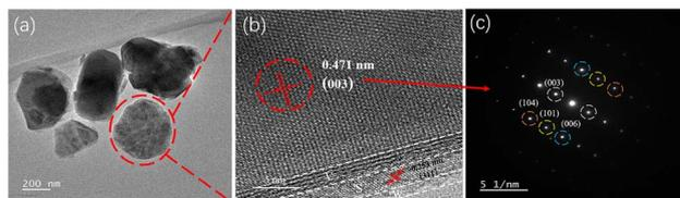
Fig. 6 (a) HRTEM image of PV-3wt% on 200 nm, (b) HRTEM images of different regions marked as V, S, W on 5 nm, and (c) corresponding Fast Fourier Transform (FFT).
