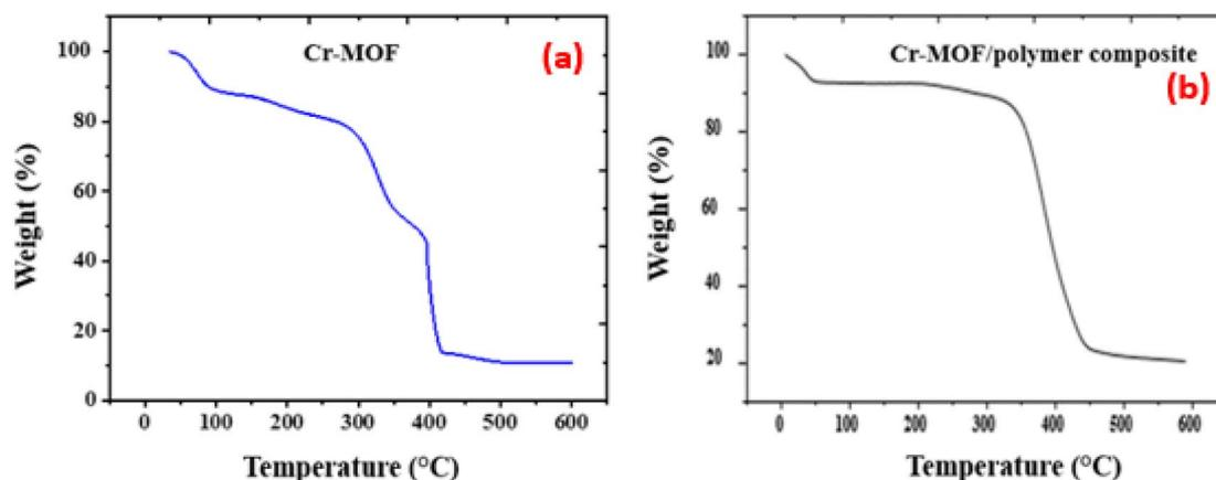
Fig. 5 Thermal stabilities of Cr-MOF (a) and Cr-MOF/polymer composite (b).
