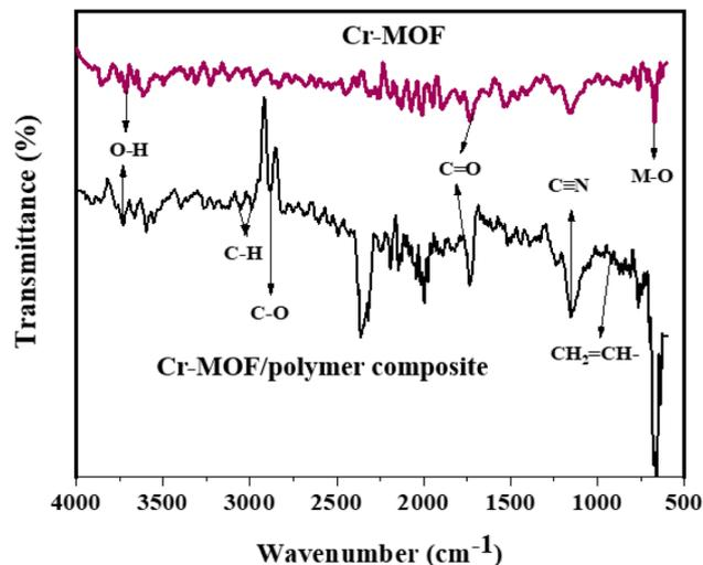
Fig. 2 FTIR spectra of Cr-MOF and Cr-MOF/polymer composite.
