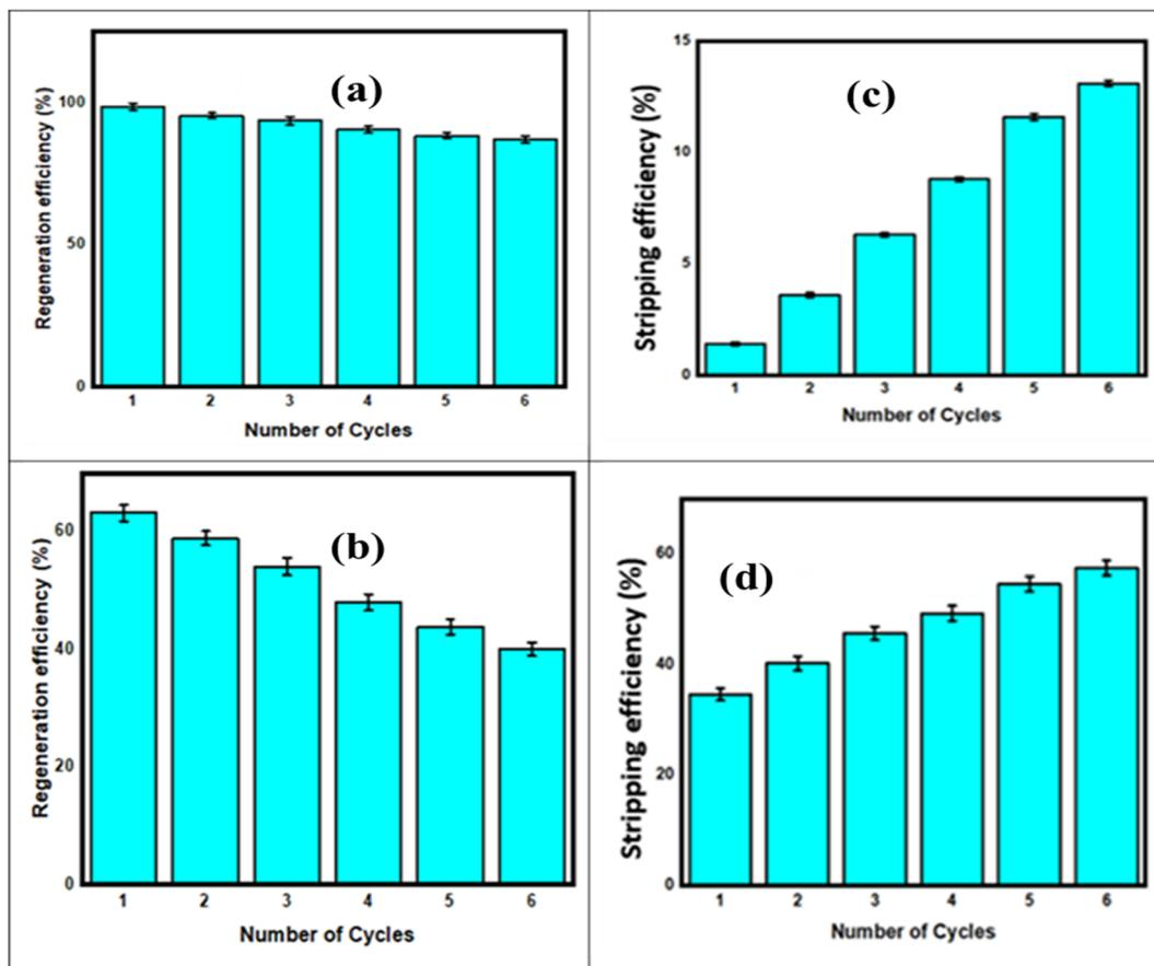
Fig. 10 (a) Regeneration efficiency of the Cr-MOF/polymer composite for spiked samples in water. (b) Stripping efficiency calculated using standard solutions of IMI in water. (c) Regeneration efficiency of the Cr-MOF/polymer composite for spiked samples in fish. (d) Stripping efficiency of the Cr-MOF/polymer composite for six continuous cycles for IMI in fish.
