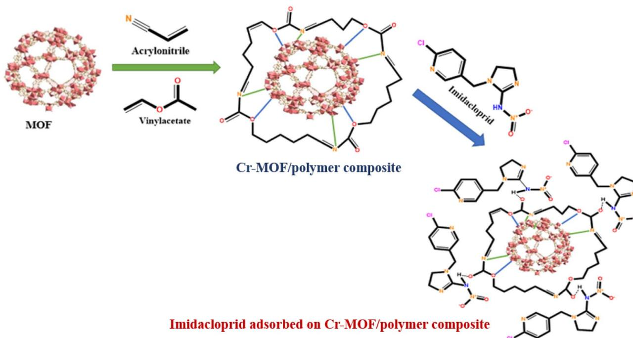
Fig. 1 Schematic of the synthesis of Cr-MOF/polymer composite, and its interaction with IMI.
