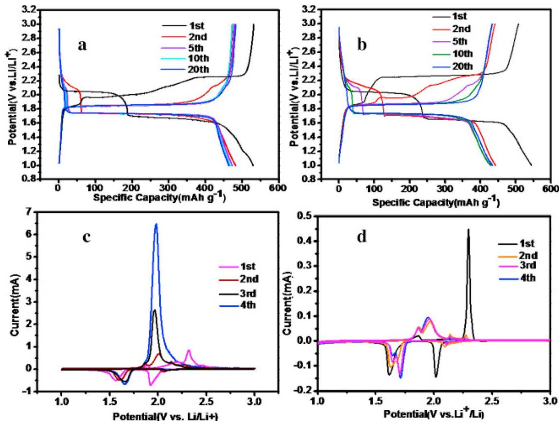
Fig. 8 Charge/discharge profiles of (a) copper sulfide and (b) CuS/rGO at a current density of  $100 \text{ mA g}^{-1}$ . Cyclic voltammetric curves of (c) CuS and (d) CuS/rGO between a  $V$  range of 1.0–3.0 V. This figure has been adapted from ref. 222 with permission from Elsevier, copyright 2016.
