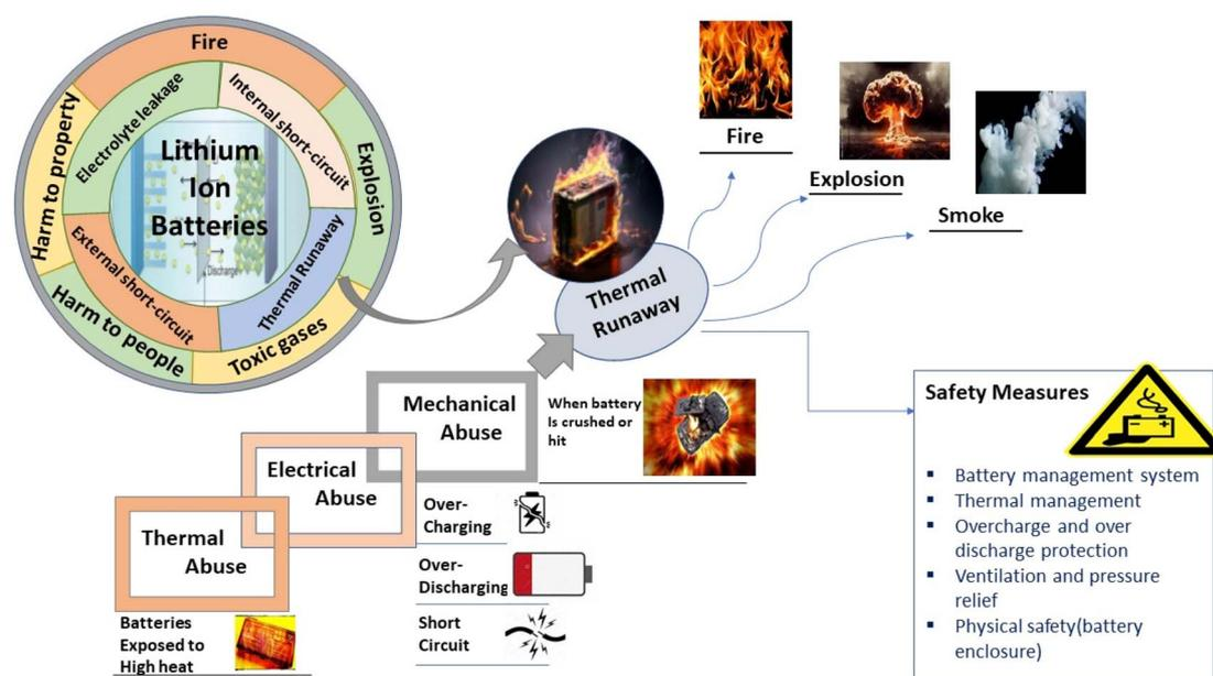
Fig. 13 Safety issues associated with Li-ion batteries.
