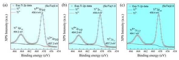
Fig. 10 XPS spectra of Ti 2p for ScTa-TO ceramics with Sc<sup>3+</sup>/Ta<sup>5+</sup> ratios of (a) 0.4. (b) 1.0. and (c) 2.0.
