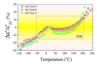
Fig. 8 Temperature coefficient of  $\varepsilon'$  at 1 kHz for ScTa-TO ceramics with Sc<sup>3+</sup>/Ta<sup>5+</sup> ratios of 0.4, 0.8, and 1.0.
