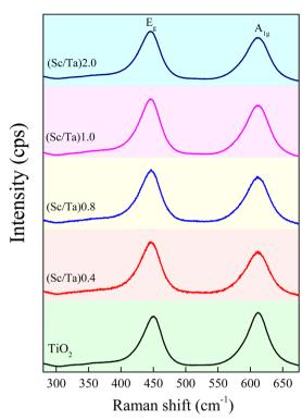
Fig. 5 Raman spectra of  $TiO_2$  and ScTa-TO ceramics with  $Sc^{3+}/Ta^{5+}$  ratios of 0.4, 0.8, 1.0, and 2.0.
