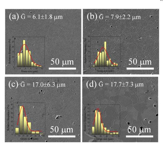
Fig. 2 SEM images of ScTa-TO ceramics with  $Sc^{3+}/Ta^{5+}$  ratios of (a) 0.4, (b) 0.8, (c) 1.0, and (d) 2.0
