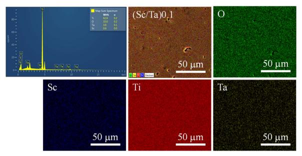
Fig. 3 EDS spectrum and SEM-mapping images of (Sc/Ta)1.0 ceramic.
