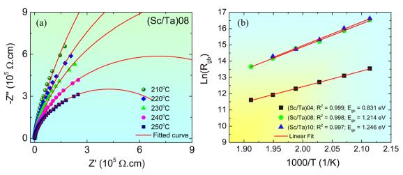
Fig. 11 (a)  $Z^*$  plots of (Sc/Ta)0.8 ceramic at different temperatures from 210 to 250 °C fitted by eqn (5). (b) Arrhenius plots of temperature dependence of  $R_{\rm qb}$  for (Sc/Ta)0.4, (Sc/Ta)0.8, and (Sc/Ta)1.0 ceramics.
