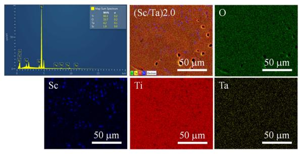
Fig. 4 EDS spectrum and SEM-mapping images of (Sc/Ta)2.0 ceramic.
