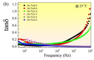
Fig. 6 Frequency dependence of (a)  $\varepsilon'$  and (b) tan  $\delta$  at 25 °C for ScTa-TO ceramics with Sc<sup>3+</sup>/Ta<sup>5+</sup> ratios of 0.4, 0.8, 1.0, 1.2, 1.6, and 2.0.
