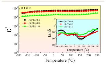
Fig. 7 Temperature dependence of  $\varepsilon'$  at 1 kHz for ScTa-TO ceramics with Sc<sup>3+</sup>/Ta<sup>5+</sup> ratios of 0.4, 0.8, and 1.0; inset shows  $\tan \delta$  at 1 kHz.
