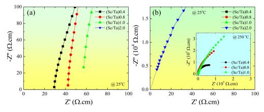
Fig. 9 (a) Impedance complex plane ( $Z^*$ ) plots at 25 °C for (Sc/Ta)0.4, (Sc/Ta)0.8, and (Sc/Ta)1.0 ceramics. (b)  $Z^*$  plot of (Sc/Ta)2.0 ceramic at 25 °C; inset shows  $Z^*$  plots at 250 °C for (Sc/Ta)0.4, (Sc/Ta)0.8, (Sc/Ta)1.0 ceramics.
