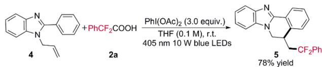
Scheme 2 Construction of the  $\text{PhCF}_2$ -substituted benzimidazole-dihydroisoquinoline.
