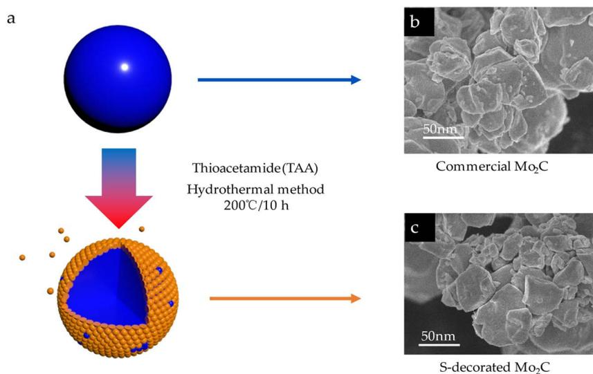
Fig. 1 (a) Schematic synthesis process of S-decorated Mo<sub>2</sub>C; (b) the SEM image of commercial Mo<sub>2</sub>C; (c) the SEM image of S@Mo<sub>2</sub>C.
