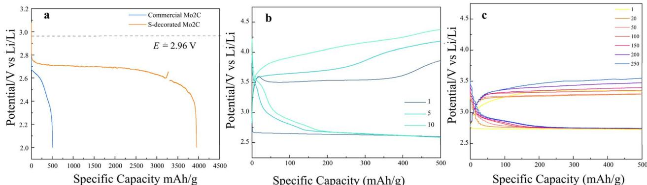
Fig. 5 (a) Voltage profile of the full discharge for commercial Mo<sub>2</sub>C and S@Mo<sub>2</sub>C in Li–O<sub>2</sub> batteries; (b) charge and discharge curves of commercial Mo<sub>2</sub>C at a current density of 100 mA g<sup>-1</sup>; (c) charge and discharge curves of S@Mo<sub>2</sub>C at a current density of 100 mA g<sup>-1</sup>.
