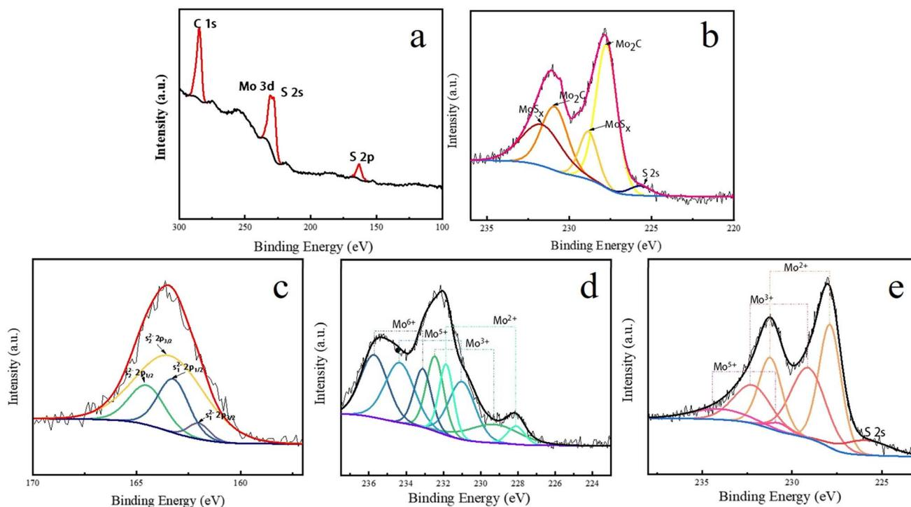
Fig. 4 (a and b) XPS images of S@Mo<sub>2</sub>C sample; (c) XPS spectra of S element of S@Mo<sub>2</sub>C; (d and e) XPS images of different ion valences of Mo element in commercial Mo<sub>2</sub>C and S@Mo<sub>2</sub>C.
