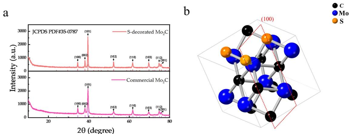
Fig. 2 (a) XRD patterns of commercial Mo<sub>2</sub>C and S-decorated Mo<sub>2</sub>C; (b) crystal structure of S-decorated Mo<sub>2</sub>C.
