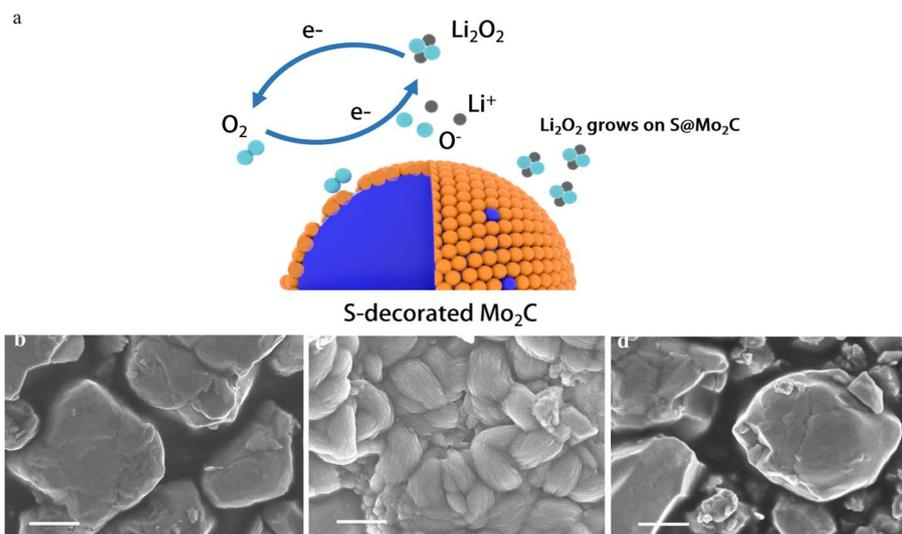
Fig. 6 (a) The schematic diagram of S@Mo<sub>2</sub>C electrode Li–O<sub>2</sub> battery; (b) pristine S@Mo<sub>2</sub>C cathode with uniform nanoparticles. (c) post-discharge: toroidal Li<sub>2</sub>O<sub>2</sub> and amorphous Li<sub>2</sub>O<sub>2</sub> deposited on the surface. (d) Post-recharge: complete decomposition of Li<sub>2</sub>O<sub>2</sub>, restoring the cathode morphology. The (c) and (d) two figures are TEM images after 250 cycles.
