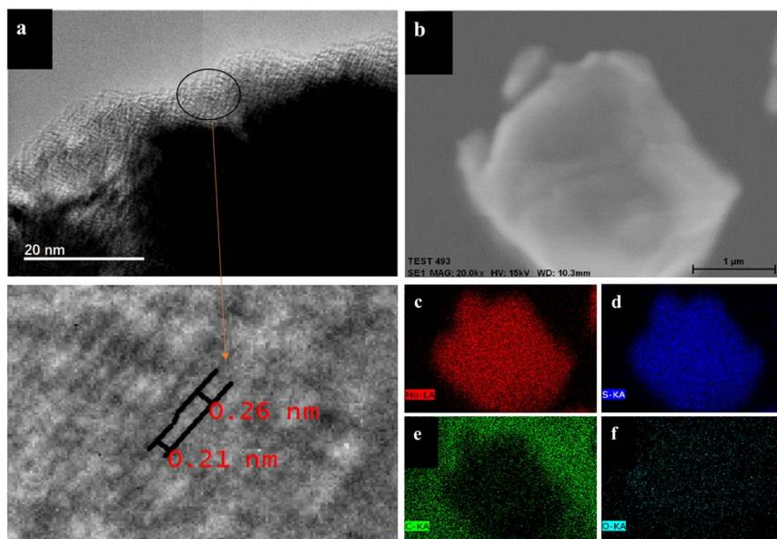
Fig. 3 (a) The TEM and magnified STEM images of S-decorated Mo<sub>2</sub>C; (b–f) elemental mapping analysis of S-decorated Mo<sub>2</sub>C.
