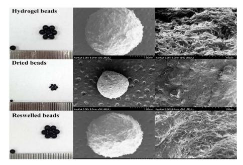
Fig. 6 Morphology of composite beads of Alg/AC/CMC (4%, 1%, 1%).41
