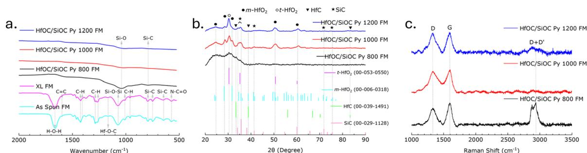
**Fig. 5** (a) The FTIR spectra of HfOC/SiOC ceramic fiber mats pyrolyzed at 800, 1000, and 1200 °C, including as-spun and crosslinked fiber mat samples, represent the gradual disappearance of H-containing functional groups. (b) Their XRD pattern, including comparable JCPDS card numbers, represents an increase in crystallinity with the increase of pyrolysis temperature. (c) Their Raman spectra indicate evolution of the free carbon phase as a function of pyrolysis temperature.
