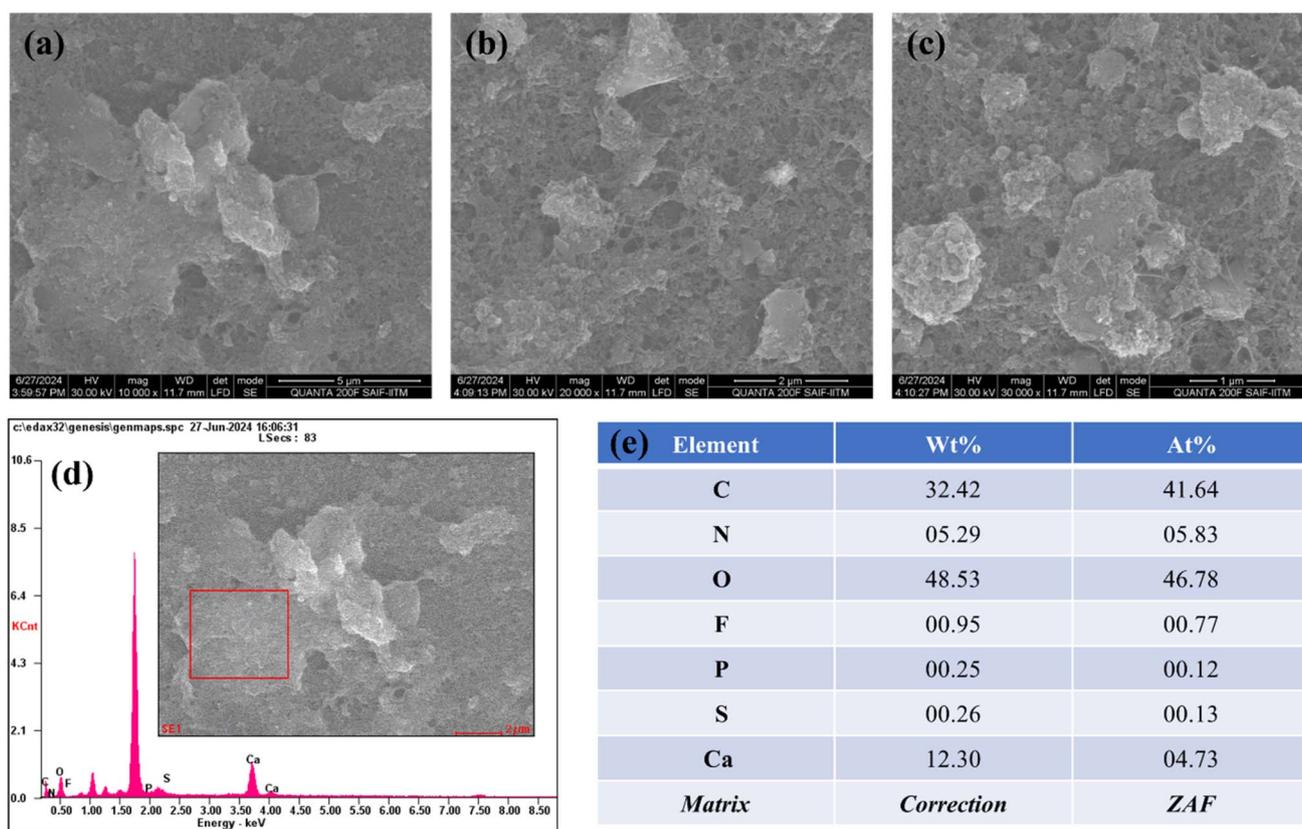
Fig. 1 HRSEM images of FAD/FA/SWCNT at 5  $\mu\text{m}$  (a), 2  $\mu\text{m}$  (b), and 1  $\mu\text{m}$  (c) resolutions. (d) Energy-dispersive spectrum (EDS) (inset: a scanned area for the analysis) and (e) the weight ratio of elements presents in FAD/FA/SWCNT composite.
