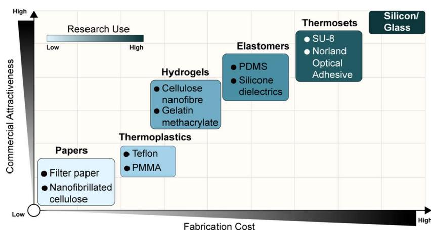
Fig. 8 The most promising materials for microfluidic chip fabrication and comparison of the resulting devices' cost.<sup>191</sup>
