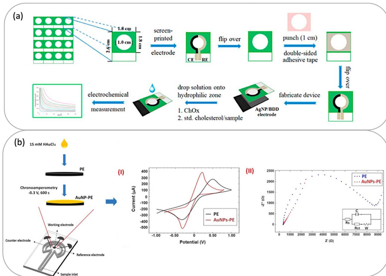
Fig. 12 (a) Schematic representation of the fabrication and analytical procedure for the cholesterol sensor based on the coupling of the AgNP/BDD electrode with  $\mu$ PAD. This figure has been adapted from ref. 233 with permission from Elsevier, copyright 2015. (b) Sketch of the AuNPs modified paper electrode sensing system, (i) CVs of PE and AuNP-PE, (ii) Nyquist diagrams of PE and AuNP-PE. This figure has been adapted from ref. 234 with permission from Elsevier, copyright 2021.
