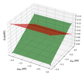
Fig. 10 Surface formation energy  $(\Omega)$  vs.  $\mu_{Mn}$  and  $\mu_{As}$  chemical potentials in eV Å<sup>-2</sup> (green plane represents the MnNa-terminated surface and the red one defines the As-terminated surface; black line in the stability map defines the region where the stability change happens).
