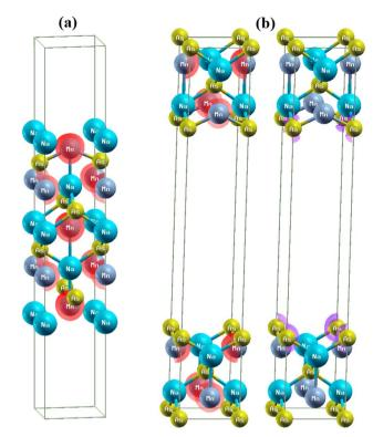
Fig. 8 Spin density (iso-surface value:  $0.1 \, e \, \mathring{A}^{-3}$ ; red surface: spin-up; violet surface: spin-down) in (a) MnNa- and (b) As-terminated (001) surface of the NaMnAs half-Heusler compound with 9ML thickness.
