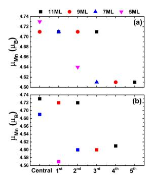
Fig. 9 Local magnetic moment of Mn atoms in different layers of (a) MnNa- and (b) As-terminated (001) surfaces of the NaMnAs half-Heusler compound with 11ML, 9ML, 7ML, and 5ML thickness.
