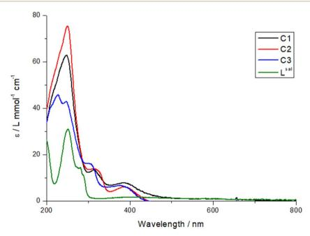
Fig. 3 UV-vis spectra of complexes C1–C3 in acetonitrile at room temperature.
