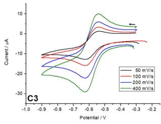
Fig. 7 Scan rate studies of catecholate to semiquinolate redox process for complex C3.
