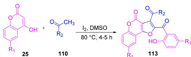
Scheme 72 Furo[3,2- c ]coumarin 113 synthesis via in situ -generated phenyl glyoxal.
