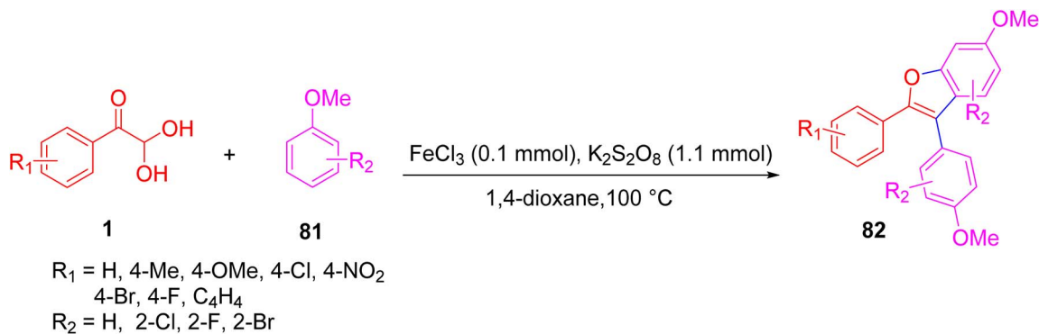
Scheme 41 Synthesis of benzofuran 82 via an FeCl 3 -mediated intermolecular tandem reaction.
