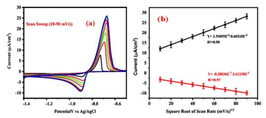
Fig. 12 (a) Scan rate impact on the redox reaction of Pb<sup>2+</sup>. (b) Anodic peak current response plot with  $R^2 = 0.98$  and  $R^2 = 0.97$  for the redox peak current response plot with changing the scan rate from 10 to 90 mV s<sup>-1</sup>.
