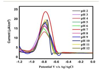
Fig. 11 DPV responses of Bi $_2$ O $_3$ /IL/rGO/GC to 20  $\mu$ M Pb $^{2+}$  in 0.1 M phosphate at different pH values ranging from 2.0–12.0.
