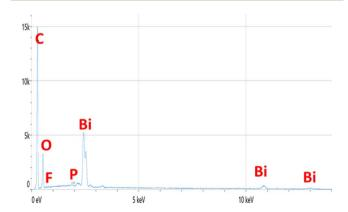
Fig. 6 Energy-dispersive X-ray (EDX) spectrum of the  ${\rm Bi}_2{\rm O}_3/{\rm IL/rGO}$  nanocomposite.
