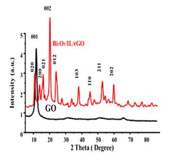
Fig. 4 X-ray diffraction (XRD) patterns of graphene oxide (GO) and the  ${\rm Bi}_2{\rm O}_3/({\rm IL/rGO})$  nanocomposite.
