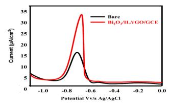
Fig. 9 DPV response of the bare/GCE and  $Bi_2O_3/IL/rGO/GCE$  in the presence of 20  $\mu$ M lead  $Pb^{2+}$ .
