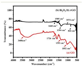
Fig. 3 (a) FTIR spectrum of GO and (b) FTIR spectrum of Bi<sub>2</sub>O<sub>3</sub>/IL/rGO. Bi<sub>2</sub>O<sub>3</sub>/(IL/rGO) nanocomposite.
