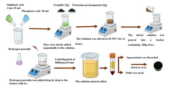
Fig. 1 Graphical representation of the graphene oxide (GO) synthesis using Hummer's method.
