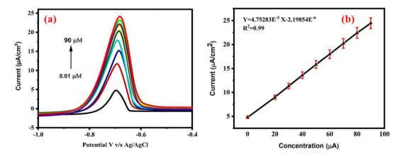
Fig. 13 (a) DPV-based calibration current response to  $Pb^{2+}$  for concentrations ranging from 0.01 to 90  $\mu$ M; (b) linearity of calibration, with  $R^2 = 0.99$ .
