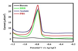
Fig. 10  $\,$  Ipa responses to 20  $\mu$ M Pb<sup>2+</sup> in different electrolytic systems ranging from acidic to basic pH.
