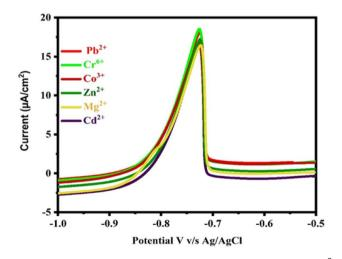
Fig. 14 Effect of interfering substances on Ipa response to 20  $\mu$ M Pb<sup>2+</sup> in 0.1 M PBS (pH 7.0).
