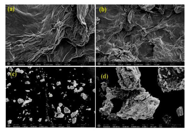
Fig. 5 (a) and (b) Scanning electron microscopy (SEM) images of graphene oxide (GO) and (c) and (d) SEM images of the  $Bi_2O_3/IL/rGO$  nanocomposite.
