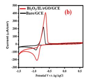
Fig. 7 (a) and (b) EIS and CV responses of bare GCE and  $Bi_2O_3/IL/rGO/GCE$  in 0.5 mM ( $K_4Fe(CN)_6$ ) and 0.1 M KCL.
