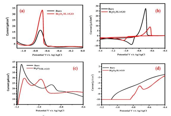
Fig. 8 Electrochemical responses of  $Pb^{2+}$  at a concentration of 20  $\mu$ M evaluated using various voltammetric techniques: (a) differential pulse voltammetry (DPV), (b) square wave voltammetry (SWV), (c) linear sweep voltammetry (LSV), and (d) cyclic voltammetry (CV).
