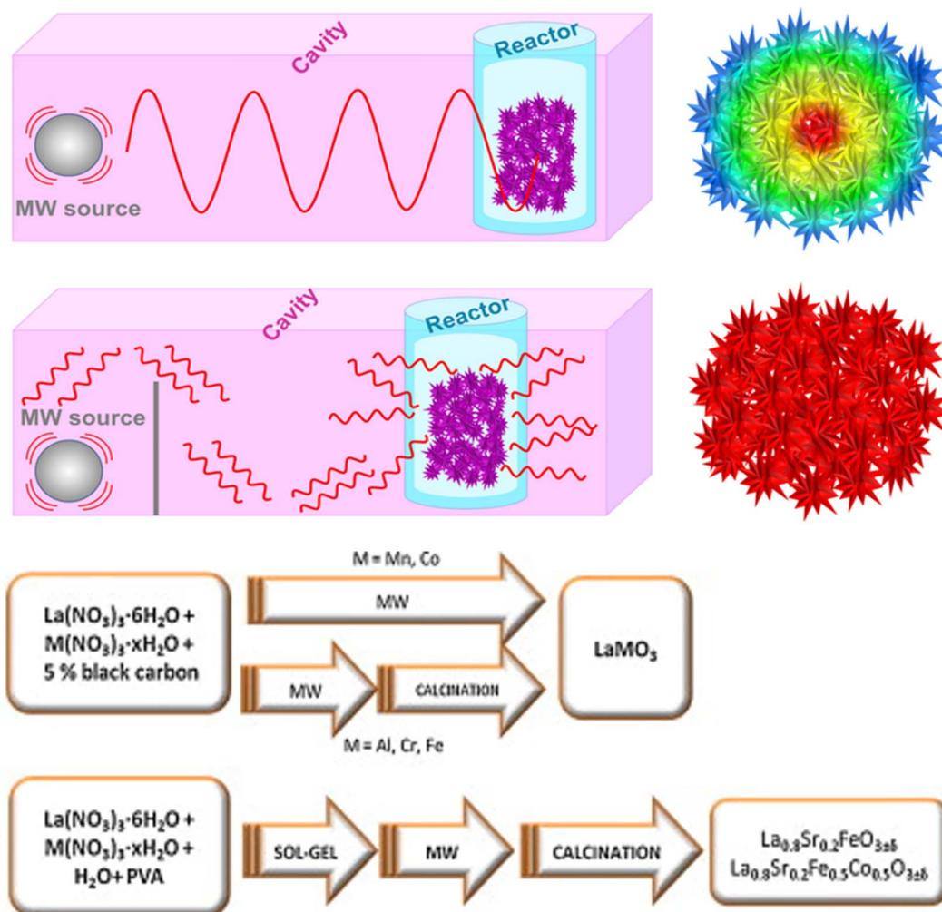
Fig. 7 Schematic representation of the microwave synthesis method.<sup>74,75</sup> This figure has been reproduced from ref. 74 and 75 with permission from RSC, copyright 2025.
