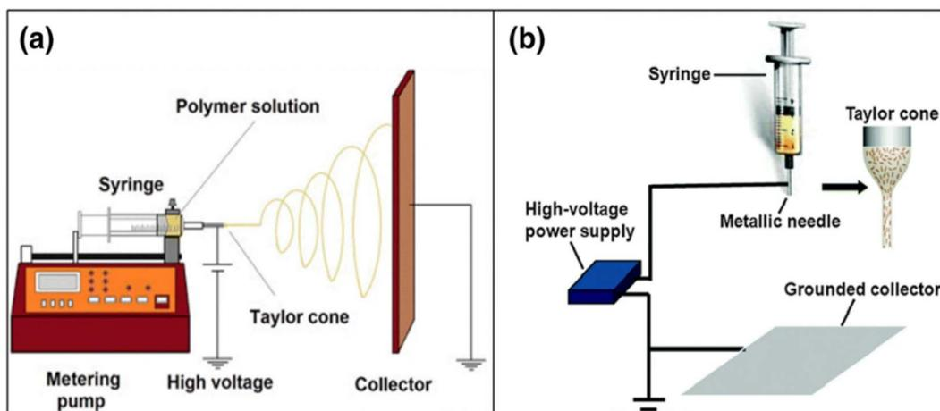
Fig. 11 Schematic diagram of set up of electrospinning apparatus (a) horizontal set up and (b) vertical setup.<sup>98</sup> This figure has been reproduced from ref. 98 with permission from Elsevier, copyright 2025.
