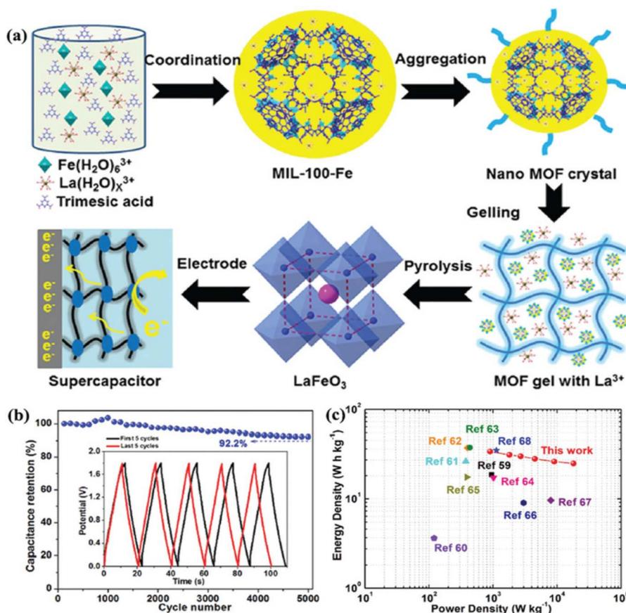
Fig. 14 (a) Schematic representations illustrating the synthesis of perovskite  $\text{LaFeO}_3$ . (b) Graph showing cycling stability versus cycle number, inset: the first and last five GCD cycles. (c) Ragone plots (energy density vs. power density) of this study and other devices at  $2 \text{ A g}^{-1}$ .<sup>138</sup> This figure has been reproduced from ref. 138 with permission from RSC, copyright 2025.
