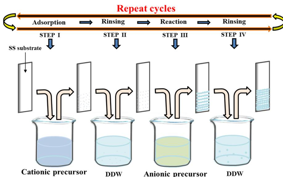
Fig. 10 Schematic representation of SILAR method.<sup>94</sup> This figure has been reproduced from ref. 94 with permission from Elsevier, copyright 2025.
