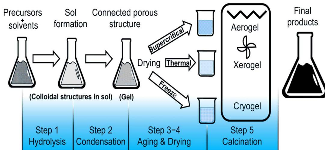
Fig. 8 Schematic representation of POs by the sol-gel method.<sup>80</sup> This figure has been reproduced from ref. 80 with permission from Elsevier, copyright 2025.
