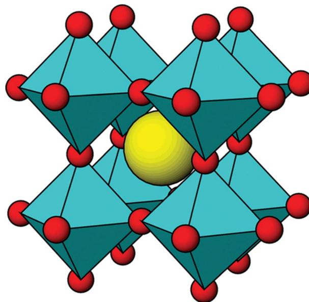
Fig. 1 Ideal cubic perovskite structure for  $ABO_3$  ( $BO_6$  units – cyan; A atoms – yellow; O atoms – red).<sup>38</sup> This figure has been reproduced from ref. 38 with permission from *Frontiers in Chemistry*, copyright 2025.
