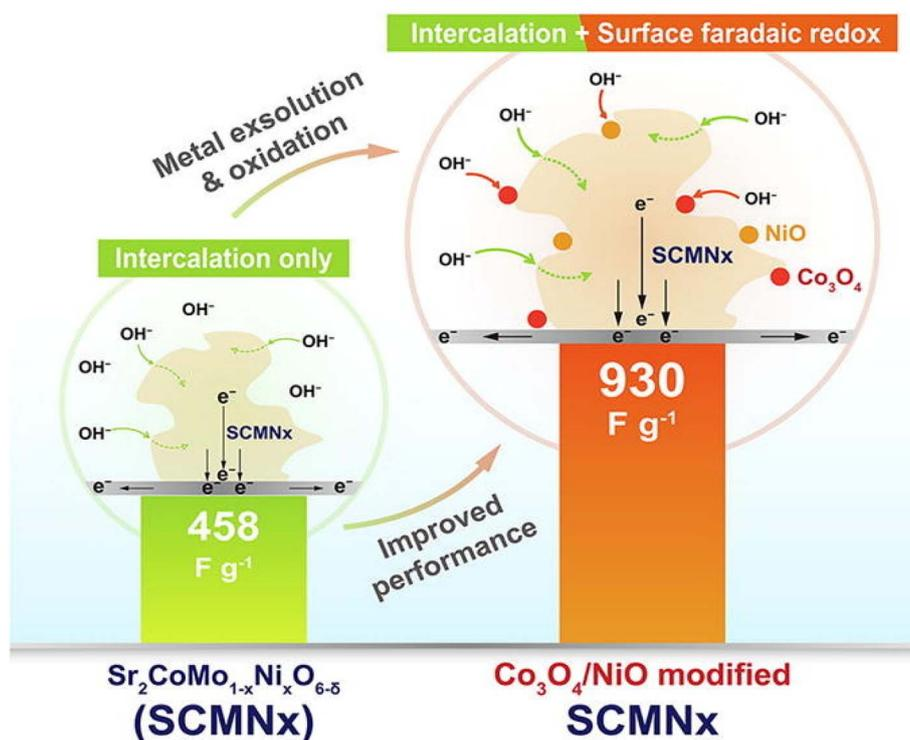
Fig. 5 Charge storage mechanism of  $\text{Sr}_2\text{CoMo}_{1-x}\text{Ni}_x\text{O}_{6-\delta}$ .<sup>65</sup> This figure has been reproduced from ref. 65 with permission from Elsevier, copyright 2025.
