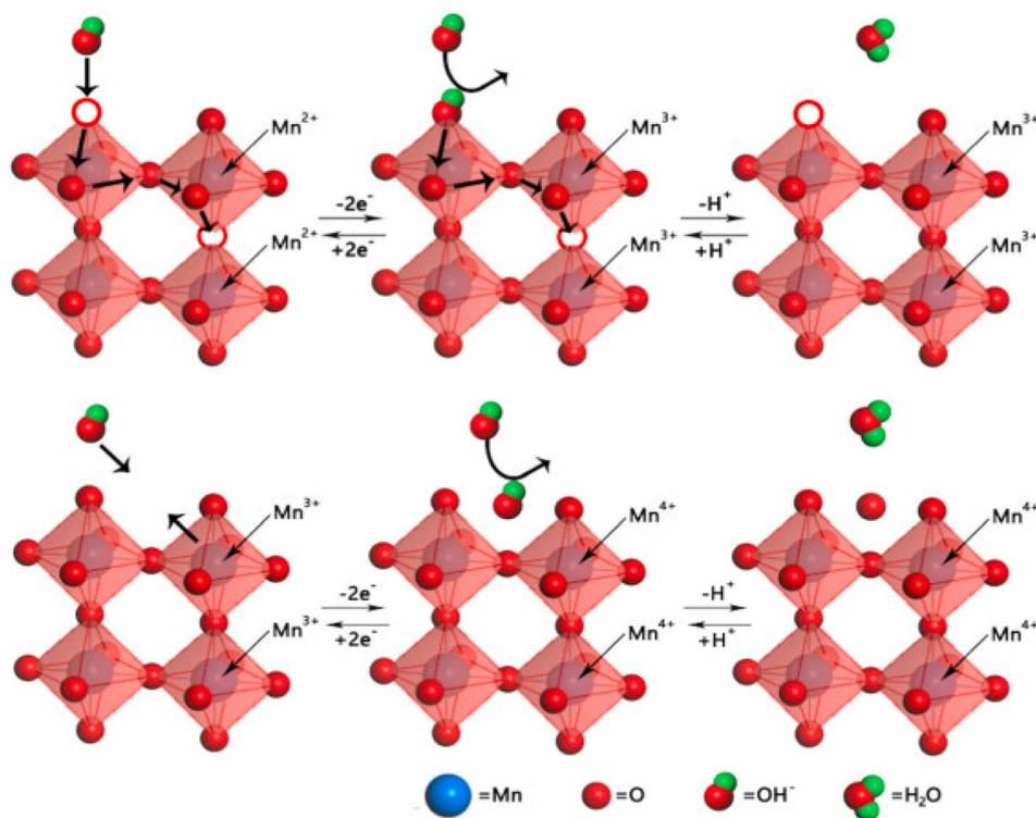
Fig. 6 Schematic illustration of oxygen intercalation mechanism in PO.<sup>70</sup> This figure has been reproduced from ref. 70 with permission from Elsevier, copyright 2025.
