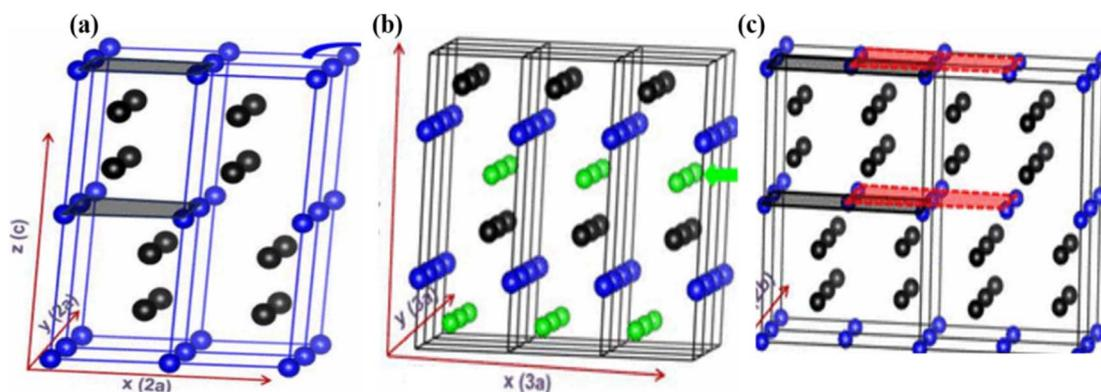
Fig. 4 Schematic representation of (a) 6H-A and (b) 6H-B and (c) orthorhombic crystal systems.<sup>61,62</sup> This figure has been reproduced from ref. 61 and 62 with permission from RSC, copyright 2025.
