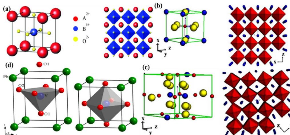
Fig. 2 Different structures of perovskite material (a) cubic, (b) monoclinic, (c) orthorhombic and (d) tetragonal.<sup>41,42</sup> This figure has been reproduced from ref. 41 and 42 with permission from Elsevier, copyright 2025.
