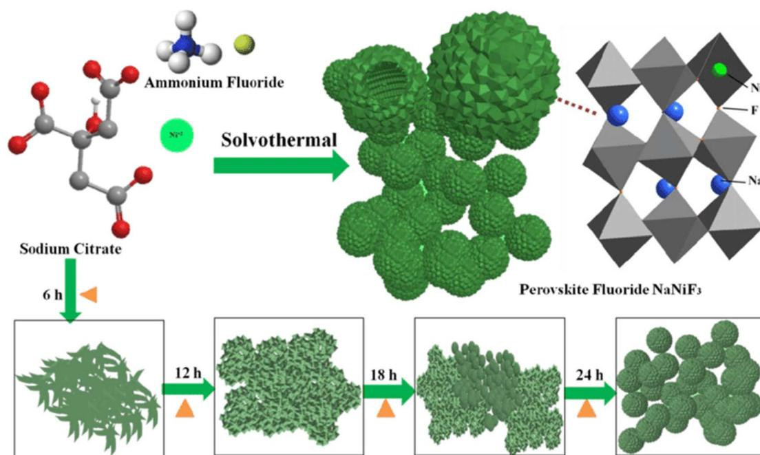
Fig. 9 Synthesis process of hollow spherical  $\text{NaNiF}_3$  perovskite fluoride nanocrystals.<sup>90</sup> This figure has been reproduced from ref. 90 with permission from Wiley, copyright 2025.
