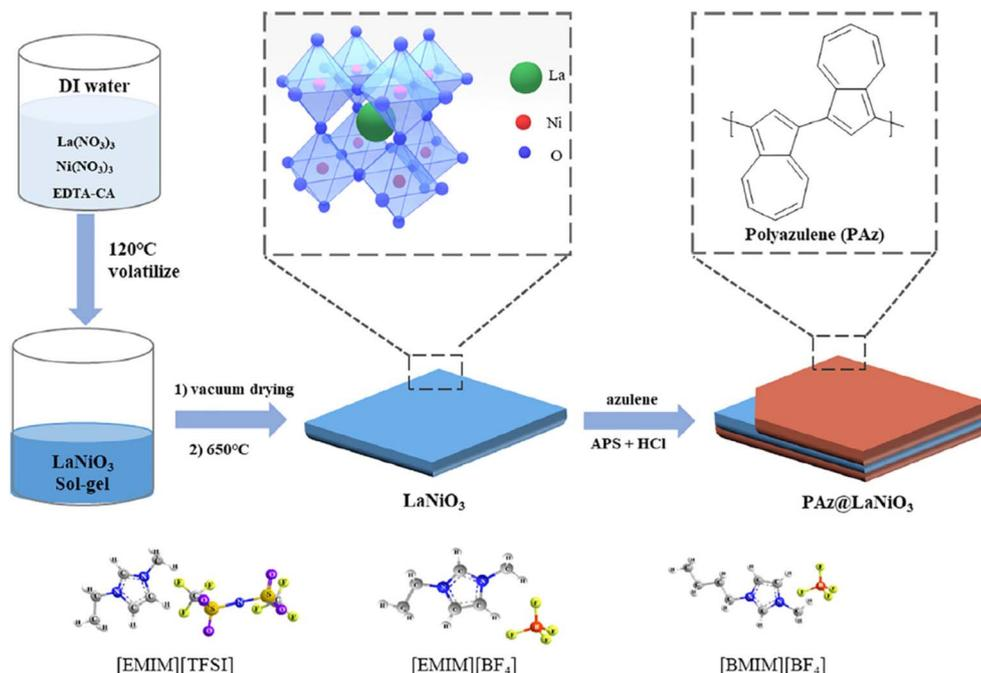
Fig. 15 Schematic representation of the preparation of PAz@LaNiO<sub>3</sub> nanosheets.<sup>195</sup>
