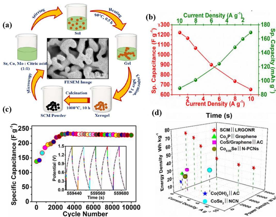
Fig. 12 (a) Schematic representation of the synthesis process of SCM. (b) GCD curves of the SCM electrode at varying current densities. (c) Cycling stability of the ASC at  $10 \text{ A g}^{-1}$ . The inset displays the final five GCD cycles. (d) Ragone plot of a hybrid SCM cell compared with literature findings.<sup>98</sup> This figure has been reproduced from ref. 98 with permission from Elsevier, copyright 2025.
