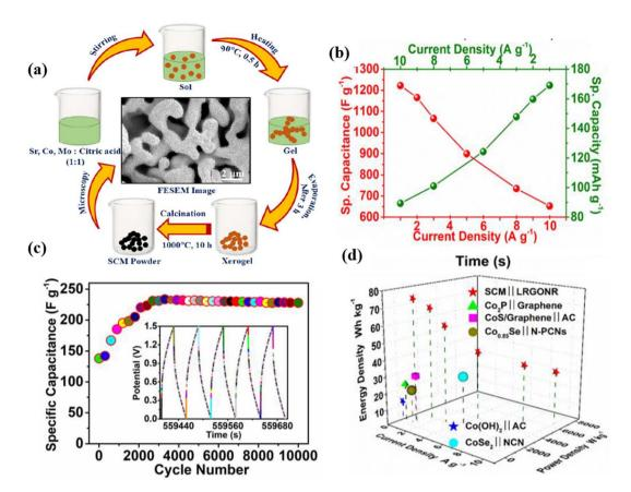
Fig. 12 (a) Schematic representation of the synthesis process of SCM. (b) GCD curves of the SCM electrode at varying current densities. (c) Cycling stability of the ASC at  $10 \text{ A g}^{-1}$ . The inset displays the final five GCD cycles. (d) Ragone plot of a hybrid SCM cell compared with literature findings. This figure has been reproduced from ref. 98 with permission from Elseiver, copyright 2025.
