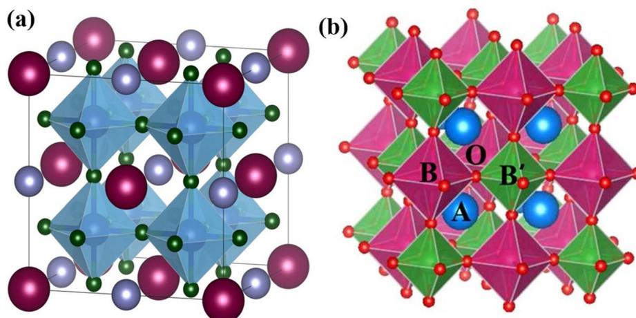
Fig. 3 Schematic illustration of (a)  $A'A''BO_6$  (double A site), (b)  $AB'B''O_6$  (double B site).<sup>46,47</sup> This figure has been reproduced from ref. 46 and 47 with permission from RSC, copyright 2025.
