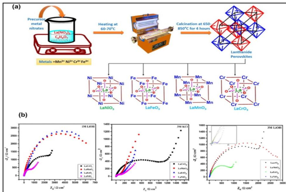
Fig. 13 (a) Synthesis procedure for four types of different perovskite oxide powders ( $\text{LaMnO}_3$ ,  $\text{LaFeO}_3$ ,  $\text{LaCrO}_3$ , and  $\text{LaNiO}_3$ ) for application as SC anode materials using the sol–gel method. (b) EIS of the four perovskite materials in various electrolyte solutions.<sup>107</sup> This figure has been reproduced from ref. 107 with permission from Elsevier, copyright 2025.
