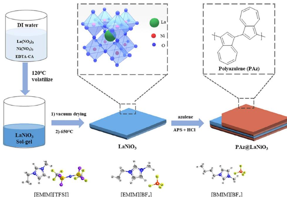
Fig. 15 Schematic representation of the preparation of PAz@LaNiO<sub>3</sub> nanosheets.<sup>195</sup>
