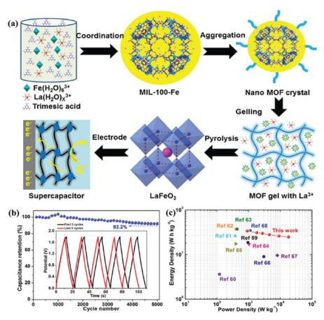
Fig. 14 (a) Schematic representations illustrating the synthesis of perovskite LaFeO<sub>3</sub>. (b) Graph showing cycling stability *versus* cycle number, inset: the first and last five GCD cycles. (c) Ragone plots (energy density vs. power density) of this study and other devices at 2 A  $g^{-1}$ . This figure has been reproduced from ref. 138 with permission from RSC, copyright 2025.
