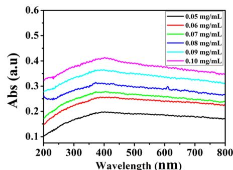
Fig. 7 UV-vis absorption of C<sub>4</sub>@NpFeSi nanoparticles.
