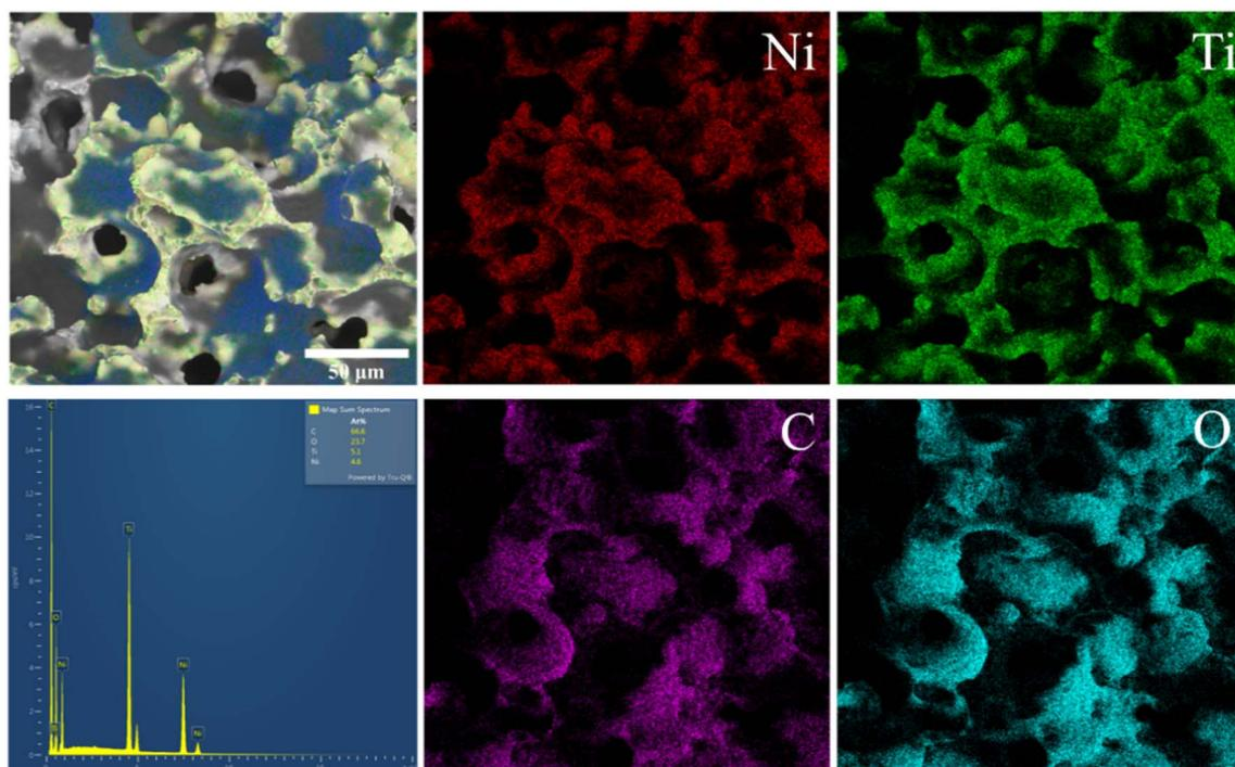
**Fig. 6** EDS spectrum and elemental mapping reveal distinct carbon (C) and oxygen (O) enrichment within the pore interiors, in contrast to the bulk NiTi matrix. This localized C/O distribution corresponds to the black hydrogel residues observed in the SEM images, confirming successful hydrogel retention within the pores during loading. The Ni/Ti ratio remained homogeneous throughout the porous architecture, demonstrating the preservation of structural integrity without elemental segregation.
