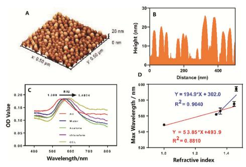
Fig. 2 (A) Microscopy (AFM) image of glass coated with gold NPs. (B) Line profile analysis of AFM image of gold NPs. (C) Sensitivity test of annealed NPs in air (n = 1), dd-water (n = 1.33), acetone (n = 1.36), chloroform (n = 1.44), and carbon tetrachloride (n = 1.46). (D) Linear fitting for different environments RI on gold NPs.
