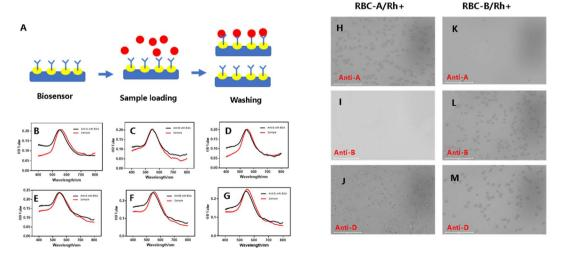
Fig. 4 LSPR-based detection for blood typing and in standard RBCs-A and -B samples. (A) Scheme showing the mechanism of the LSPR-based blood typing biosensor. (B-G) LSPR spectra of standard RBCs-A and -B samples on different antibodies binding gold NPs and their corresponding optical microscope photo (H-M).
