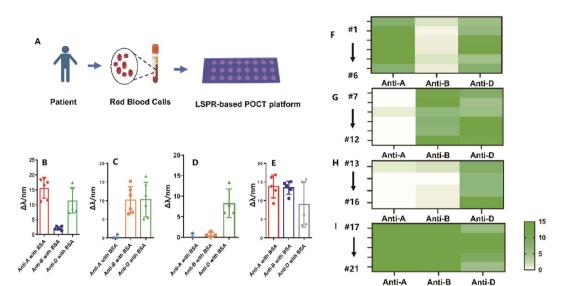
Fig. 6 Blood typing in patient samples on POCT platform. (A) Workflow of the on-chip testing based on the spectrometer readout. (B–E) LSPR red-shift showing the on-chip testing results of the 21 clinical samples. (F–I) Heatmap of the LSPR red-shift of the images in (B).
