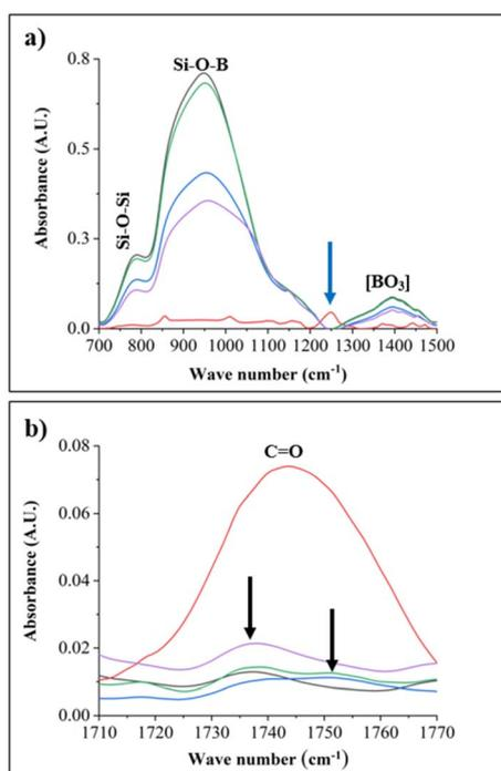
Fig. 5 FT-IR spectra of crude PECA (red), 60H40T30p (blue); sample 40H60T30p (green) sample 20H80t50p (purple) and a pristine pre-treated glass slide (black). (a) Highlights prominent absorption spectra on the glass substrates despite the PECA-FNS coating, while (b) displays the C=O stretching band indicative of the PECA polymer.
