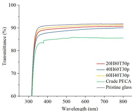
Fig. 7 Transmittance spectra measured from 300–800 nm: crude PECA (green), sample 60H40T30p (yellow), sample 40H60T30p (blue), 80H20T50p (red), and a pristine pre-treated glass slide (purple).
