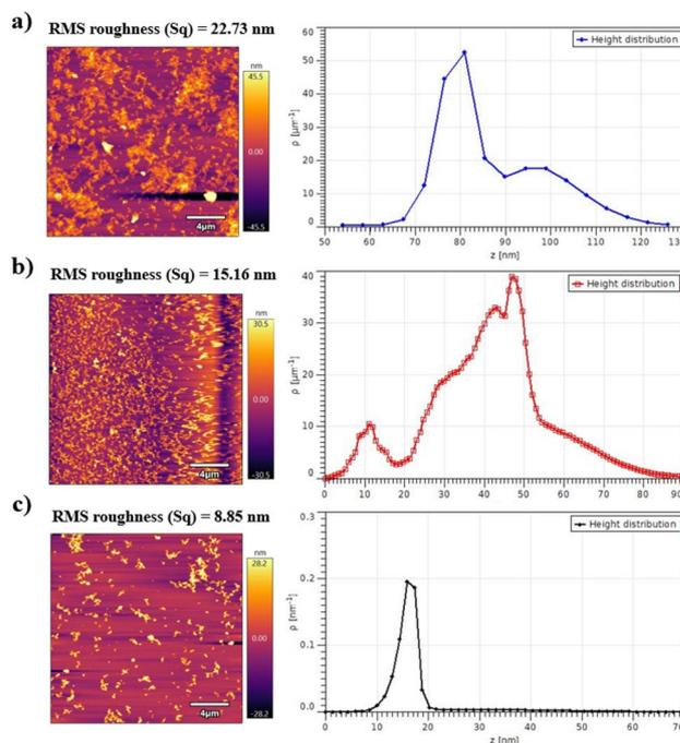
Fig. 6 AFM top-view images ( $20\text{ }\mu\text{m} \times 20\text{ }\mu\text{m}$ ) (on the left) and their corresponding height distribution histogram represented by the surface features  $\rho$  ( $\mu\text{m}^{-1}$ ) against the height  $z$  (nm): (a) sample 60H40T30p, (b) sample 40H60T30, and (c) sample 20H80T50p.
