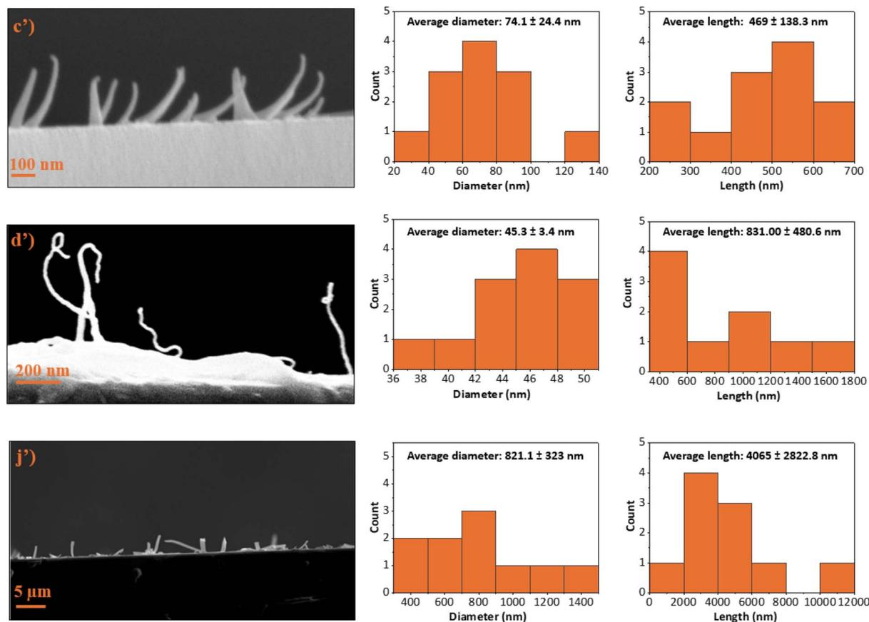
Fig. 3 SEM side-view of the different PECA-FNS (on the left) and their corresponding diameter and length histograms (on the right starting from the top to the bottom): (c') sample 60H40T30p, (d') sample 40H60T30p, and (j') sample 20H80T50p.
