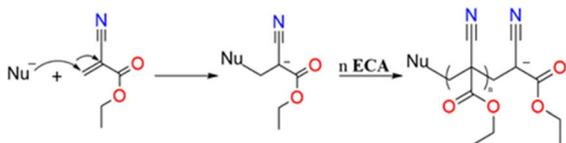
**Scheme 1** Anionic polymerisation of ECA in the presence of a nucleophile, for example a water molecule.
