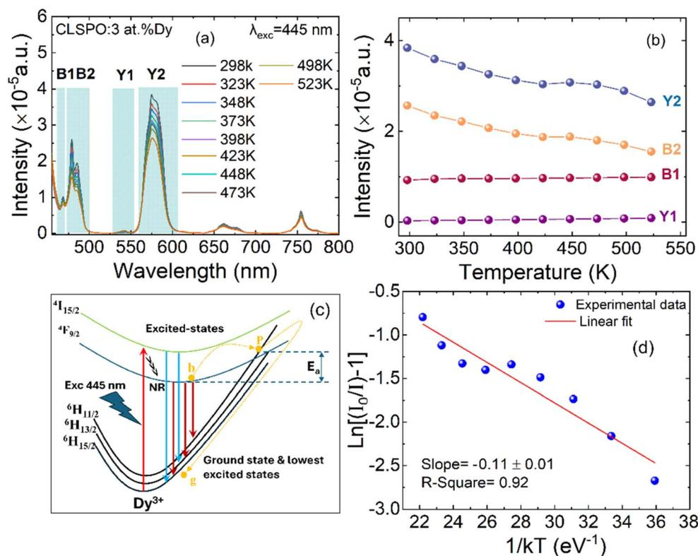
Fig. 10 (a) Photoluminescence spectra; (b) photoluminescence intensities of blue and yellow emissions from CLSPO:3 at%  $\text{Dy}^{3+}$  phosphors as a function of temperature over a temperature range from 298 K to 523 K; (c) configurational coordinate diagram illustrating the thermal quenching mechanism in CLSPO: $\text{Dy}^{3+}$  phosphors; (d) evaluation of the activation energy using an Arrhenius-type activation model for CLSPO:3 at%  $\text{Dy}^{3+}$  phosphors.
