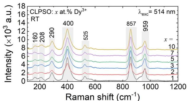
Fig. 4 Raman spectra for CLPSO:  $x$  at% Dy<sup>3+</sup> with  $x = 1, 2, 3, 5, 7$  and  $10$ .
