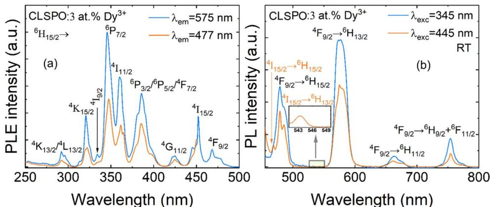
Fig. 6 (a) Excitation spectra of CLSPO:3 at.% Dy<sup>3+</sup> phosphor with emission wavelength  $\lambda_{em}$  monitored at 575 and 477 nm; (b) emission spectra under the pumping  $\lambda_{exc}$  of 345 nm and 445 nm.
