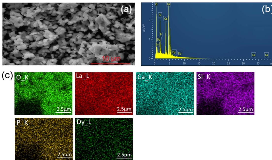
Fig. 3 (a) SEM image (b) EDX spectra and (c) elemental mapping for the CLPSO:3 at% Dy<sup>3+</sup> phosphors.
