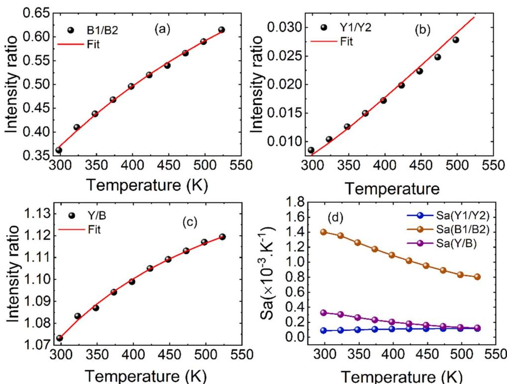
Fig. 12 Luminescence intensity ratio of (a)  $B_1/B_2$ , (b)  $Y_1/Y_2$ , and (c)  $Y/B$  in CLSPO:3 at%  $Dy^{3+}$  phosphors as a function of temperature; (d)  $S_a$  as a function of temperature for the three luminescence intensity ratios in CLSPO:3 at%  $Dy^{3+}$  phosphors.
