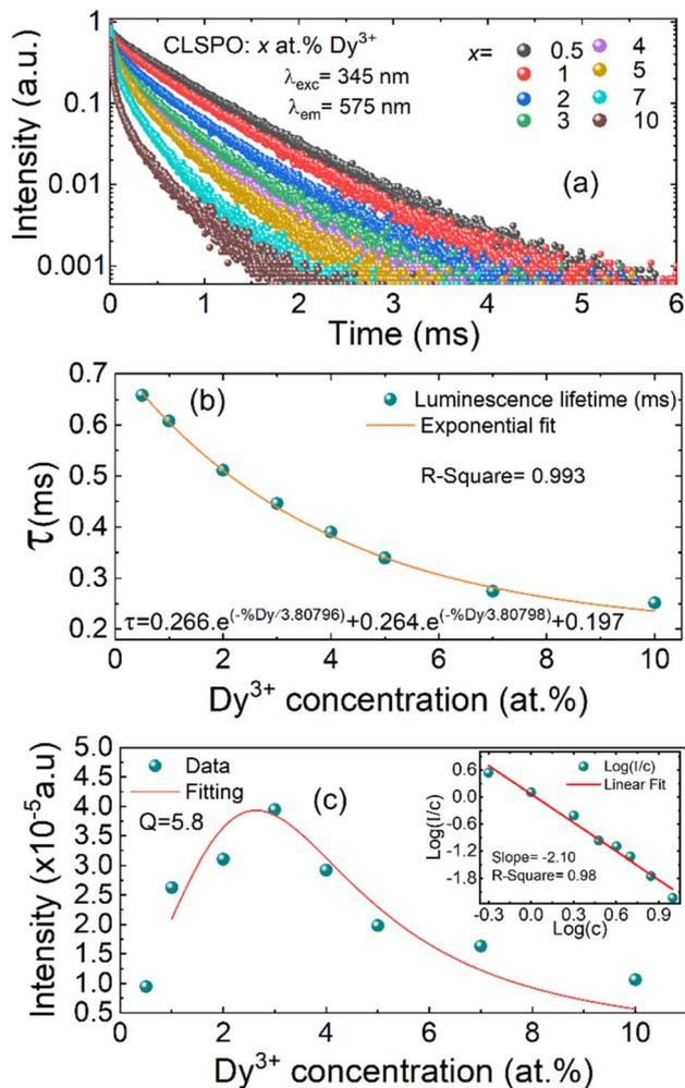
Fig. 9 (a) Decay curves for CLSPO: $x\text{Dy}^{3+}$  ( $x = 0.5, 1, 2, 3, 4, 5, 7$  and 10 at%), with excitation at 345 nm and emission at 575 nm; (b) exponential fit of the average decay lifetime to the concentration level of the  $\text{Dy}^{3+}$  ion; (c) variation of  $Y_2$  with  $\text{Dy}^{3+}$  concentration in CLSPO: $\text{Dy}^{3+}$  phosphors; (the inset displays a plot of  $\log(I/c)$  versus  $\log(c)$ ).
