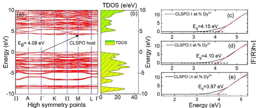
Fig. 5 (a) Bandgap structure of CLSPO host *via* density functional theory (DFT) calculation and (b) the corresponding calculated TDOS; bandgap values obtained *via* the K–M function for: (c) CLSPO:1 at% Dy<sup>3+</sup>; (d) CLSPO:3 at% Dy<sup>3+</sup>; and (e) CLSPO:10 at% Dy<sup>3+</sup>.
