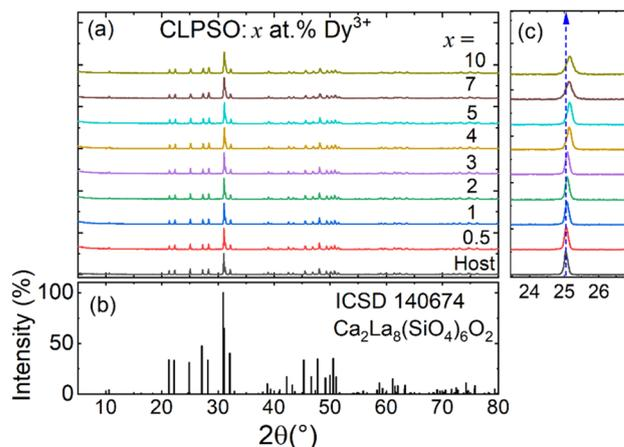
Fig. 1 (a) XRD patterns for the CLSPO doped with different concentrations of  $\text{Dy}^{3+}$  ions; (b) reference plot downloaded from ICSD database, file number 140674, for the apatite compound  $\text{Ca}_2\text{La}_8(\text{SiO}_4)_6\text{O}_2$ ; (c) variation of the position of the diffraction peak of the (002) plan as function of  $\text{Dy}^{3+}$  ions concentration.
