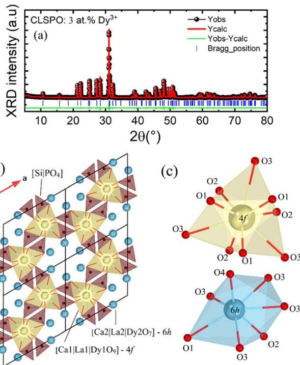
Fig. 2 (a) Refinement plots of CLSPO:3 at%  $\text{Dy}^{3+}$  sample; (b) view of the crystal structure of CLSPO: $\text{Dy}^{3+}$  phosphor along  $a$ - $b$  crystallographic plan; (c) oxygen atoms environment around the two cationic sites 4f and 6h.
