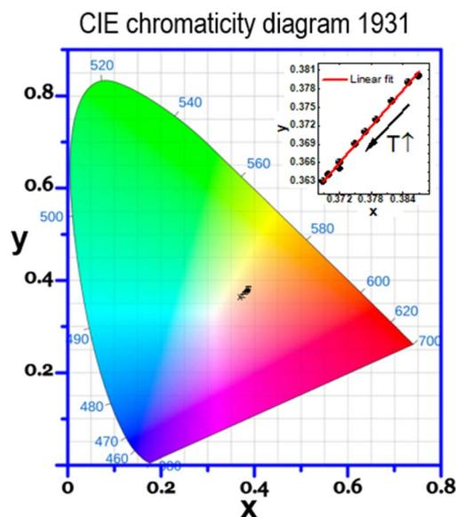
Fig. 11 CIE color coordinates for CLSPO:3 at%  $\text{Dy}^{3+}$  phosphors in the temperature range 298 to 523 K; the figure at top right shows the evolution of color coordinates as a function of temperature.
