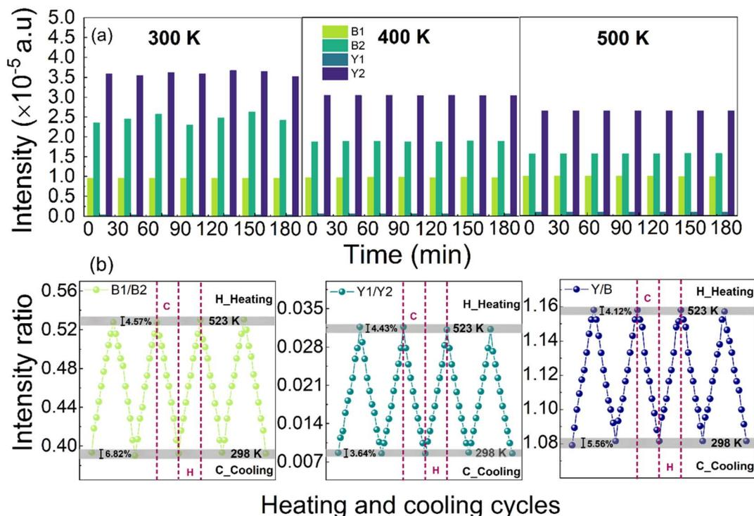
Fig. 13 (a) The photoluminescence intensity stability at temperatures of 300, 400, and 500 K for 180 minutes and (b) the repeatability test of the luminescence intensity ratio of during heating and cooling cycles of CLSPO:3 at% Dy<sup>3+</sup> phosphors.
