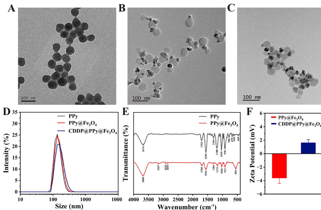
Fig. 2 (A–C) Transmission electron microscopy images showing (A) PPy, (B) PPy@Fe<sub>3</sub>O<sub>4</sub>, and (C) CDDP@PPy@Fe<sub>3</sub>O<sub>4</sub>. (D) Particle-size distribution of PPy, PPy@Fe<sub>3</sub>O<sub>4</sub>, and CDDP@PPy@Fe<sub>3</sub>O<sub>4</sub>. (E) Fourier transform infrared spectroscopy of PPy and PPy@Fe<sub>3</sub>O<sub>4</sub>. (F) Zeta potential of PPy@Fe<sub>3</sub>O<sub>4</sub> and CDDP@PPy@Fe<sub>3</sub>O<sub>4</sub>.
