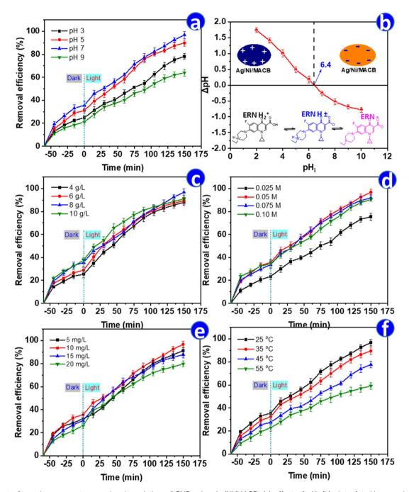
Fig. 6 Effect of reaction parameters on the degradation of ENR using Ag/Ni/MACB: (a) effect of pH, (b) plot of  $\Delta$ pH versus initial pH for determining pH<sub>pzc</sub>, along with the surface charge of Ag/Ni/MACB and ERN as a function of pH, (c) effect of catalyst dosage, (d) effect of H<sub>2</sub>O<sub>2</sub> concentration, (e) effect of initial enrofloxacin concentration, and (f) effect of temperature.
