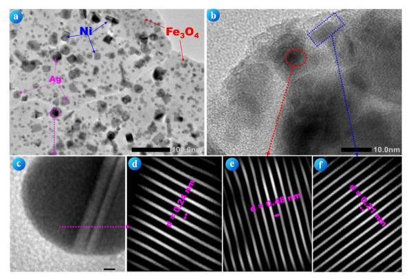
Fig. 3 (a) TEM image showing the surface morphology of the Ag/Ni/MACB composite; (b and c) magnified TEM images of selected nanoparticles; (d-f) the lattice spacings (d-spacing) of Ag, Fe<sub>3</sub>O<sub>4</sub>, and Ni nanoparticles, respectively, obtained using ImageJ analysis.
