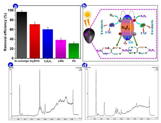
Fig. 7 (a) Degradation performance of ENR in the presence of different scavengers; (b) proposed degradation mechanism; (c and d) total ion chromatograms (TIC) of the ENR solution after photo-Fenton catalytic degradation by Ag/Ni/ACB at 60 min (c) and 150 min (d).
