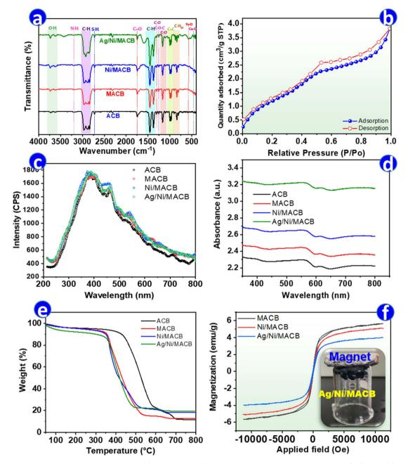
Fig. 4 Characterization of the synthesized samples: (a) FTIR spectra, (b)  $N_2$  adsorption—desorption isotherm of Ag/Ni/MACB, (c) PL spectra, (d) UV-Vis DRS curves, (e) TGA profile, and (f) magnetization curves.
