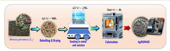
Scheme 1 Schematic illustration of the synthesis process of Ag/Ni/MACB via a one-pot green synthesis.
