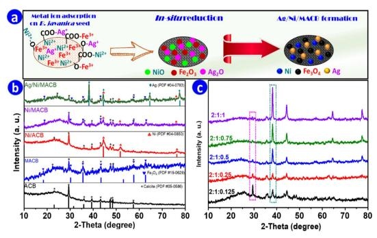
Fig. 1 (a) Proposed formation mechanism of the Ag/Ni/MACB catalyst, (b) XRD patterns of different samples, including ACB, MACB, Ni/ACB, Ni/MACB, and Ag/Ni/MACB, (c) XRD patterns of Ag/Ni/MACB with varying Ag contents.
