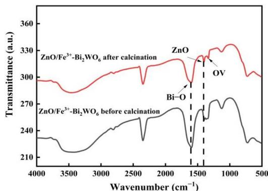
Fig. 7 Infrared spectra of ZnO/Fe<sup>3+</sup>-doped Bi<sub>2</sub>WO<sub>6</sub> before and after calcination.
