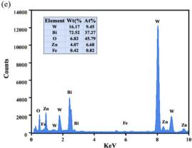
Fig. 3 TEM images of the ZnO/Fe<sup>3+</sup>-doped Bi<sub>2</sub>WO<sub>6</sub> nanocomposites (a-d) and TEM-EDS diagram (e).
