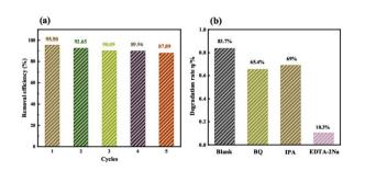
Fig. 12 The cycle experimental diagram (a) and active species capture experimental diagram (b) of  $ZnO/Fe^{3+}$ - $Bi_2WO_6$  catalyst.
