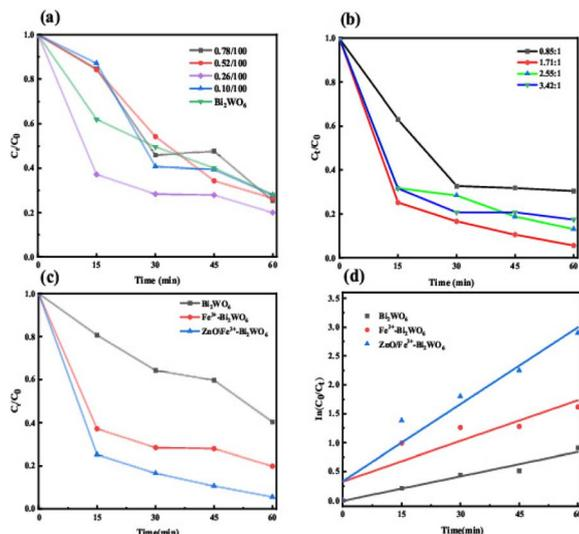
Fig. 11 Degradation curves (a–c) and kinetic curves (d) of different materials under simulated sunlight irradiation.
