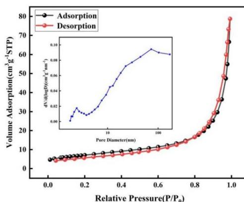
Fig. 6 Nitrogen adsorption–desorption isotherm, and pore size distribution of ZnO/Fe<sup>3+</sup>-doped Bi<sub>2</sub>WO<sub>6</sub>.
