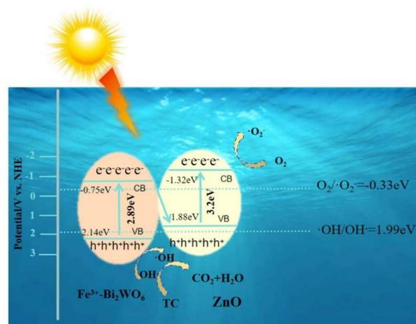
Fig. 13 Degradation mechanism of ZnO/ $\text{Fe}^{3+}$ -doped  $\text{Bi}_2\text{WO}_6$ .
