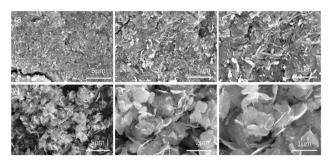
Fig. 2 SEM images of Bi<sub>2</sub>WO<sub>6</sub> (a-c) and ZnO/Fe<sup>3+</sup>-doped Bi<sub>2</sub>WO<sub>6</sub> (df).
