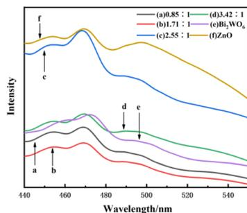
Fig. 9 Fluorescence spectra of ZnO/Fe<sup>3+</sup>-doped Bi<sub>2</sub>WO<sub>6</sub>, pure Bi<sub>2</sub>WO<sub>6</sub> and ZnO with different molar ratios.
