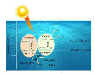
Fig. 13 Degradation mechanism of ZnO/Fe<sup>3+</sup>-doped Bi<sub>2</sub>WO<sub>6</sub>
