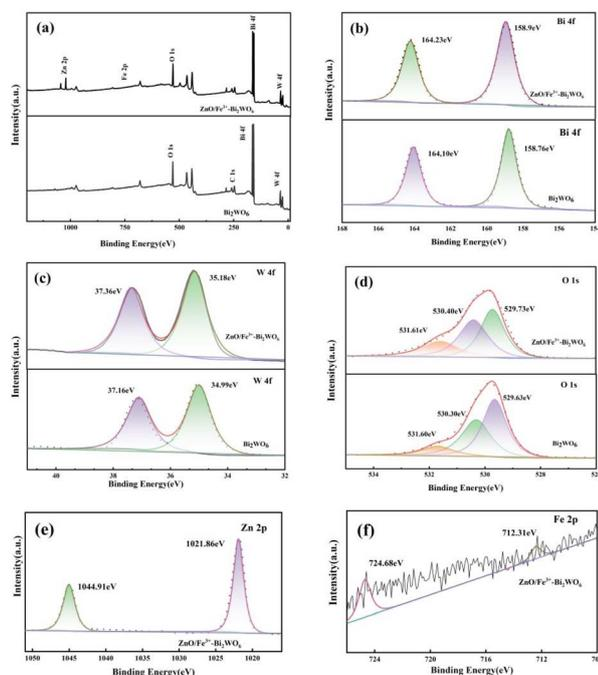
Fig. 5 XPS spectra of ZnO/Fe<sup>3+</sup>-doped Bi<sub>2</sub>WO<sub>6</sub> and Bi<sub>2</sub>WO<sub>6</sub> sample: (a) survey of the photocatalyst; (b) Bi 4f; (c) W 4f; (d) O 1s; (e) Zn 2p; (f) Fe 2p.
