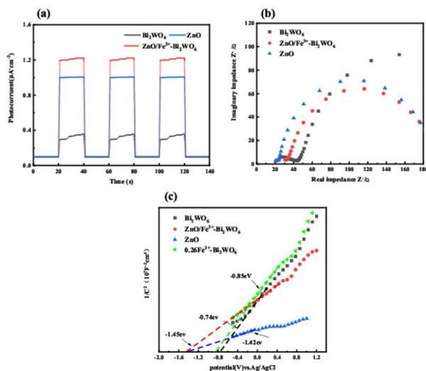
Fig. 10 Impedance spectra (a), photocurrent response curves (b) and MS curves (c) of ZnO/Fe<sup>3+</sup>-doped Bi<sub>2</sub>WO<sub>6</sub>, Bi<sub>2</sub>WO<sub>6</sub>, ZnO and 0.26Fe<sup>3+</sup>-doped Bi<sub>2</sub>WO<sub>6</sub>.
