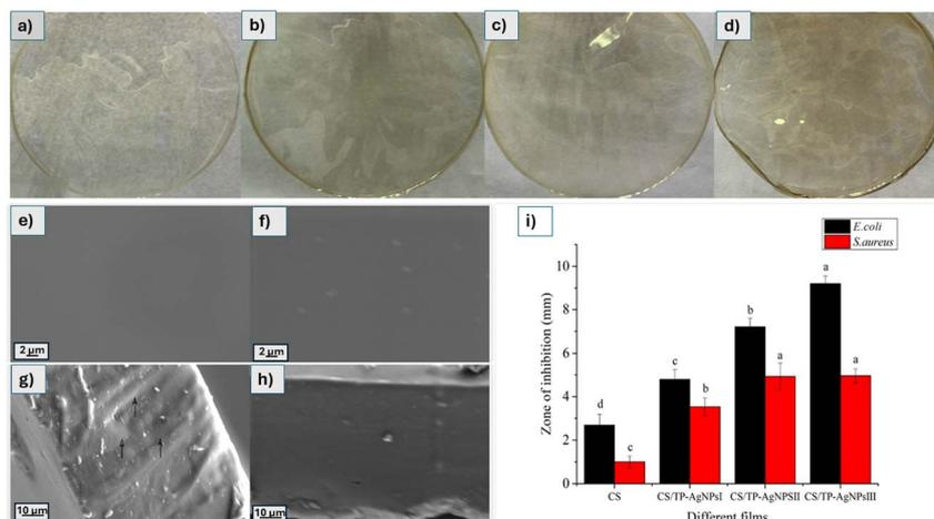
Fig. 10 (a) CS film, (b) CS/TP–AgNPsI film, (c) CS/TP–AgNPsII film, (d) CS/TP–AgNPsIII film. SEM images of the surface and cross-section for (e and g) CS film and (f and h) CS/TP–AgNPsIII film. (i) The inhibition zone (A) of chitosan films, both with and without varying concentrations of TP–AgNPs, against the growth of *E. coli* and *S. aureus*. Error bars represent the standard deviation, reproduced with permission from ref. 127 copyright © 2019 Elsevier B.V. All rights reserved.
