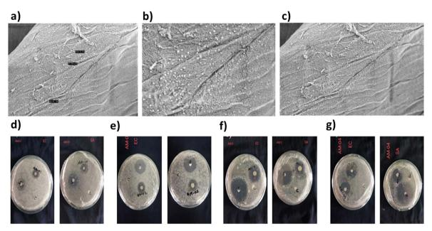
Fig. 13 SEM images of AgNPs: (a) nanoparticle (NP) size, (b) green synthesis, (c) chemical synthesis, inhibition zone of AgNPs, (d) recycled AgNPs in green synthesis, (e) pure AgNPs in green synthesis, (f) recycled AgNPs in chemical synthesis, and (g) pure AgNPs in chemical synthesis on fabric samples against *S. aureus* and *E. coli*. Reproduced from ref. 159 copyright © 2023, The Author(s) under a Creative Commons Attribution 4.0.
