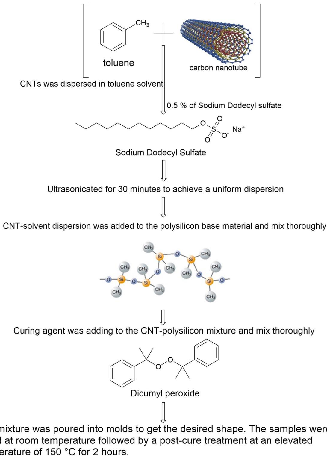
Fig. 1 Steps for the preparation of samples.
