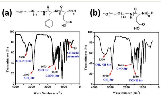
Fig. 2 FTIR spectra of (a) mPEG-b-PBLG and (b) mPEG-b-PLG.
