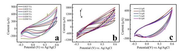
Fig. 6 Cyclic voltammetry peaks of glycine at (a) different scan rates (b) different concentrations and (c) at different pH values (experimental conditions: 5 mM glycine, 0.1 mM PBS pH = 8, potential window -0.3 to 0.6 V).
