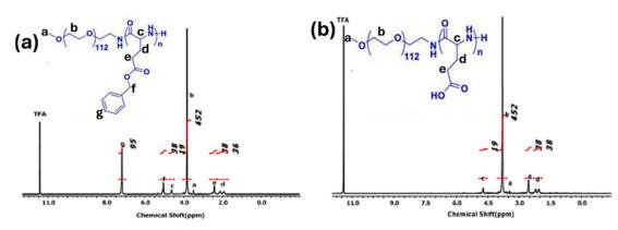
Fig. 3 <sup>1</sup>H NMR spectra of (a) mPEG-b-PBLG and (b) mPEG-b-PLG
