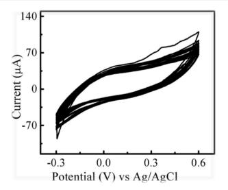
Fig. 8 Stability of CdOQDs/polymer-ePAS after 25 cycles. Experimental conditions: (concentration of glycine 5 mM, scan rate 0.01 V  $s^{-2}$ , 0.1 mM PBS, potential window -0.3 to +0.6 V).
