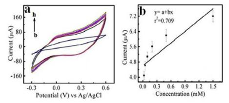
Fig. 7 Voltammetry peaks at different concentrations (a) concentration  $\{0.05-1.5 \text{ mM}\}$  (b) straight line graph between concentration and current, which shows the dependence of peak current on the concentration of samples. Conditions: PBS pH 7.0; scan rate  $0.01 \text{ V s}^{-2}$ ; potential window -0.4 to +0.6 V.
