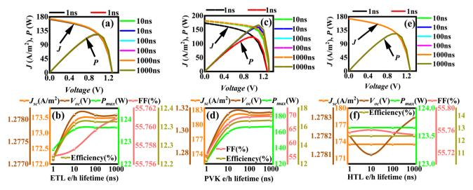
Fig. 5 (a) J-V and P-V characteristics at different e-h lifetime (ns) in ETL, and its effect on (b)  $J_{sc}$ ,  $V_{oc}$ ,  $P_{max}$ , FF, and efficiency, (c) J-V and P-V curves at different e-h lifetime (ns) in PVK, and its effect on (d)  $J_{sc}$ ,  $V_{oc}$ ,  $P_{max}$ , FF, and efficiency, (e) J-V and P-V response at different e-h lifetime (ns) in HTL, and its effect on (f)  $J_{sc}$ ,  $V_{oc}$ ,  $P_{max}$ , FF, and efficiency.
