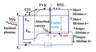
Fig. 4 Schematic illustration exhibiting the role of e-h lifetime of ETL, PVK, and HTL on solar cell perform.
