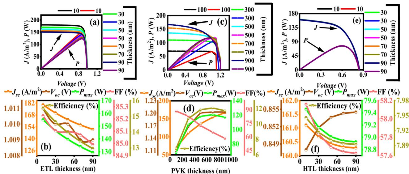
Fig. 2 (a)  $J$ - $V$  and  $P$ - $V$  characteristics at different ETL thicknesses (nm), and its effect on (b)  $J_{sc}$ ,  $V_{oc}$ ,  $P_{max}$ , FF, and efficiency, (c)  $J$ - $V$  and  $P$ - $V$  curves at different PVK thicknesses (nm), and its effect on (d)  $J_{sc}$ ,  $V_{oc}$ ,  $P_{max}$ , FF, and efficiency, (e)  $J$ - $V$  and  $P$ - $V$  response at different HTL thicknesses (nm), and its effect on (f)  $J_{sc}$ ,  $V_{oc}$ ,  $P_{max}$ , FF, and efficiency.
