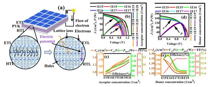
Fig. 3 (a) Schematic illustration exhibiting the role of donor/acceptor concentrations of ETL and HTL on solar cell performance, (b) J-V and P-V characteristics at different acceptor concentrations, and its effect on (c)  $J_{\text{sc}}$ ,  $V_{\text{oc}}$ ,  $P_{\text{max}}$ , FF, and efficiency, (d) J-V and P-V curves at different donor concentrations, and its effect on (e)  $J_{\text{sc}}$ ,  $V_{\text{oc}}$ ,  $P_{\text{max}}$ , FF, and efficiency.
