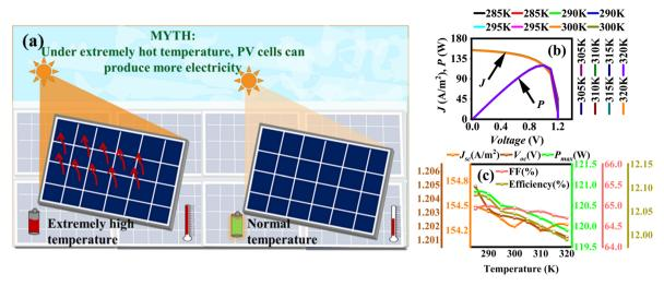
Fig. 6 (a) Visual representation of impact of lower and higher temperature (K) on solar cell performance, (b) J-V and P-V characteristics at different device's operating temperature (K), and its effect on (c)  $J_{sc}$ ,  $V_{oc}$ ,  $P_{max}$ , FF, and efficiency.
