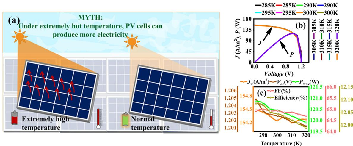
Fig. 6 (a) Visual representation of impact of lower and higher temperature (K) on solar cell performance, (b)  $J$ - $V$  and  $P$ - $V$  characteristics at different device's operating temperature (K), and its effect on (c)  $J_{sc}$ ,  $V_{oc}$ ,  $P_{max}$ , FF, and efficiency.
