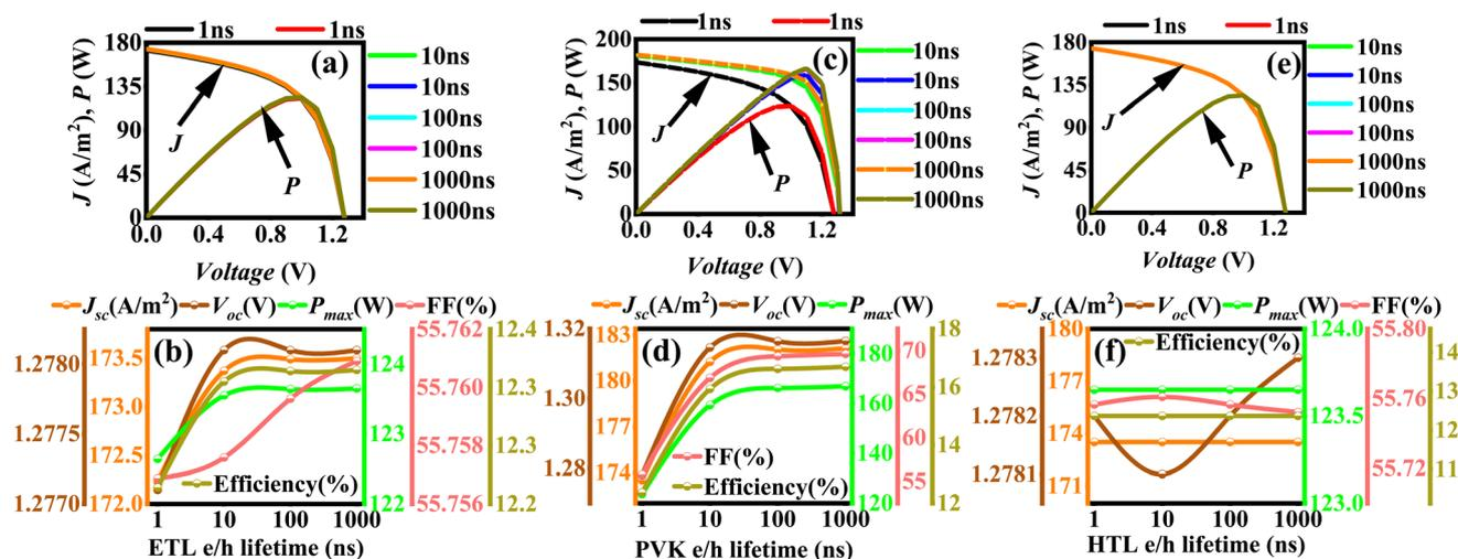
Fig. 5 (a)  $J$ - $V$  and  $P$ - $V$  characteristics at different e-h lifetime (ns) in ETL, and its effect on (b)  $J_{sc}$ ,  $V_{oc}$ ,  $P_{max}$ , FF, and efficiency, (c)  $J$ - $V$  and  $P$ - $V$  curves at different e-h lifetime (ns) in PVK, and its effect on (d)  $J_{sc}$ ,  $V_{oc}$ ,  $P_{max}$ , FF, and efficiency, (e)  $J$ - $V$  and  $P$ - $V$  response at different e-h lifetime (ns) in HTL, and its effect on (f)  $J_{sc}$ ,  $V_{oc}$ ,  $P_{max}$ , FF, and efficiency.
