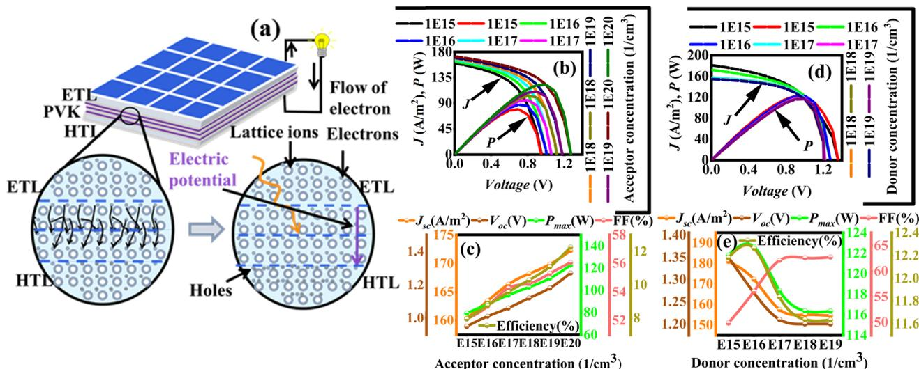
Fig. 3 (a) Schematic illustration exhibiting the role of donor/acceptor concentrations of ETL and HTL on solar cell performance, (b)  $J$ - $V$  and  $P$ - $V$  characteristics at different acceptor concentrations, and its effect on (c)  $J_{sc}$ ,  $V_{oc}$ ,  $P_{max}$ , FF, and efficiency, (d)  $J$ - $V$  and  $P$ - $V$  curves at different donor concentrations, and its effect on (e)  $J_{sc}$ ,  $V_{oc}$ ,  $P_{max}$ , FF, and efficiency.
