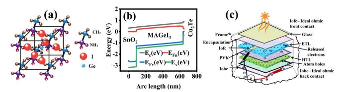
Fig. 1 (a) Crystal structure of CH<sub>3</sub>NH<sub>3</sub>Gel<sub>3</sub> perovskite material, (b) energy band alignment of ETL, PVK layer, and HTL to ensure the smooth pathway for removal of electron and hole from absorbing layer towards respective electrodes, and (c) schematic illustration of working of solar cell highlighting the role of thicknesses of ETL, PVK, and HTL.
