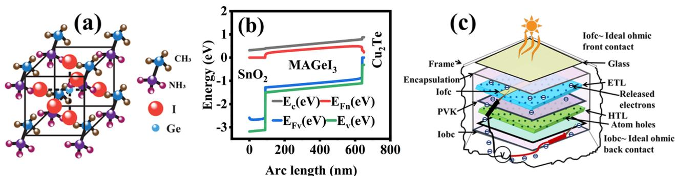
Fig. 1 (a) Crystal structure of  $\text{CH}_3\text{NH}_3\text{GeI}_3$  perovskite material, (b) energy band alignment of ETL, PVK layer, and HTL to ensure the smooth pathway for removal of electron and hole from absorbing layer towards respective electrodes, and (c) schematic illustration of working of solar cell highlighting the role of thicknesses of ETL, PVK, and HTL.
