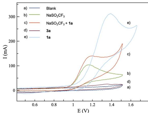
Fig. 2 Cyclic voltammograms of substrate **1a** in 0.1 M  $\text{LiClO}_4/\text{ACN}$ , using a Glassy Carbon (GC) as working electrode, Pt as counter electrode and  $\text{Fc}/\text{Fc}^+$  (0.1 M in ACN) as internal standard.
