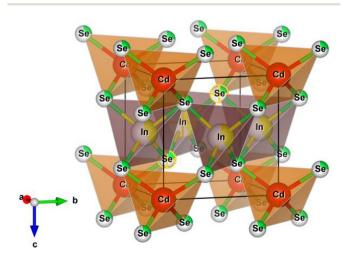
Fig. 3 Polyhedron representation of the tetragonal structure of the ternary semiconducting compound CdIn<sub>2</sub>Se<sub>4</sub>.
