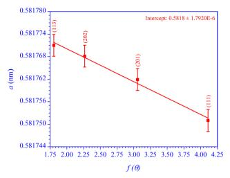
Fig. 5 N-R diagram of the ternary semiconducting compound CdIn<sub>2</sub>Se<sub>4</sub>
