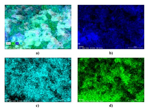
Fig. 10 Elemental mapping of the ternary semiconducting compound Cdln<sub>2</sub>Se<sub>4</sub>.
