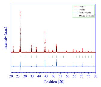
Fig. 2 Rietveld profile fitting of the ternary semiconducting compound CdIn<sub>2</sub>Se<sub>4</sub>.
