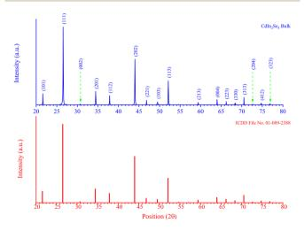
Fig. 1  $\,$  X-ray diffractogram of the ternary semiconducting compound  $\,$  CdIn $_2$ Se $_4$ .
