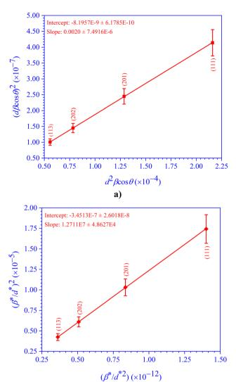
Fig. 8 (a) SSP and (b) H-W plots for the ternary semiconducting compound  $Cdln_2Se_4$ .
