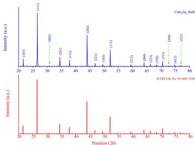
Fig. 1 X-ray diffractogram of the ternary semiconducting compound CdIn<sub>2</sub>Se<sub>4</sub>.
