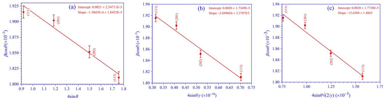
Fig. 7 W–H plots: (a) UDM, (b) USDM, and (c) UDEDM for the ternary semiconducting compound CdIn<sub>2</sub>Se<sub>4</sub>.
