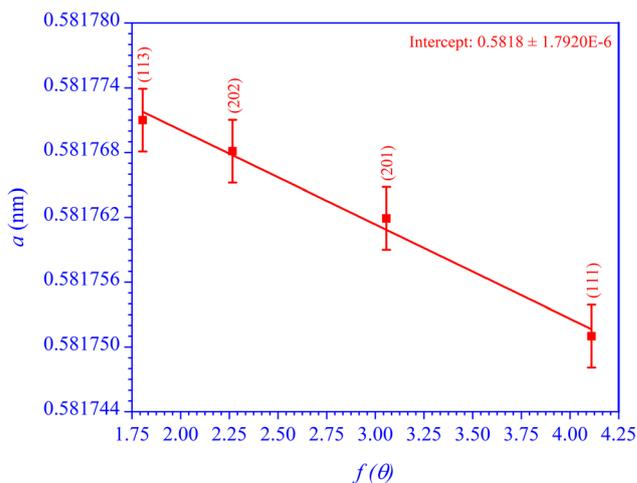
**Fig. 5** N–R diagram of the ternary semiconducting compound CdIn<sub>2</sub>Se<sub>4</sub>.
