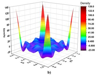
Fig. 4 (a) 2D, and (b) 3D electron density maps of individual atoms on the x-y (z=0) plane in the unit cell of the ternary semiconducting compound  $Cdln_2Se_4$ .
