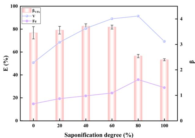
Fig. 3 Effect of saponification degree on extraction.
