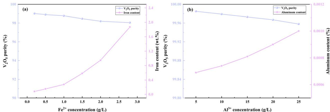
Fig. 2 Effect of (a) Fe<sup>2+</sup> and (b) Al<sup>3+</sup> concentration on V<sub>2</sub>O<sub>5</sub> purity (vanadium precipitation conditions: initial pH 1.8, temperature 95 °C, time 1.5 h).
