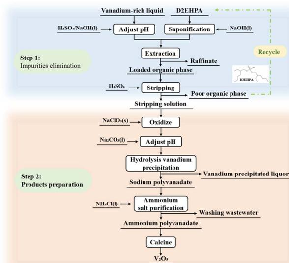
Fig. 1 A flowchart of the  $V_2O_5$  preparation process.
