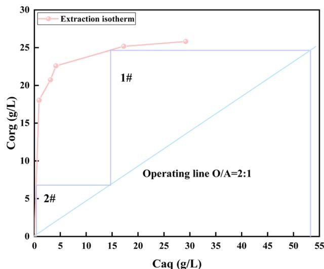
Fig. 5 McCabe–Thiele diagram for determining the number of vanadium extraction stages (conditions: initial pH of 1.8, D2EHPA concentration of 40 vol%, time of 8 minutes).
