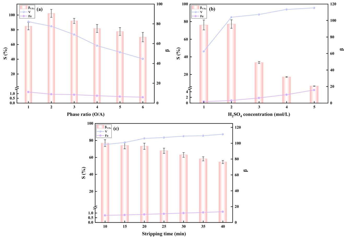
Fig. 6 Effect of phase ratio (a), H<sub>2</sub>SO<sub>4</sub> concentration (b), and time (c) on vanadium and Fe<sup>2+</sup> stripping rates and  $\beta_{V/Fe}$ .
