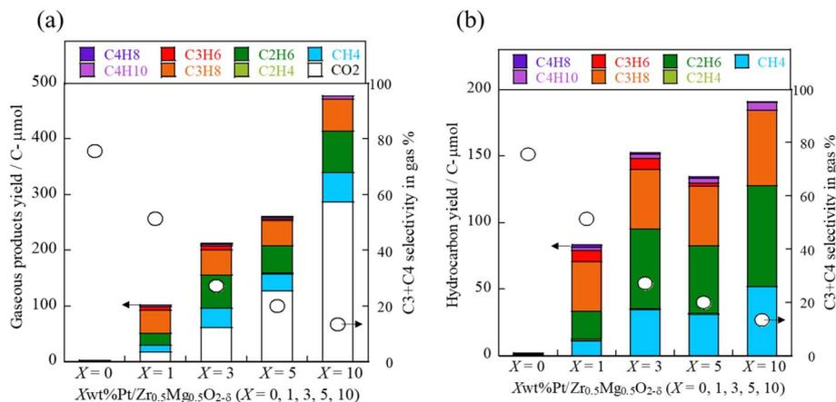
Fig. 6 (a) Gaseous product yields and (b) hydrocarbon yield using  $X$  wt% Pt/Zr<sub>0.5</sub>Mg<sub>0.5</sub>O<sub>2-δ</sub> ( $X = 0, 1, 3, 5, 10$ ), cellulose, 443 K, 12 h. Liquid products are shown in Fig. S10 in ESI.†
