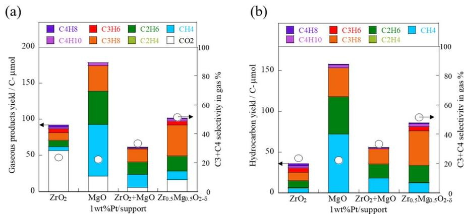
Fig. 4 (a) Gaseous product yield and (b) hydrocarbon yield obtained using 1 wt% Pt/support (ZrO<sub>2</sub>, MgO, mixed, doped), cellulose, 443 K, 12 h. Liquid products are shown in Fig. S8 in ESI†
