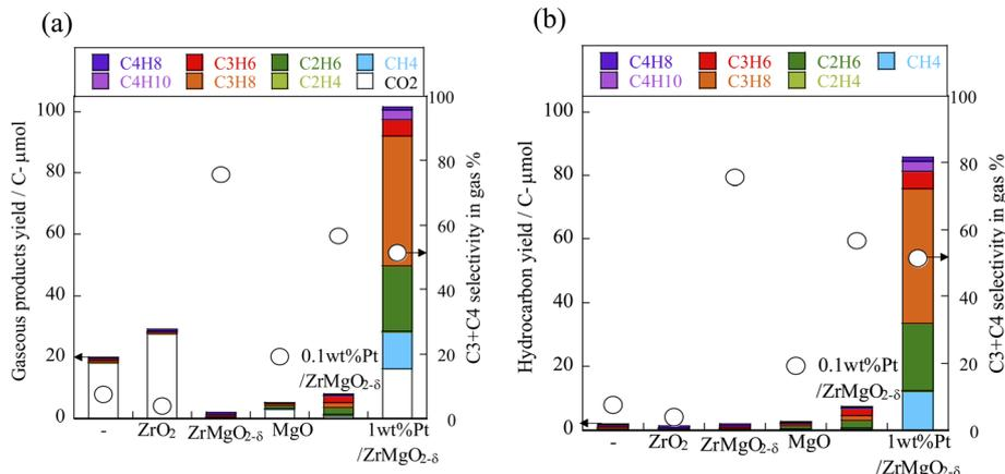
Fig. 7 (a) Gaseous product yield and (b) hydrocarbon yield using  $X$  wt% Pt/Zr<sub>1-x</sub>Mg<sub>x</sub>O<sub>2-δ</sub> ( $X = 0, 0.1, 1$ ) ( $x = 0, 0.5, 1$ ), cellulose, 443 K, 12 h. Liquid products are shown in Fig. S18 in ESI.†
