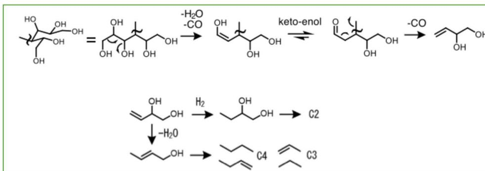
Fig. 11 Estimated reaction mechanisms from cellulose over Pt/Zr<sub>0.5</sub>Mg<sub>0.5</sub>O<sub>2- $\delta$</sub>  catalyst.
