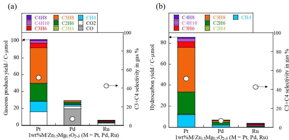
Fig. 5 (a) Gaseous product yield and (b) hydrocarbon yield using 1 wt% M/Zr<sub>0.5</sub>Mg<sub>0.5</sub>O<sub>2-δ</sub> (M = Pt, Pd, Ru), cellulose, 443 K, 12 h. Liquid products are shown in Fig. S9 in ESI†
