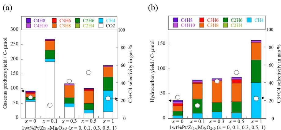
Fig. 3 (a) Gaseous product yield and (b) hydrocarbon yield obtained using 1 wt% Pt/Zr<sub>1-x</sub>Mg<sub>x</sub>O<sub>2-δ</sub> (x = 0, 0.1, 0.3, 0.5, 1), cellulose, 443 K, 12 h. Liquid products are shown in Fig. S7 in ESI.†
