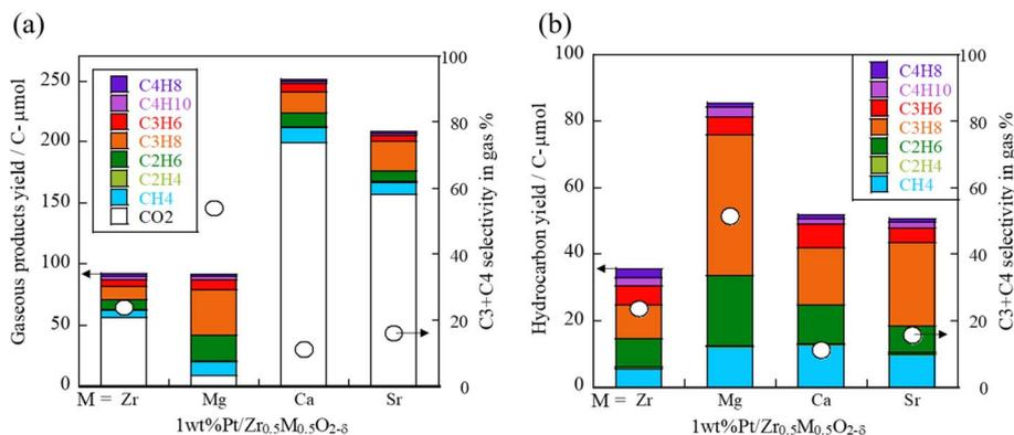
Fig. 2 (a) Gaseous product yield and (b) hydrocarbon yield obtained using 1 wt% Pt/Zr<sub>0.5</sub>Mg<sub>0.5</sub>O<sub>2-δ</sub> (M = Zr, Mg, Ca, Sr), cellulose, 443 K, 12 h. Liquid products are shown in Fig. S4 in ESI.†
