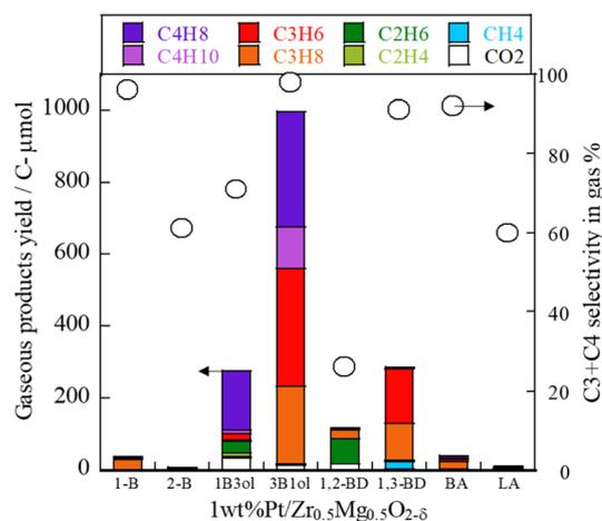
Fig. 8 Conversion of C<sub>3</sub> and C<sub>4</sub> hydrocarbon-like liquid compounds using 1 wt% Pt/Zr<sub>0.5</sub>Mg<sub>0.5</sub>O<sub>2-δ</sub> catalyst (1-B: 1-butanol, 2-B: 2-butanol, 1B3ol: 1-butene-3-ol, 3B1ol: 3-butene-1-ol, 1,2-BD: 1,2-butanediol, 1,3-BD: 1,3-butanediol, BA: butyric acid, LA: levulinic acid).
