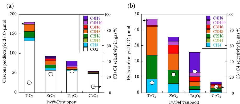
Fig. 1 (a) Gaseous product yield and (b) hydrocarbon yield obtained using 1 wt% Pt/support (TiO<sub>2</sub>, ZrO<sub>2</sub>, Ta<sub>2</sub>O<sub>5</sub>, CeO<sub>2</sub>), cellulose, 443 K, 12 h.
