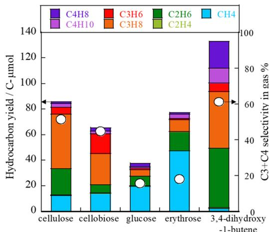
Fig. 10 Conversion of candidate intermediates using 1 wt% Pt/Zr<sub>0.5</sub>Mg<sub>0.5</sub>O<sub>2-δ</sub>, 443 K, 12 h.
