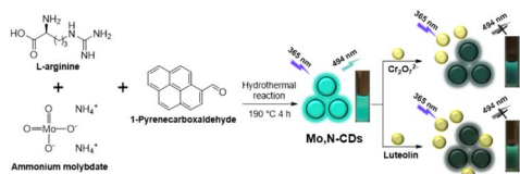
Scheme 1 Synthesis of Mo, N-CDs for \text{Cr}_2\text{O}_7^{2-} and luteolin detection.
