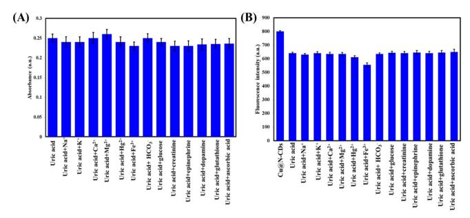
Fig. 4 Anti-interference studies were conducted on the Cu@N-CDs/AP-NH<sub>2</sub>/ph-OH/uricase system for the determination of uric acid using the colorimetric method ((A) with a uric acid concentration of 30  $\mu$ M) and the fluorometric method ((B) with a uric acid concentration of 120  $\mu$ M). The concentrations of interfering ions and biomolecules were set at 500  $\mu$ M and 20  $\mu$ M, respectively.
