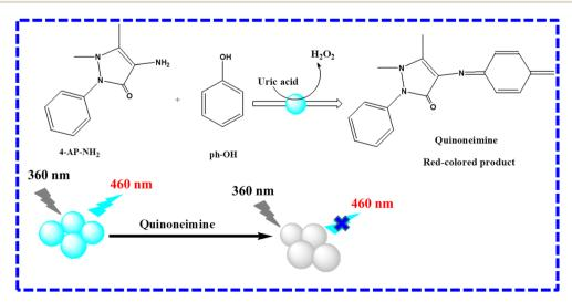
Scheme 1 Dual-mode detection of uric acid via Cu@N-CDs, AP-NH<sub>2</sub>, uricase, and ph-OH.
