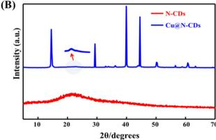
Fig. 1 EXD (A) and PXRD (B) patterns of Cu@N-CDs.
